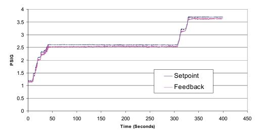
Figure 5-20: Pressure-Controlled Excavator 12-ft Tank Test: Descending Readings
