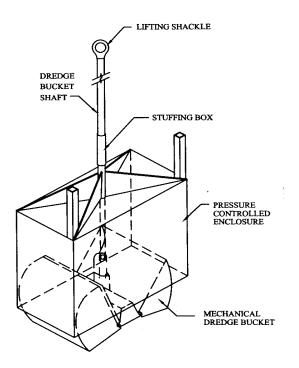
Figure 4-1: Enclosure and Bucket
