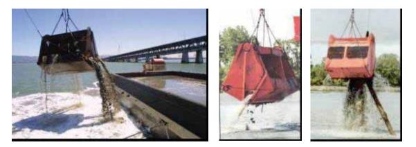
Figure 2-3. Leaky Clamshell Buckets
