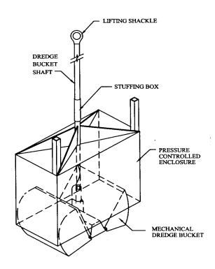
Figure S-1: Pressure-Controlled Enclosure and Bucket
