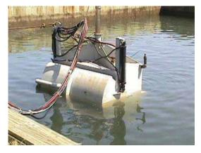
Figure 5-25: Field Prototype Unit Descending for Excavation
