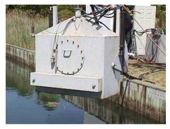
Figure S-2: Pressure-Controlled Excavator Ready for Submersion
