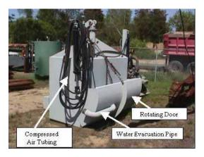
Figure 5-16: Pressure Controlled Excavator: Compressed Air Hosing and Rotating Door
