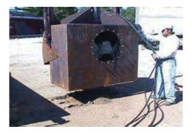
Figure 5-10: Enclosed Excavator Maintenance Hatch
