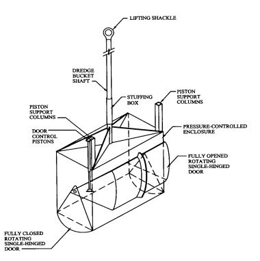
Figure 4-2: Enclosure with Single Hinged Door
