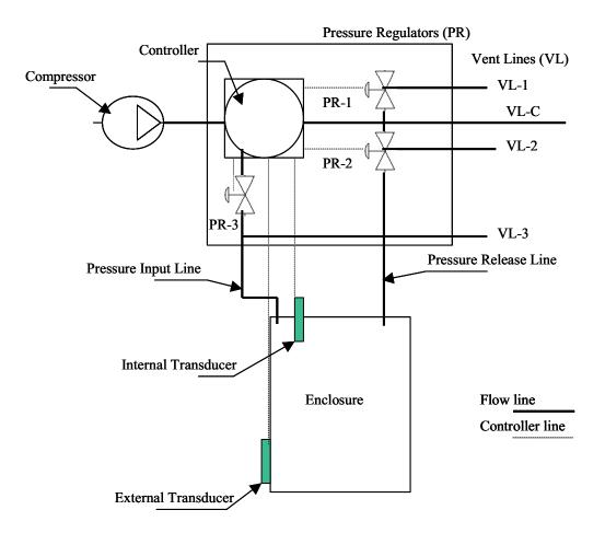
Figure 4-4: Pressure Controller Feedback Control System
