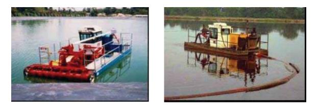
Figure 2-2. Hydraulic Cutterheads and Horizontal Augers
