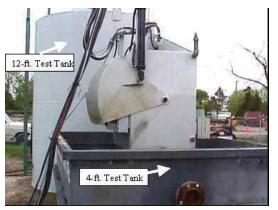
Figure 5-18: Pressure-Controlled Excavator: 4-Foot Tank Test
