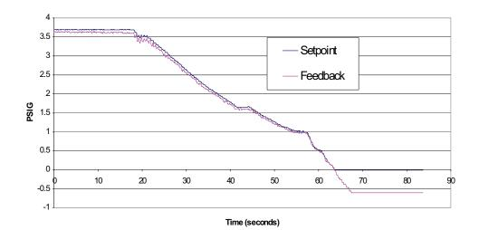
Figure 5-21: Pressure-Controlled Excavator 12-ft Tank Test: Ascending Readings
