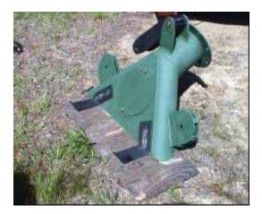
Figure 4-4. Cutter-less Vacuum Head
