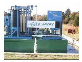
Figure 4-1. Mobile Water Filtration Plant (Membrane Treatment provided by the Pall Corporation)
