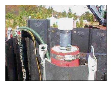
Figure 6-3. Sealing Tube Cap and Air-Fill Port
