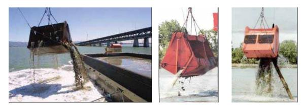
Figure 2-3. Leaky Clamshell Buckets
