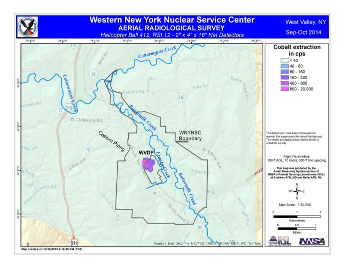
Figure 22: Interpolated map of count rates from cobalt-60 isotopic extraction (detail over WNYNSC). Cobalt-60 signatures were not observed anywhere else in the survey area.
