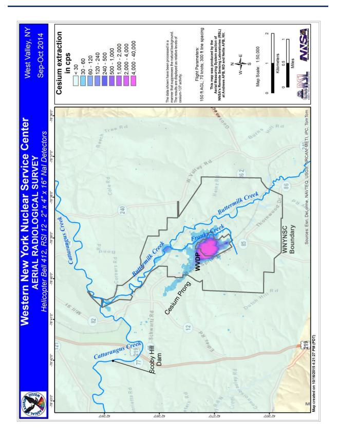
Figure 20: Interpolated map of count rates from cesium-137 isotopic extraction (detail over WNYNSC).
