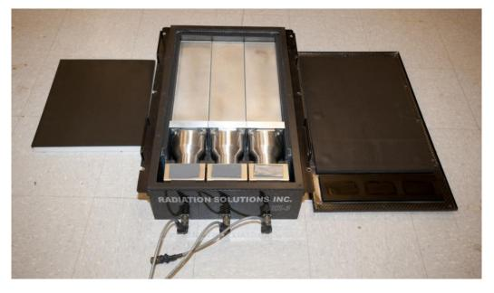
Figure 2: RSX-3 detector unit with three 2" × 4" × 16" Nal(TI) scintillators, three photomultiplier tubes, and three ADS modules.
