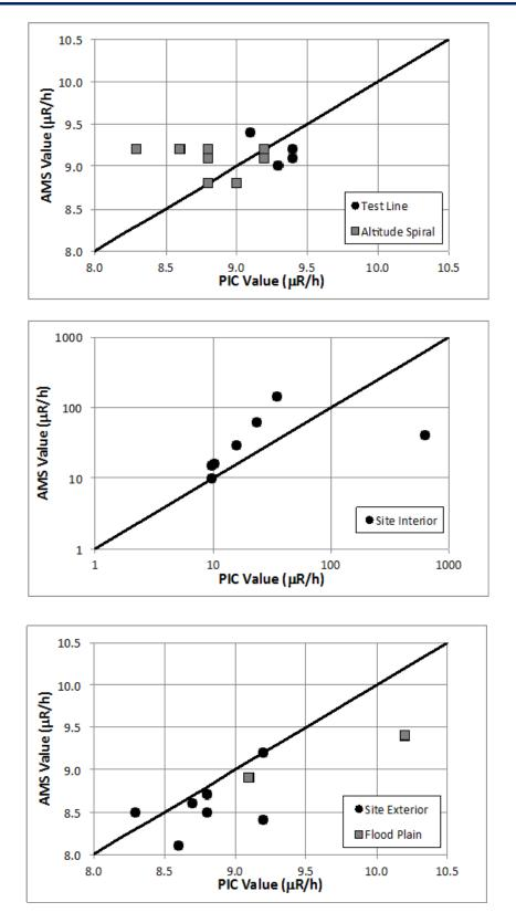
Figure 13: Comparison of exposure rates from AMS and PIC measurements. The top panel shows results for test line and altitude spiral, the middle panel shows results for site interior measurements, and the bottom panel shows results for the site exterior and flood plain. The straight lines indicate a perfect correlation, added as a guide for the eye. Note the logarithmic axes in the middle plot.
