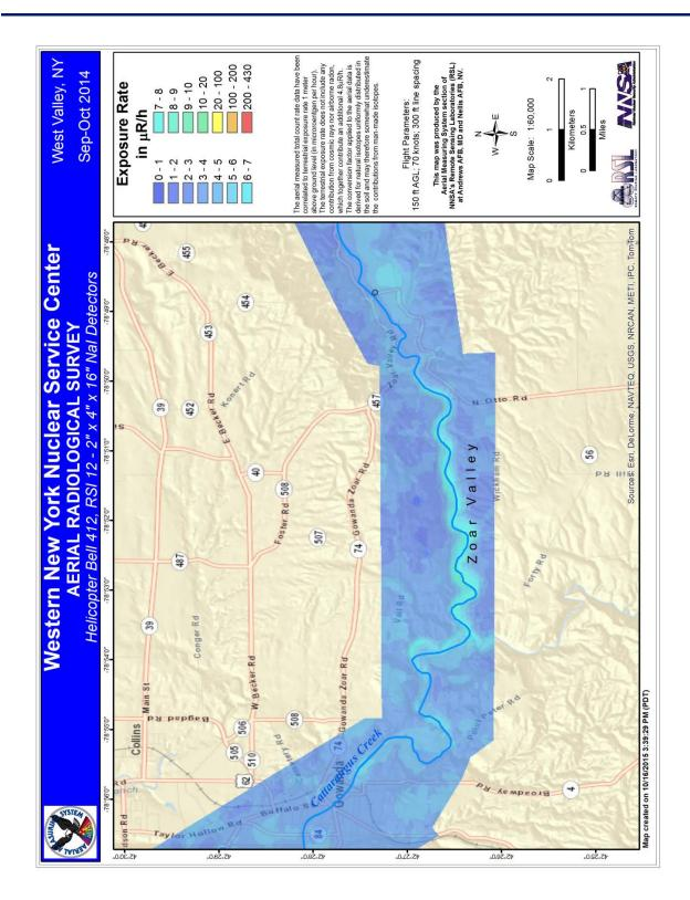
Figure 12: Exposure rate measurement (circle at east end of map, intersection of N Otto Road and Zoar Valley Road) taken with the pressurized ionization chamber along Cattaraugus Creek near Zoar Valley, overlaid on the inferred terrestrial exposure rate map from aerial survey data. PIC exposure rates have been corrected to eliminate contributions from radon and cosmic rays to facilitate direct comparison to the aerial data.
