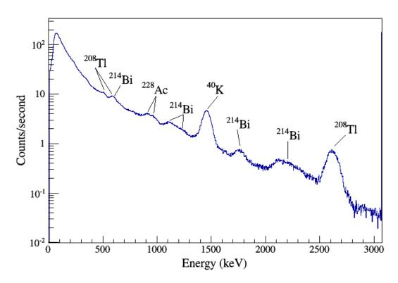
Figure 7: Typical spectrum of natural radioactive background, as measured by the AMS detectors at nominal survey altitude. Annotated peaks are commonly observed signatures of various decay products from radioactive potassium, uranium and thorium.
