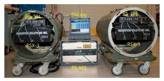
Figure 3: Components of the RSI data acquisition system.
