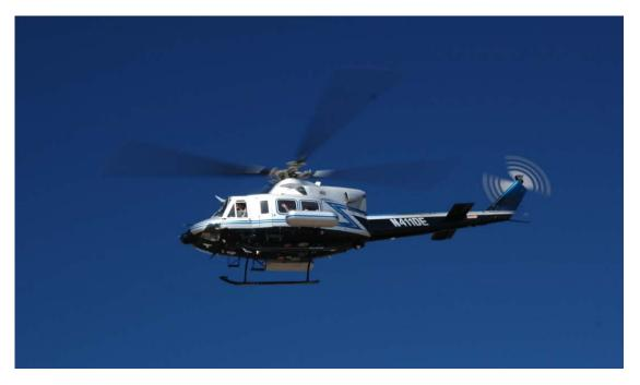
Figure 4: AMS Bell 412 helicopter with externally mounted detector pods.
