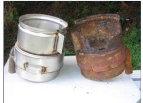
Corrosion due to combustion involving chlorine
