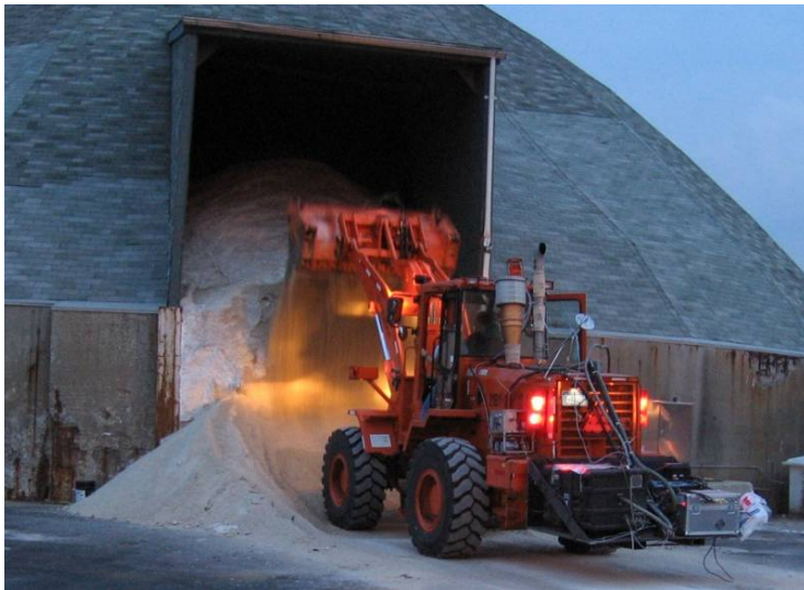
In-Use Testing of a Daewoo Loader
