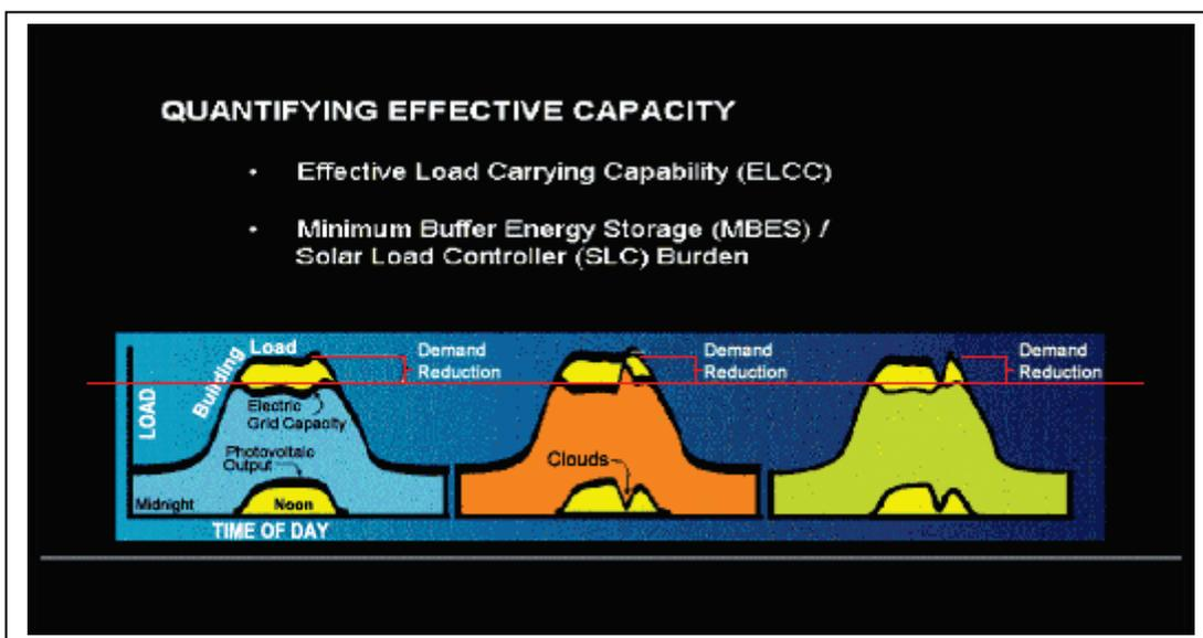
excess demand can be met by adding energy from the solar generation of electricity. When solar conditions are not good, backup energy supplies would be needed at that time (see middle graph), or alternatively, a reduction in consumer consumption would be necessary to guarantee that all resources above the red line are provided (see right graph).
