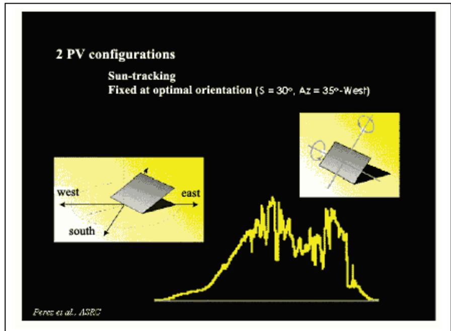
The graph at the bottom of the diagram shows typical solar energy collection by an ideal Sun-tracking PV array from sunrise to sunset on a July day.
