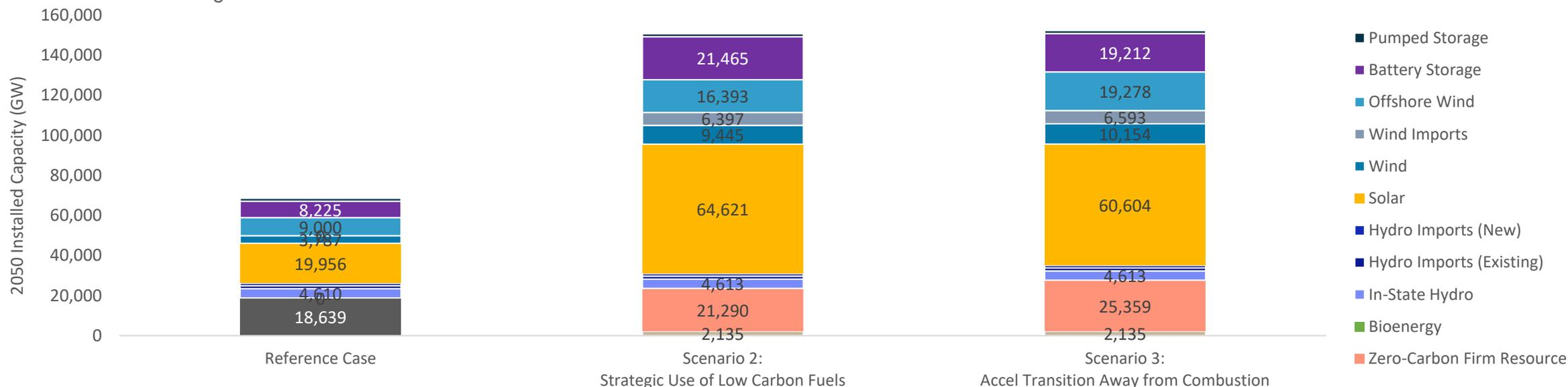
Note: In Scenario 3, existing fossil fuel resources are retired by 2040 and no new combustion-based (CCGT or CT) capacity is permitted. New firm capacity is provided by a combustion-free resource (e.g. hydrogen fuel cells).
