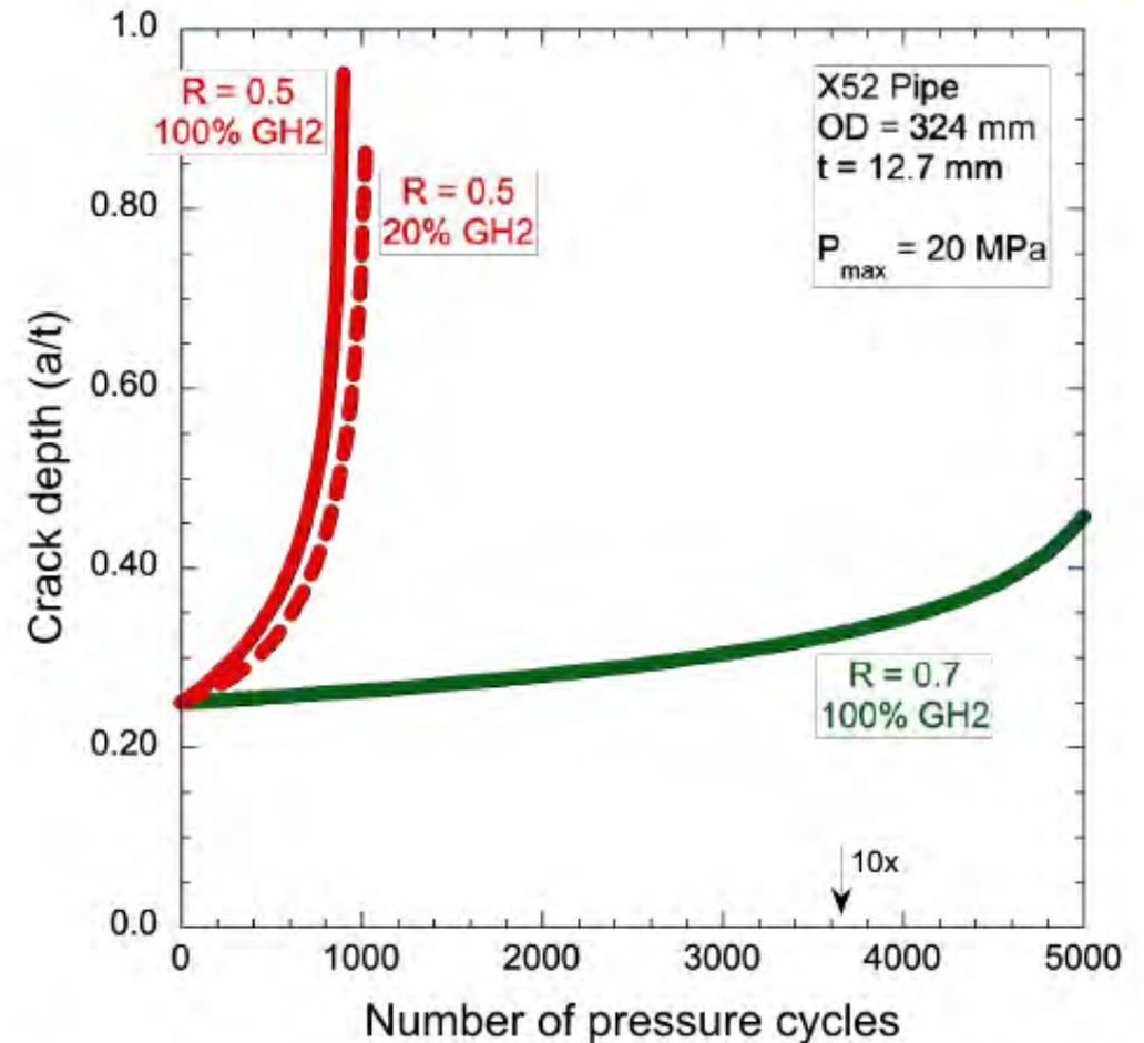
The blending ratio has no effect on fatigue response (for  $R = 0.5$ )
