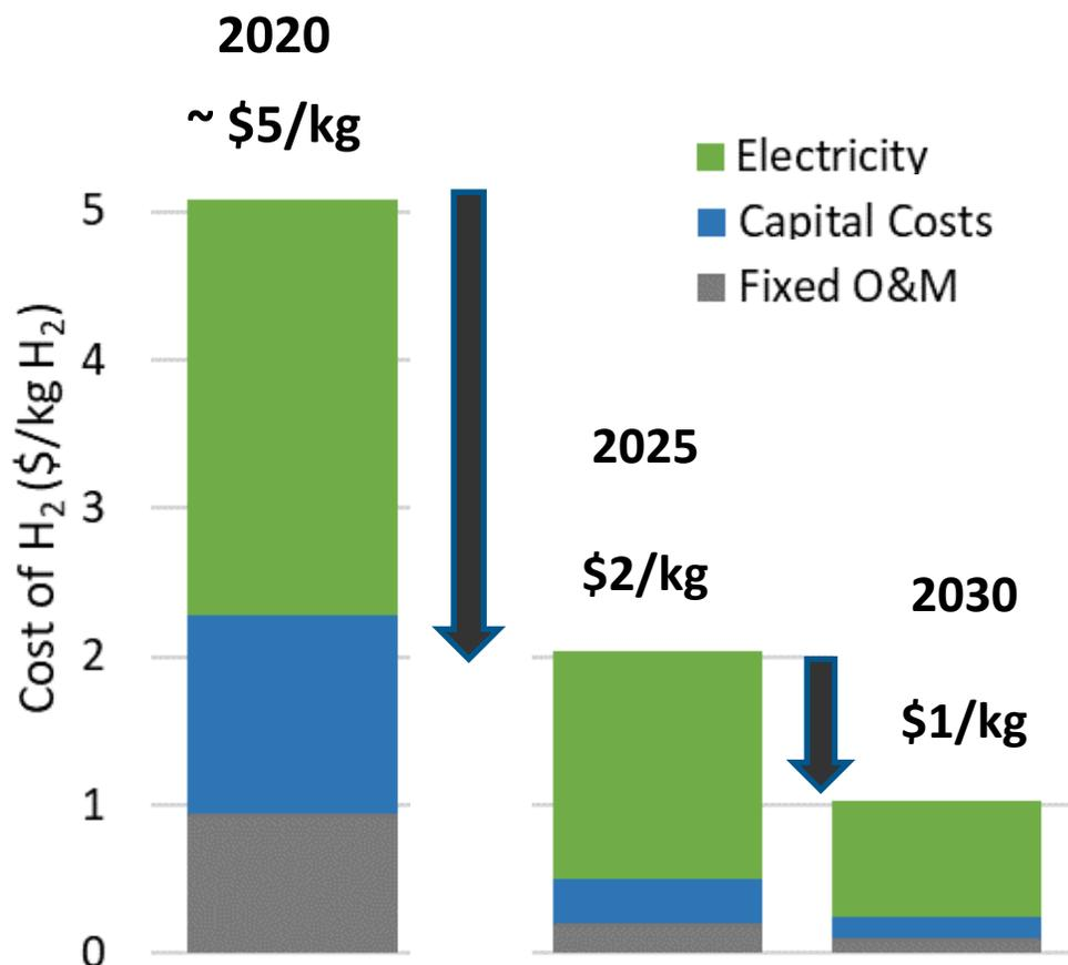
2020 Baseline: PEM low volume capital cost ~\$1,500/kW, electricity at \$50/MWh. Need less than \$300/kW by 2025, less than \$150/kW by 2030 (at scale)
