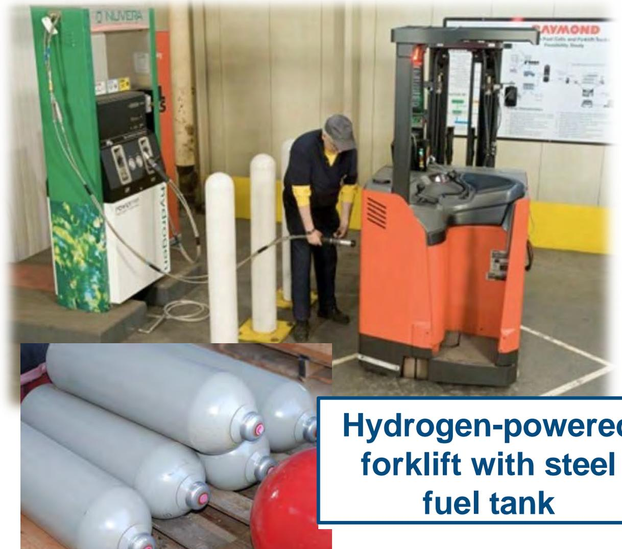
**Hydrogen-powered forklift with steel fuel tank**
