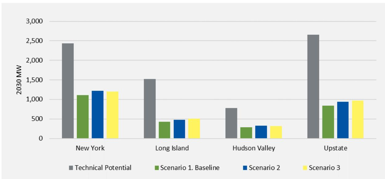
Figure 5-6 shows 2030 regional natural gas peak demand reduction. This trend closely follows the regional natural gas energy savings trend shown in Figure 5-3, with Upstate having a disproportionate share of the natural gas savings.
