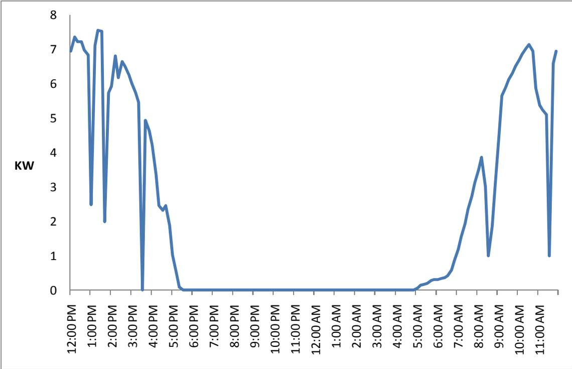
**Figure 9-5 Individual Photovoltaic Generation Variation**
