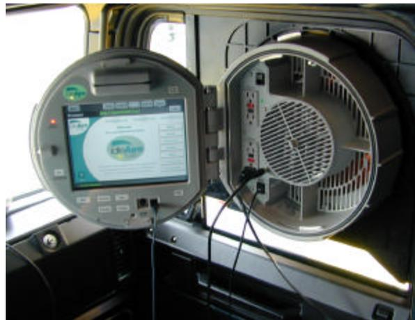
**Figure 4. Computer service console with outlets, internet & cable connections, card reader, and conditioned air delivery system**
