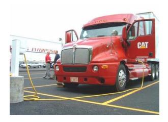
Also known as "shorepower" Dual Unit EPS systems split the requirements for installed equipment between the parking space and the parked truck. The cost is about \$5,000 per space to install and electric HVAC units average about \$4,000 per truck.
