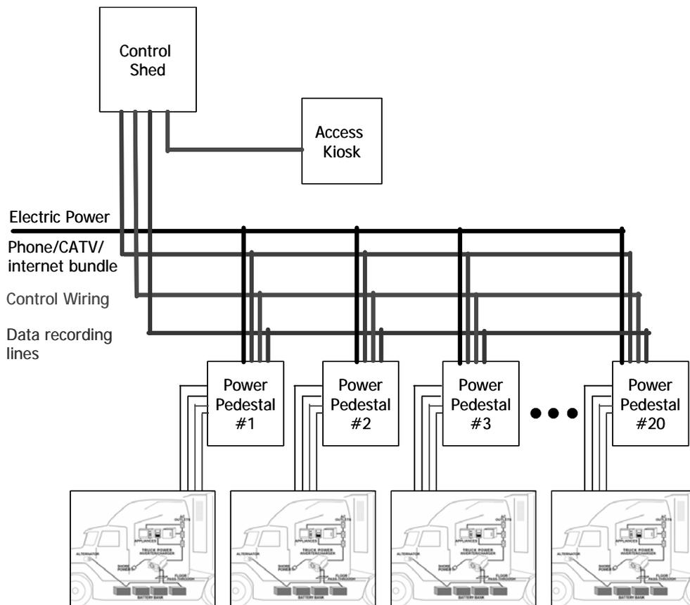
**Figure 4: Shorepower TSE system diagram**
