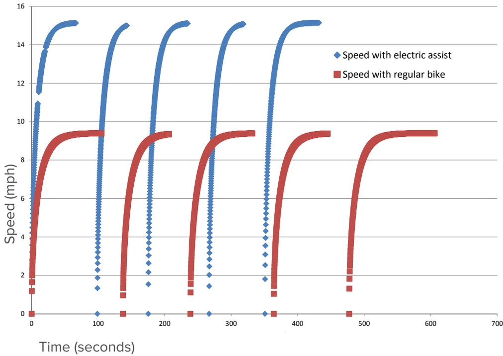
Speed-time series illustrating the electric-assist bicycle's faster acceleration from a complete stop, when compared to a standard bicycle
