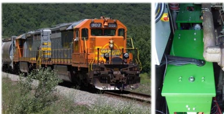
Figure 16: WCOR Locomotive #307 with a Split DWS-APU
