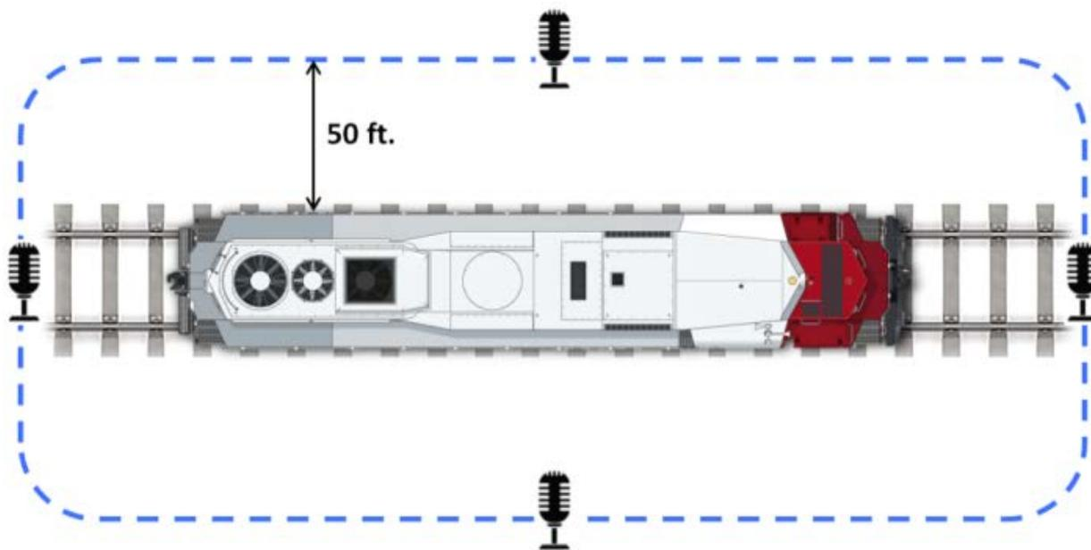
**Figure 5: Noise Reading locations (50ft Shown)**
