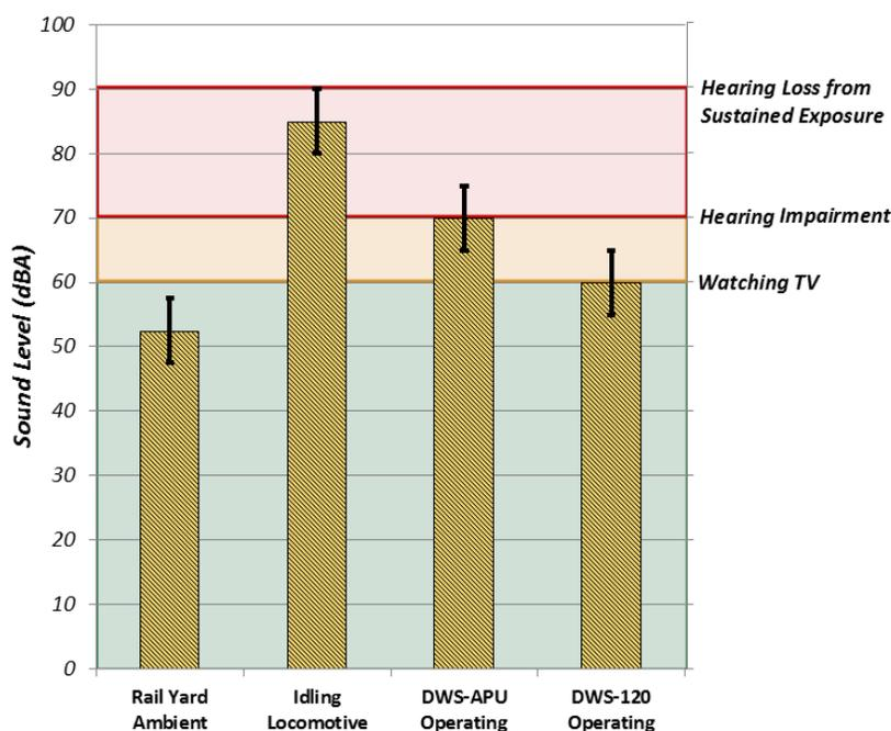
Figure 20: Locomotive Comparative Sound Levels
