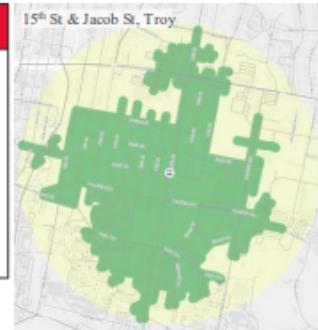
About 50% of the maximum walk radius (1/2-mile, in yellow) is accessible if following the street network (in green)
