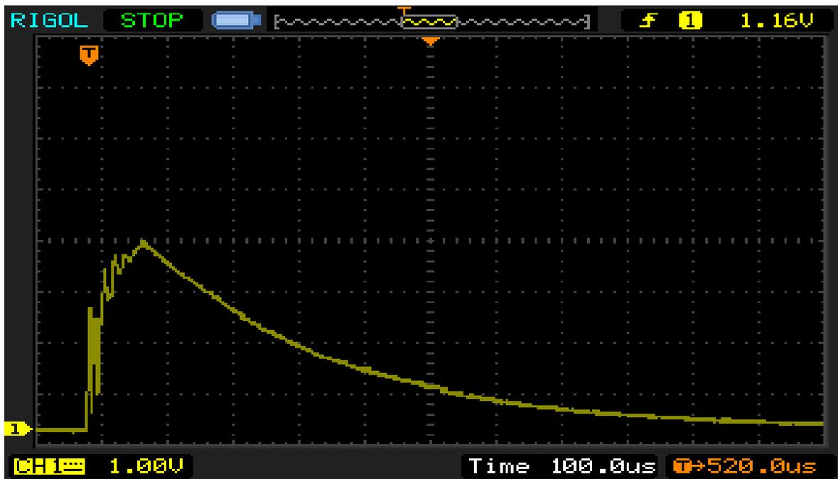
These findings were reported to the pedestrian signal manufacturer, who confirmed the results. The substantial in-rush current arises from the need of the pedestrian signal heads to store energy required to display a countdown timer during the “off” state of the flashing “DON’T WALK” signal.
