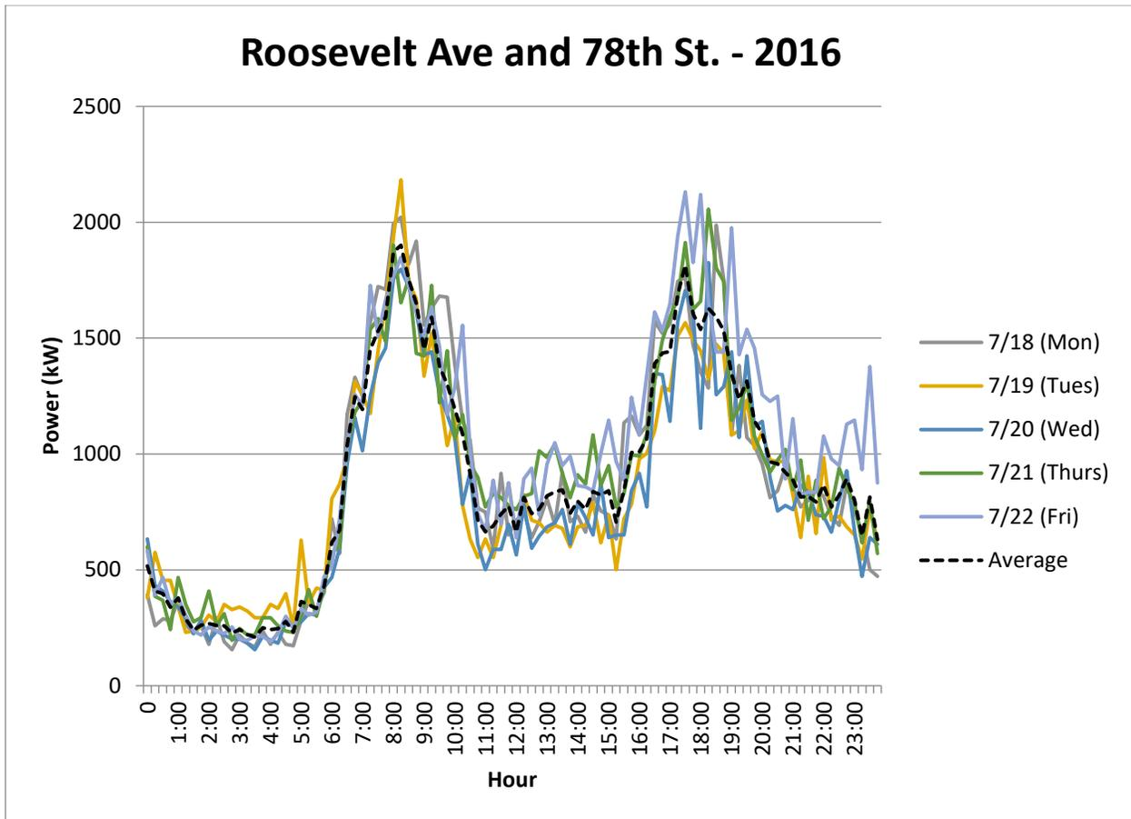
Figure 11 shows demand at the Roosevelt Avenue and 78th St. substation, one of 13 substations serving the 7 Line. Weekday peak demand occurs from about 7:00 a.m. to 9:00 a.m. and again from about 5:00 p.m. to 7:00 p.m.
