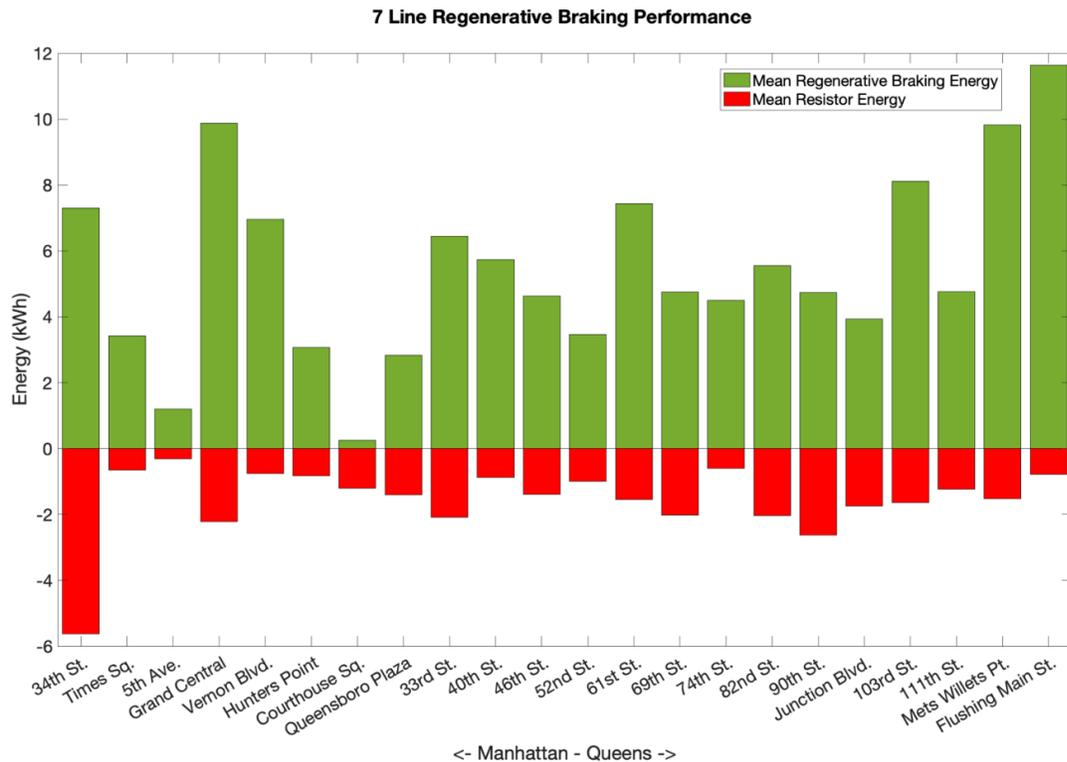
The mean regenerative energy was measured at 5.4 kWh per stop with mean resistor energy at 1.6 kWh per stop. Regenerative braking performance is variable at each stop with a standard deviation of about 2.7 kWh.
