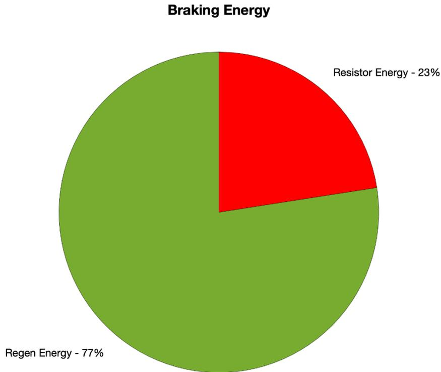
Figure 5 shows the utilization of the braking energy generated by the train.
