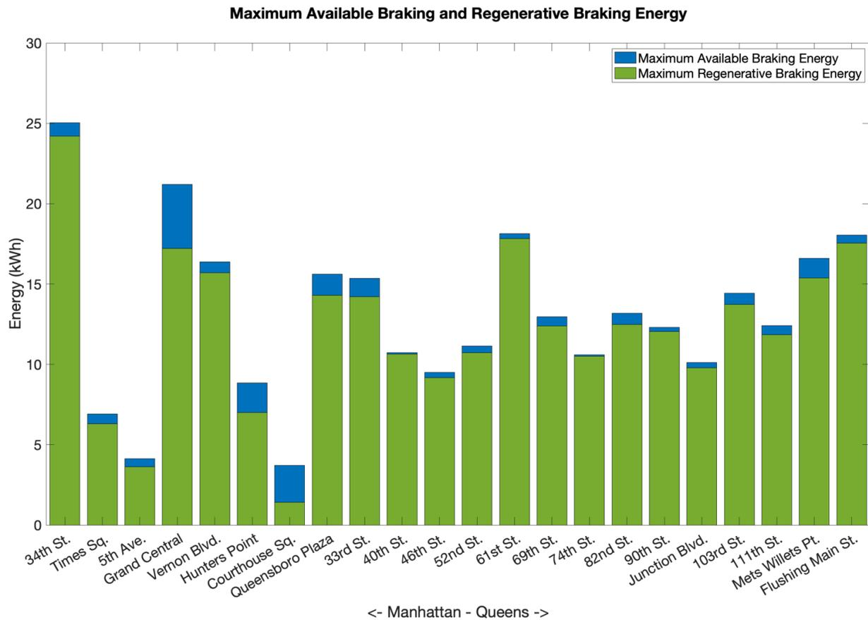
Figure 8 also reveals individual regenerative braking events delivering as much as 24 kWh. This is because in operation the 3rd rail is a complex electrical grid with multiple trains drawing power (and others braking) simultaneously. Regenerative braking performance in real-world operation is not limited to one-to-one train interaction. Substation (or wayside) ESS sizing and performance must be based on 3rd-rail grid parameters while onboard ESS designs can be based on train parameters.
