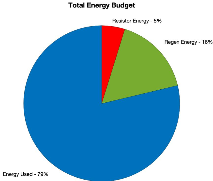
Figure 4 shows the total energy budget for a subway train operating on the 7 Line and gives the breakdown of mean energy used, mean energy returned via regenerative braking and mean energy dissipated through the onboard resistors.
