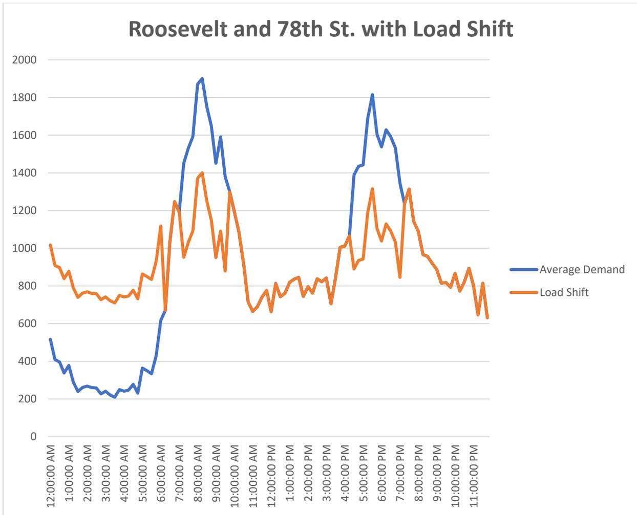
Figure 12 shows the average demand at the Roosevelt and 78th St. substation as well as the demand with load shifting ESS implemented. The ESS would charge overnight, in this case from midnight to about 6:00 a.m. The energy would be discharged into the system during peak demand periods, in this case from 7:00 a.m. to 9:00 a.m. and from 4:00 p.m. to 7:00 p.m., resulting in more than 25% demand savings.
