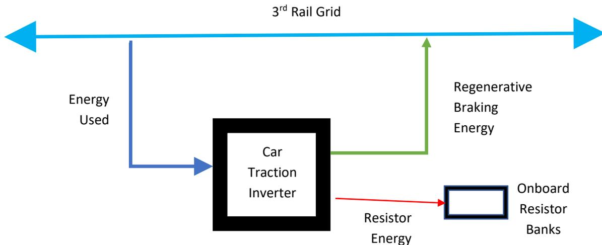
Train car traction power flow is shown in Figure 2. When the train is accelerating or cruising the energy used is drawn from the 3rd-rail grid by the traction inverters on each car. When the train is braking the energy generated by the motors goes through the traction inverters and is either returned to the 3rd-rail grid as regenerative braking energy or sent to the onboard resistor banks and dissipated as heat.
