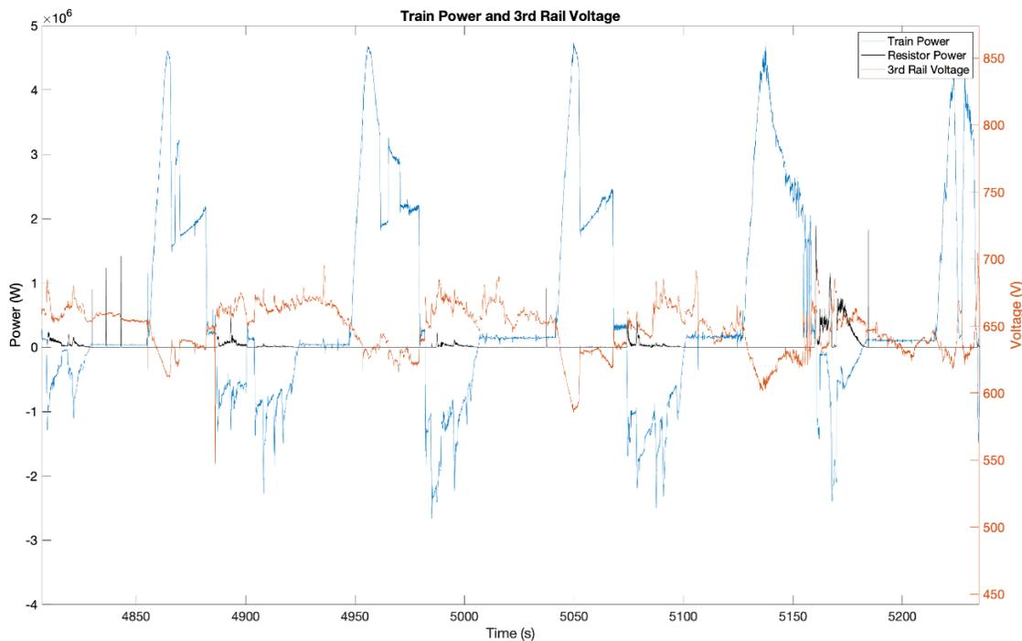
Later in the same trip, as shown in Figure 14, the baseline ESS setting of 640 V would result in ESS charging where successful regenerative braking is already occurring and little to no resistor energy is being produced (time 4980 s). This, along with the moderate 3rd-rail voltage variation when the train is accelerating (4950 s), which would result no ESS discharge and in no energy savings.
