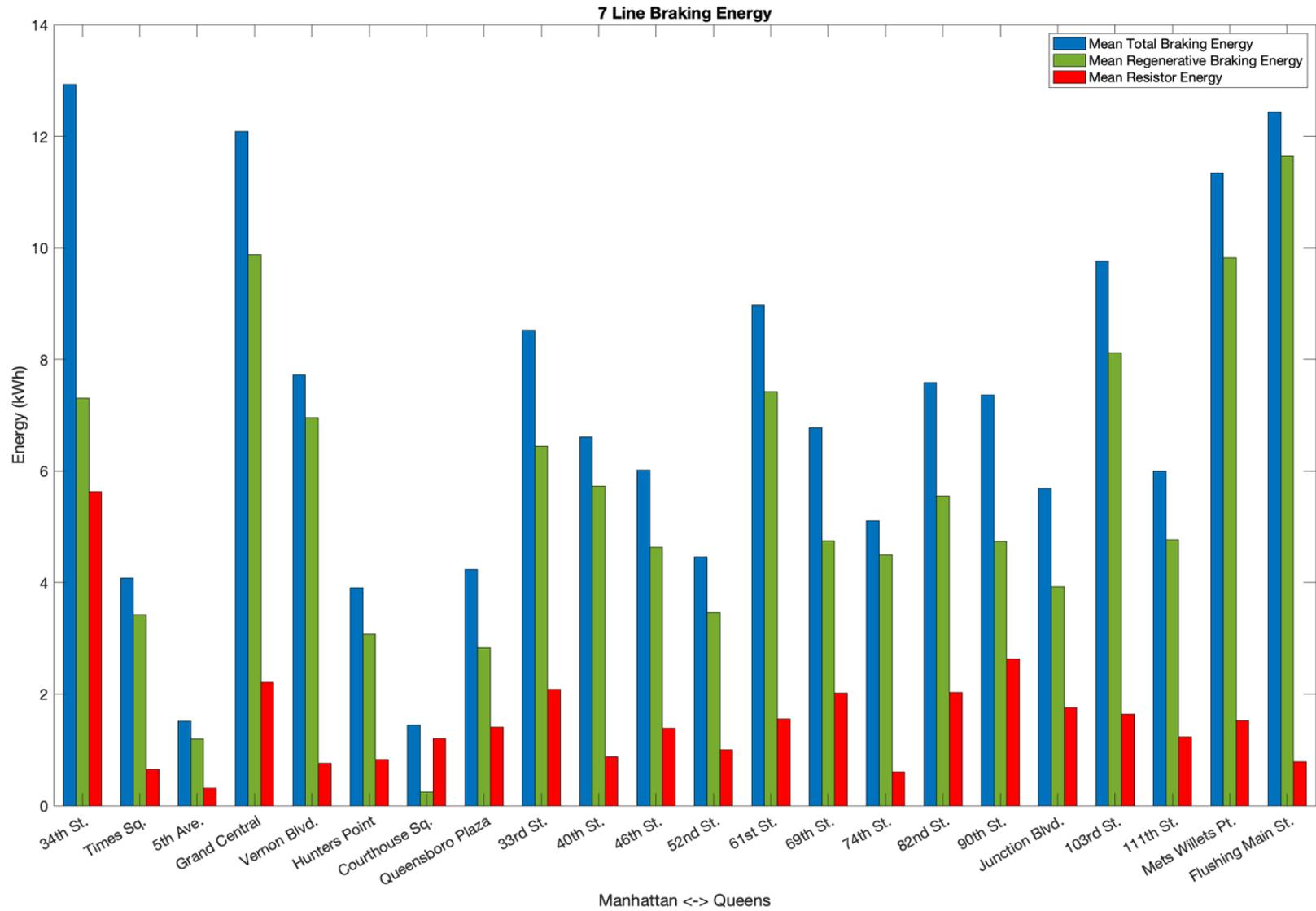
The mean total braking energy generated by a braking train is 6.7 kWh per stop. The amount of total available braking energy for any individual stop is dependent on multiple factors:
