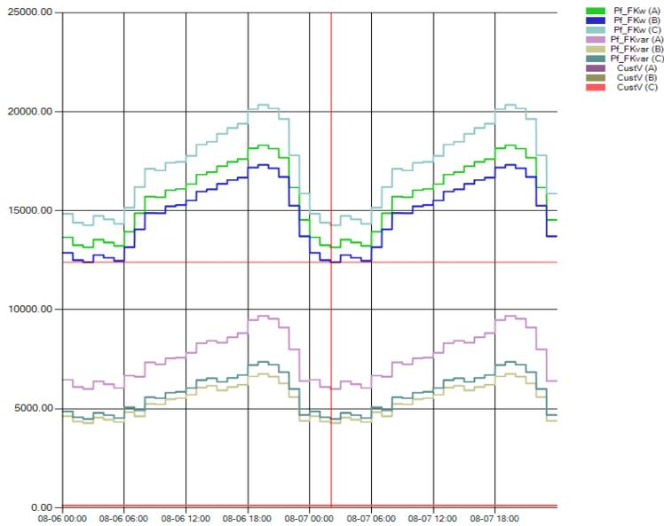
**Figure 4-2. Feeder Base Case Power Flow**
