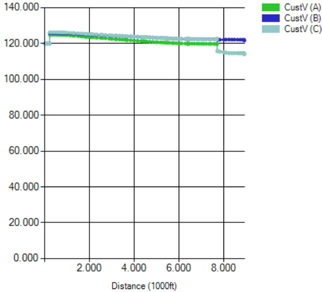
**Table 4-7. Power flow min and max results for 20 percent penetration (DC Fast Charging only)**
