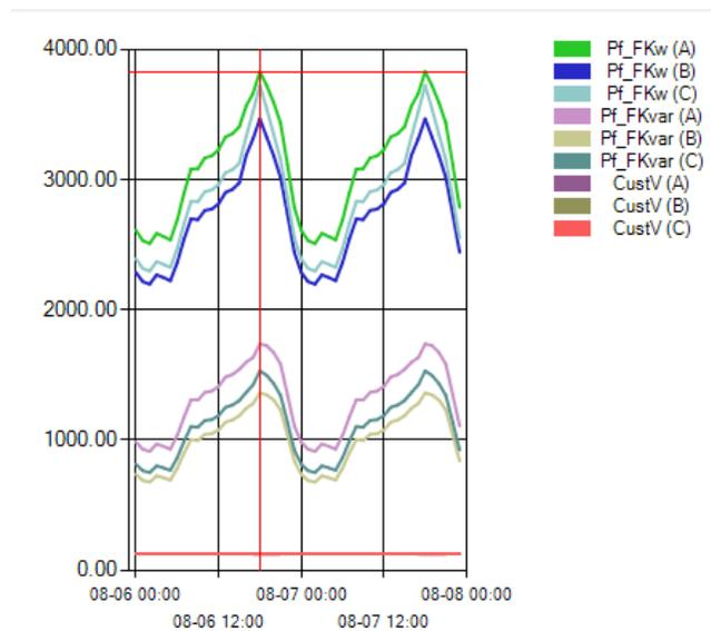
Figure 4-20. Power Flow for Feeder with 10 percent Penetration of EVs and Only Level 2 Home Charging
