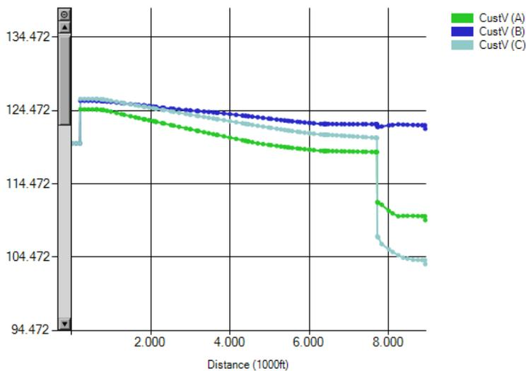
**Figure 4-17. Voltage Distance Plot for Feeder (Line Segment 2) with 20 percent penetration of EVs with Level 2 and DC Fast charging scenario**
