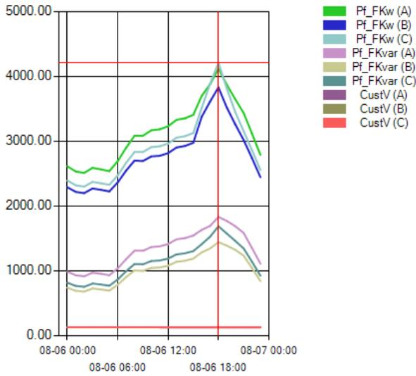
Figure 4-23. Power Flow Comparison for the Level 2 Charging Scenarios
