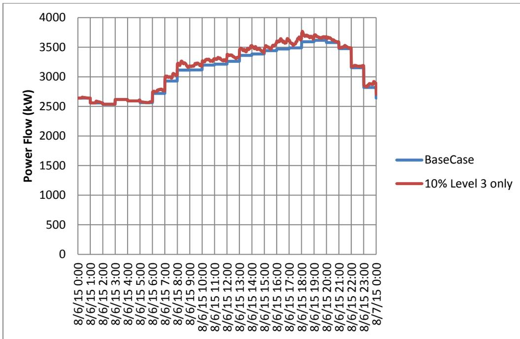
**Table 4-5. Feeder Power Flow Results and Base Case Comparison**
