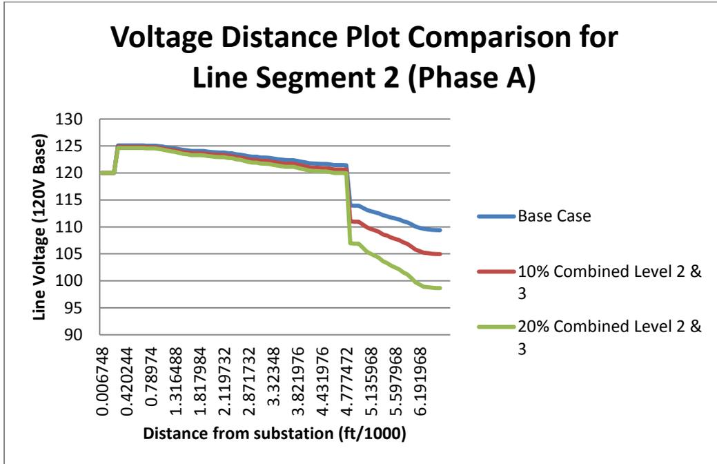
**Table 4-15. Power Flow Results for Feeder for 20 percent EV Penetration with Level 2 & DC Fast Charging Scenario**
