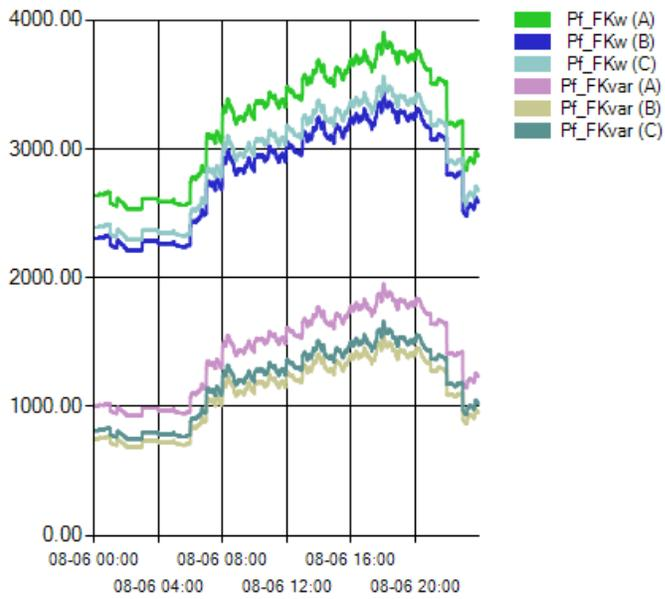
**Figure 4-5. Comparison of A-Phase Power Flow with Base Case, 10 percent, and 20 percent Penetration (with DC Fast charging only)**
