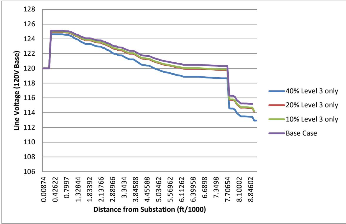
**Figure 4-11. Line Segment 2 Voltage Distance Plot Comparison (DC Fast only)**
