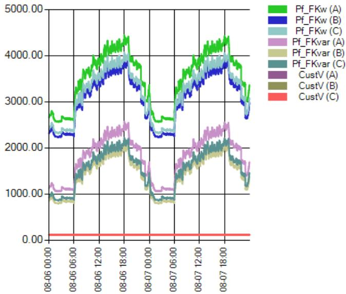
**Figure 4-9. Power Flow Comparison with DC Fast Charging only**
