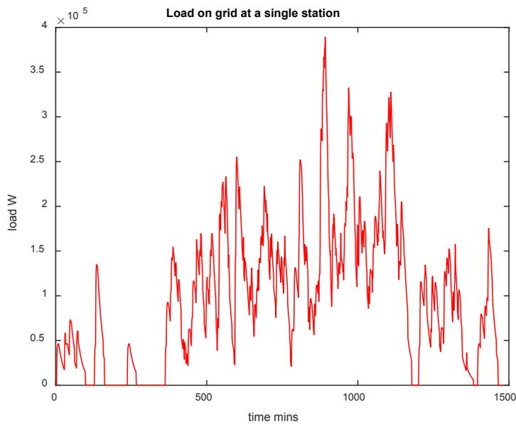
Multiple DC Fast charging station load profiles are created using this model unless the number of chargers in the system is equal to the number of chargers per station. Each load profile differs a bit. For the purpose of testing, five of these DC Fast charging station load profiles were added to the DEW database to test the effect.
