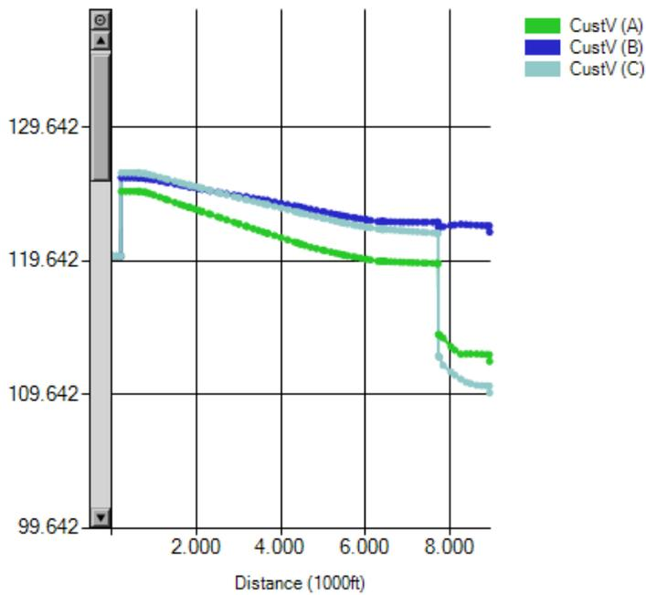
**Figure 4-14. Voltage Distance Plot Comparison (Phase A, Line Segment 2, 10 percent Penetration Combined Level 2 and DC Fast Charging)**
