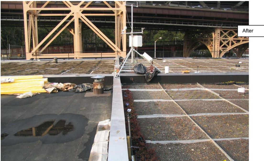
Thermocouple wires, flow meter wires, power cable and telephone cables run out of the gooseneck from the building at Quad I
