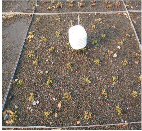
Installation of Heat Flow Sensor and Water Content Reflectometer
