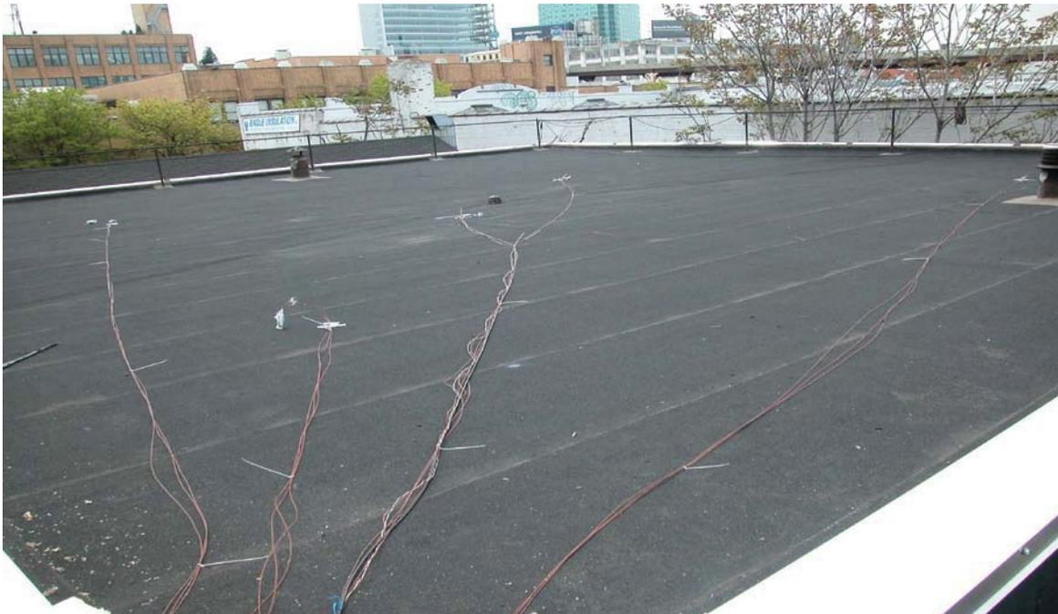
Installation of TI, TM, TT and TA Thermocouples. TI is at the ceiling inside the building. TA is covered by radiation shield.
