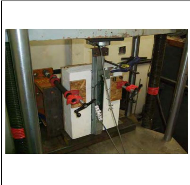
**Figure 20. Cladding Connections to Steel Framing**
