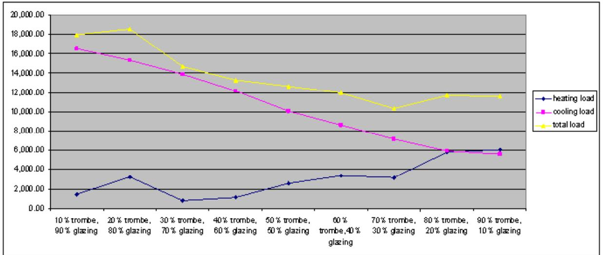
Figure 2 - Chart illustrating heating and cooling trends when altering trombe-to-glazing ratios.
