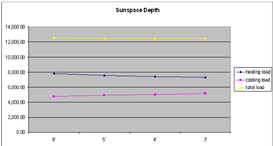
Figure 3b - Chart illustrating heating and cooling trends when altering sunspace depth.
