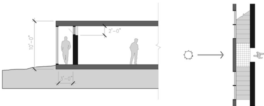
Figure 3d - Illustration of best practice sunspace condition (left). One alternative solution (right).
