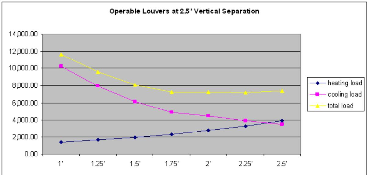
Figure 2e - Chart illustrating heating and cooling trends when altering operable louver projections.
