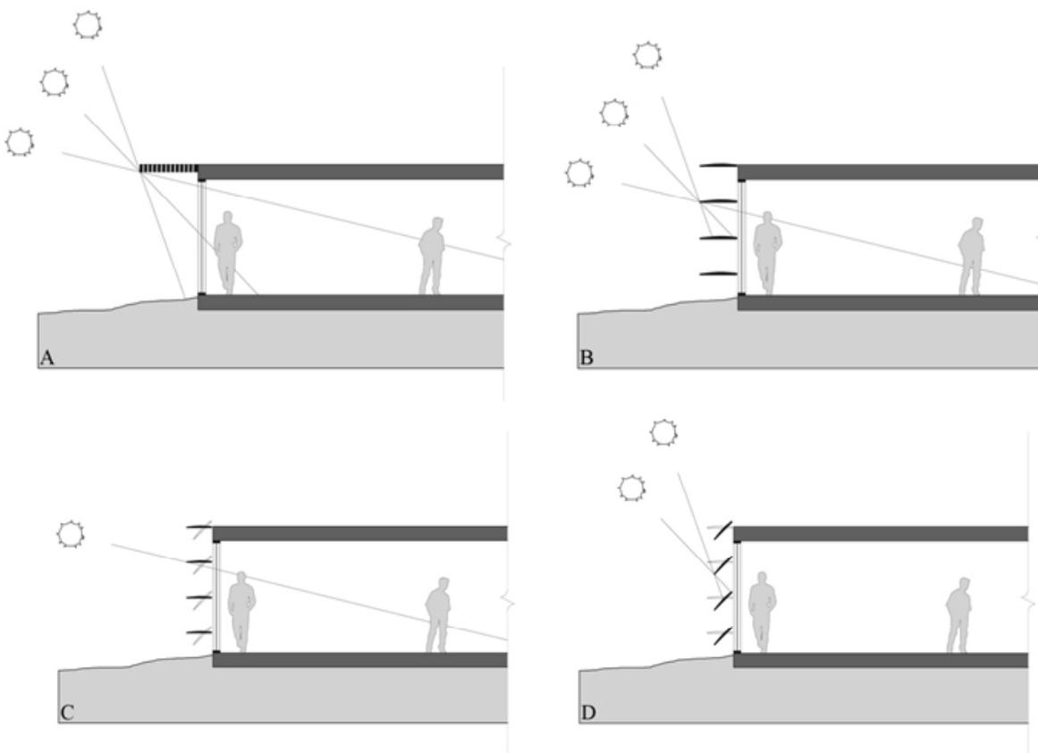
Figure 2g – Illustrations of different shading options – (A) Fixed overhang at 4 feet (B) Fixed louver at 2.5 feet (C) Winter operable louver at 1.75 feet (D) Summer operable louver at 1.75 feet
