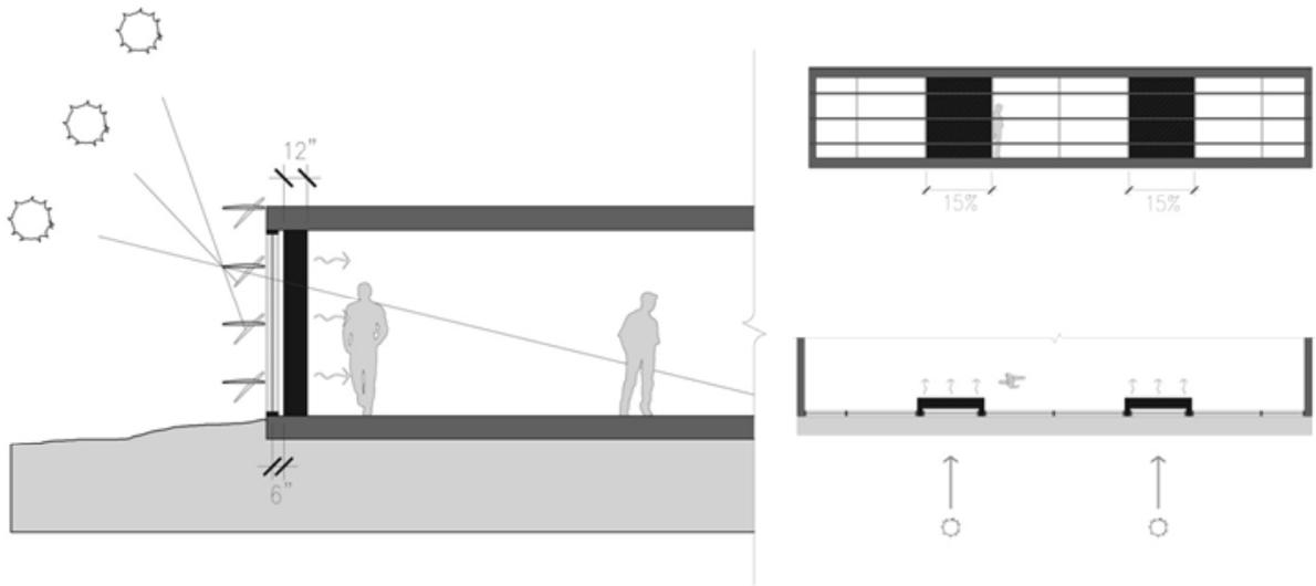
Figure 2h – Illustrations of optimum trombe application (correct louvers, cavity spacing, trombe width and a 30% trombe/70% glazing elevation and plan)
