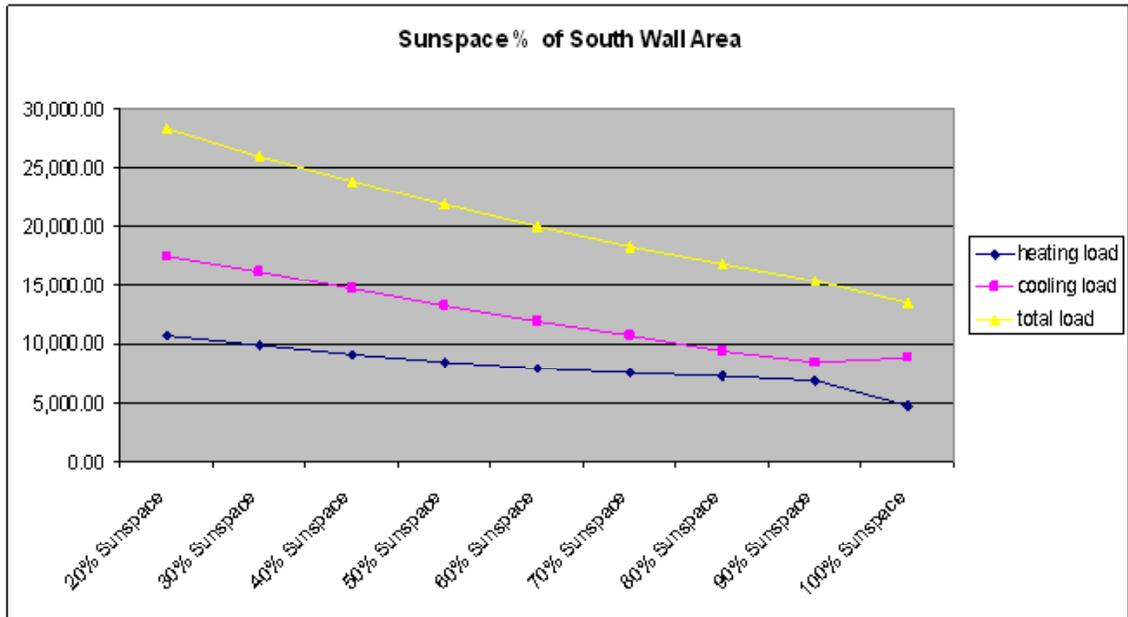
Figure 3c - Chart illustrating heating and cooling trends when varying sunspace as a percentage of overall south facing wall.
