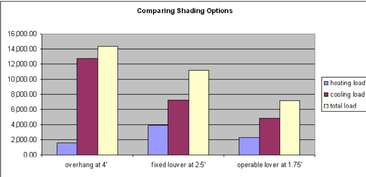
Figure 2f - Chart illustrating differences in performance between best versions of different shading options.
