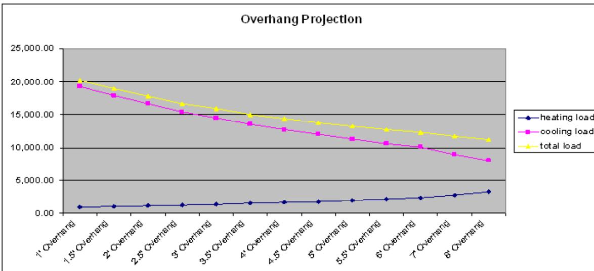
Figure 2c - Chart illustrating heating and cooling trends when altering overhang projections.
