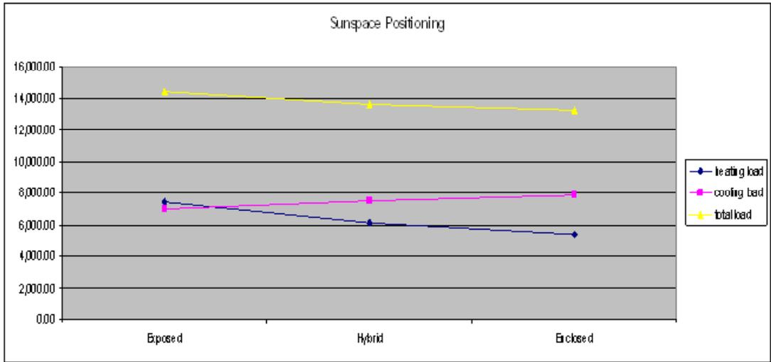
Figure 3 - Chart illustrating heating and cooling trends when moving between internal and external sunspaces.
