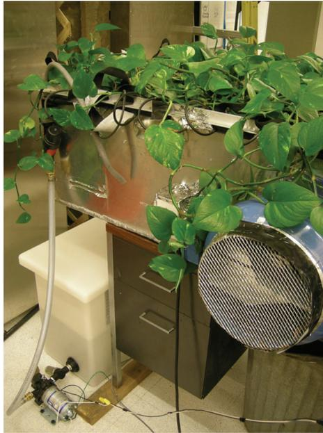
**Figure 3-1. Modified bio-filtration system**
