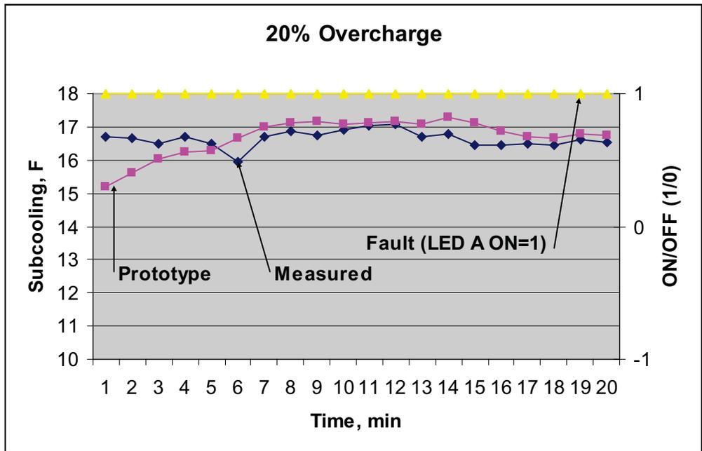
**Figure 4-11 Subcooling Profile Along with ON/OFF Status for the 20% Overcharge Case.**
