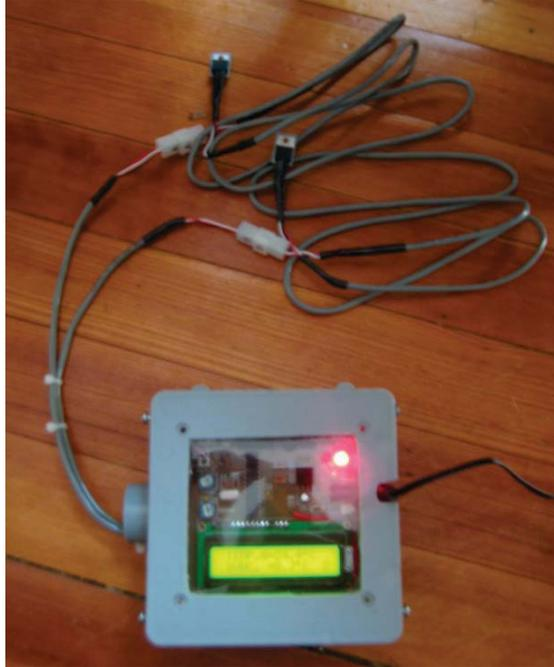
**Figure 4-4 Field-Ready Refrigerant Charge Fault Detector Prototype Built by SWA.**
