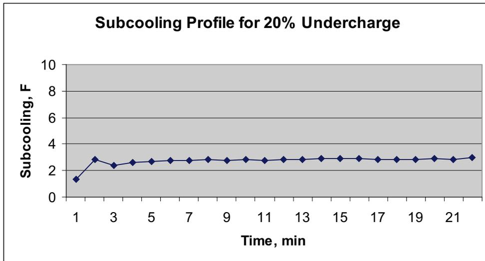
**Figure 3-8 Refrigerant Subcooling as a Function of Time for 20% Undercharge.**
