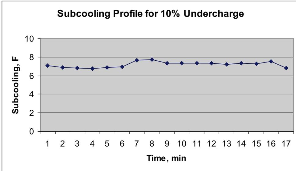
**Figure 3-7 Refrigerant Subcooling as a Function of Time for 10% Undercharge.**
