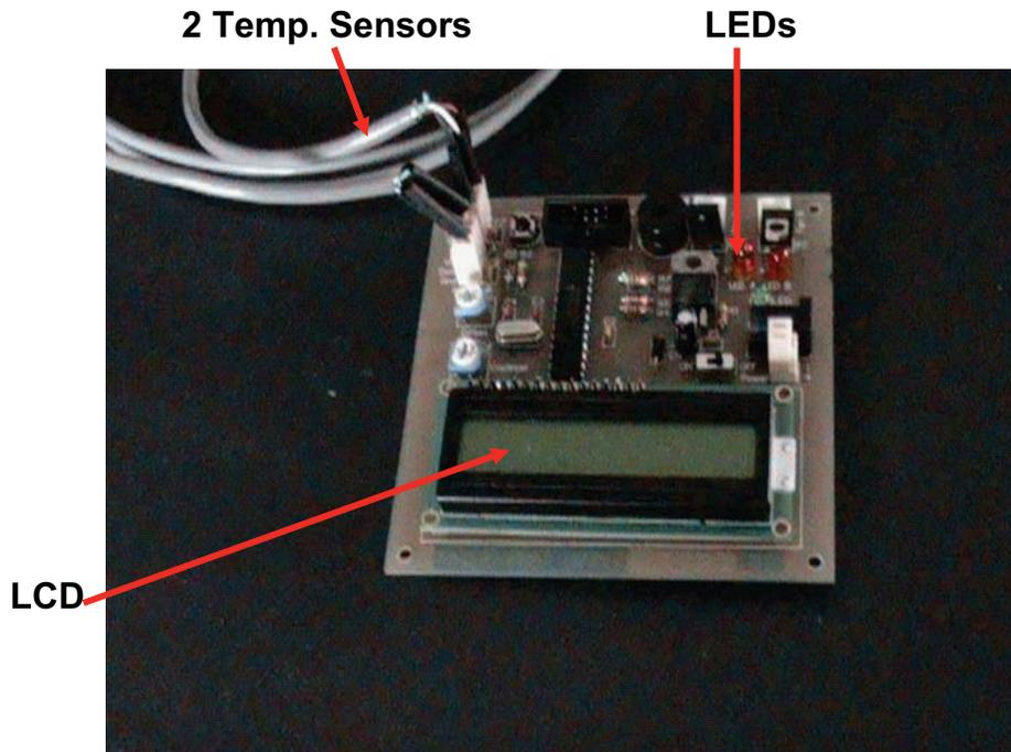
**Figure 2-9 A Differential Temperature Prototype Built by SWA for Sensing Subcooling and Diagnosing Charge Fault.**
