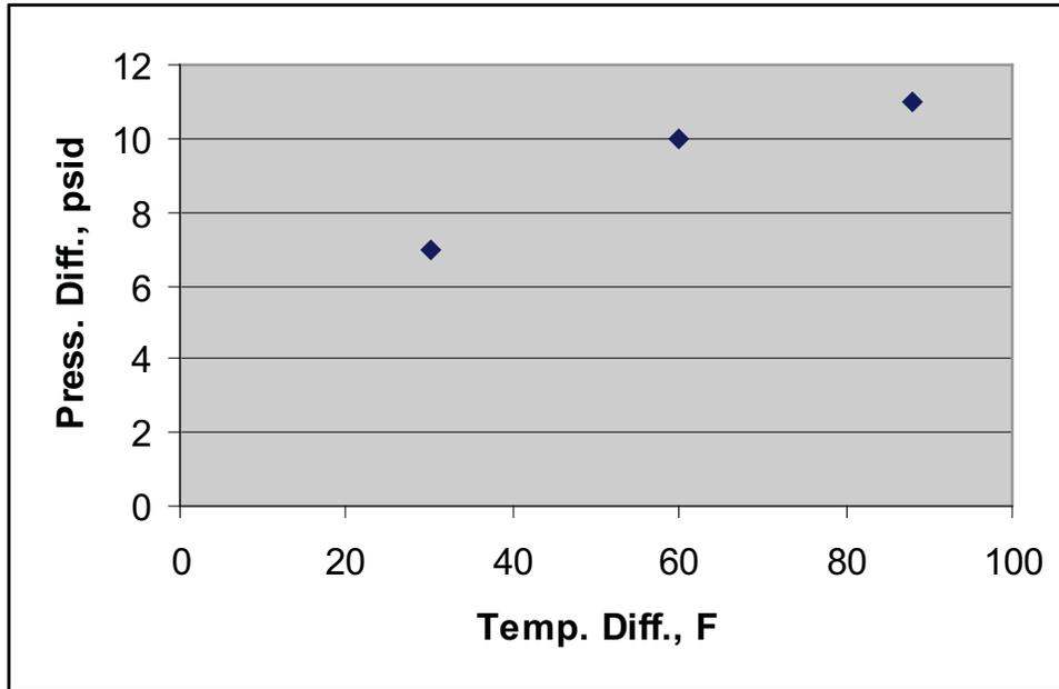
**Figure 2-5 Measured Pressure Differential as a Function of the Measured Temperature Differential Using the Pressure Differential Prototype.**
