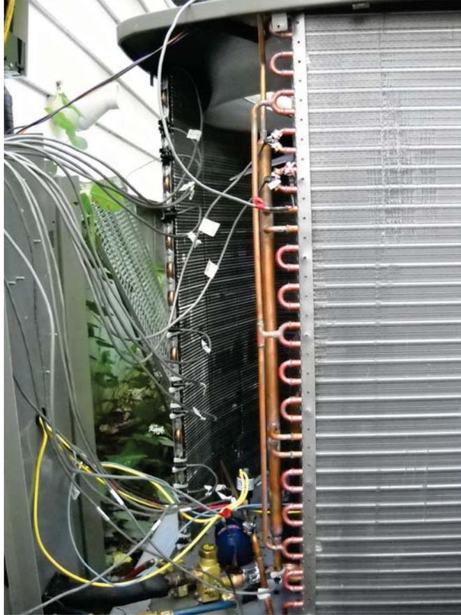
**Figure 3-3 Condenser Coil (Outdoor Unit) with Temperature Sensors Placed.**
