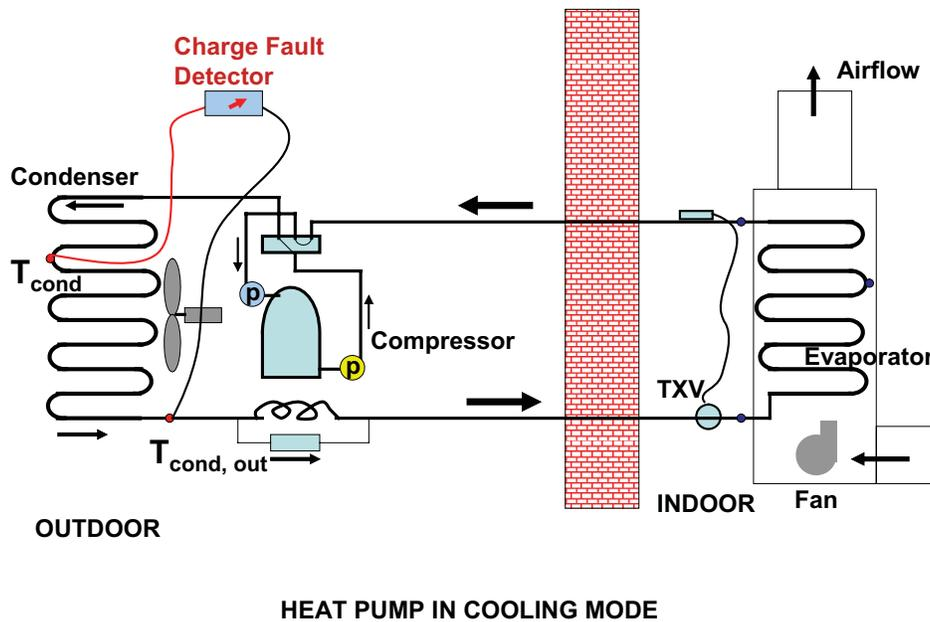
**Figure 2-7 A Concept of Measuring Subcooling for Charge Fault Detection.**
