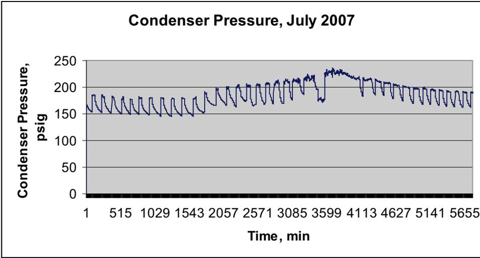
**Figure 2-3 A Condenser Pressure Profile of an R-22 System.**
