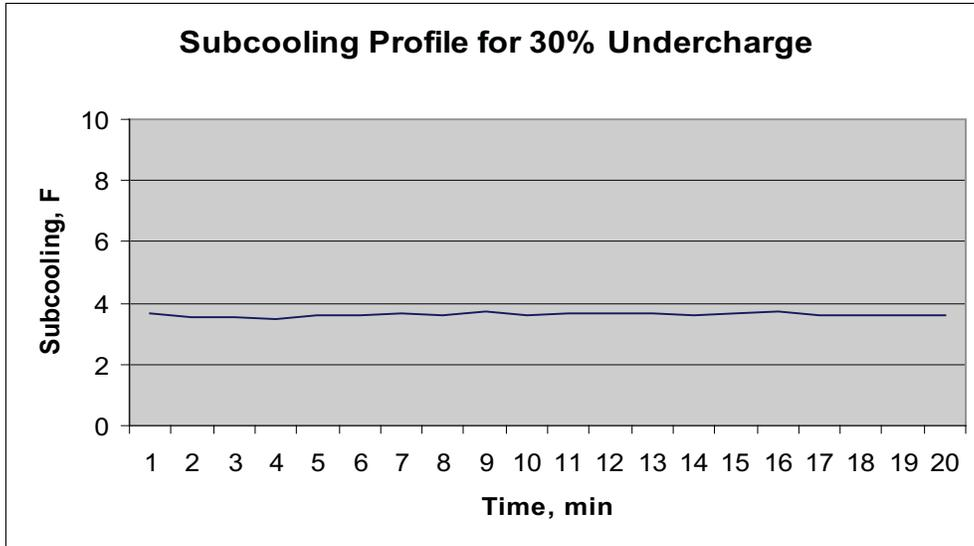
**Figure 3-9 Refrigerant Subcooling as a Function of Time for 30% Undercharge.**
