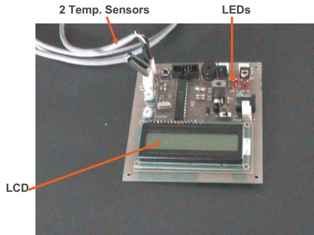
**Figure 4-3 Digital Prototype Built by SWA for Refrigerant Charge Fault Detection.**
