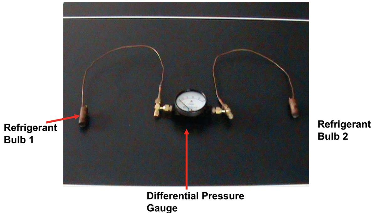
**Figure 2-4 A Breadboard Prototype for Detecting Refrigerant Charge Fault Employing Differential Pressure Sensing.**
