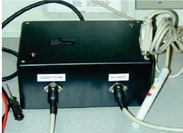
**Figure 4-1 A Pre-Prototype Charge Detector Built by Oak Ridge National Laboratory.**
