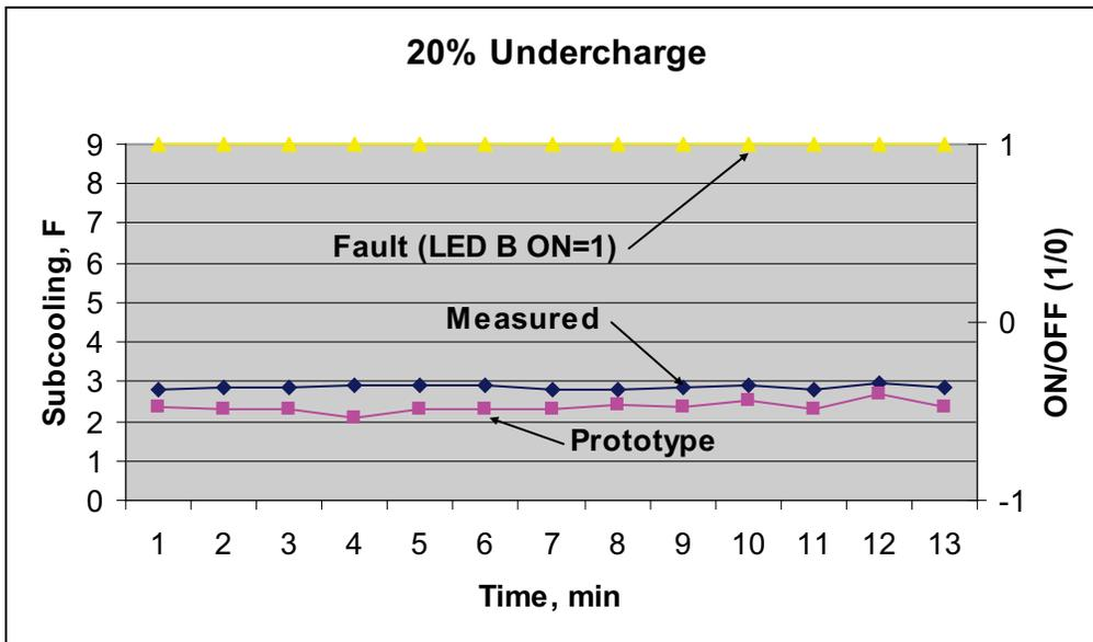
Figure 4-9 Subcooling Profile Along with ON/OFF Status for the 20% Undercharge Case.
