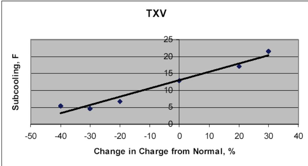
**Figure 3-13 Condenser Subcooling as a Function of R-410A Refrigerant Charge (SWA data).**
