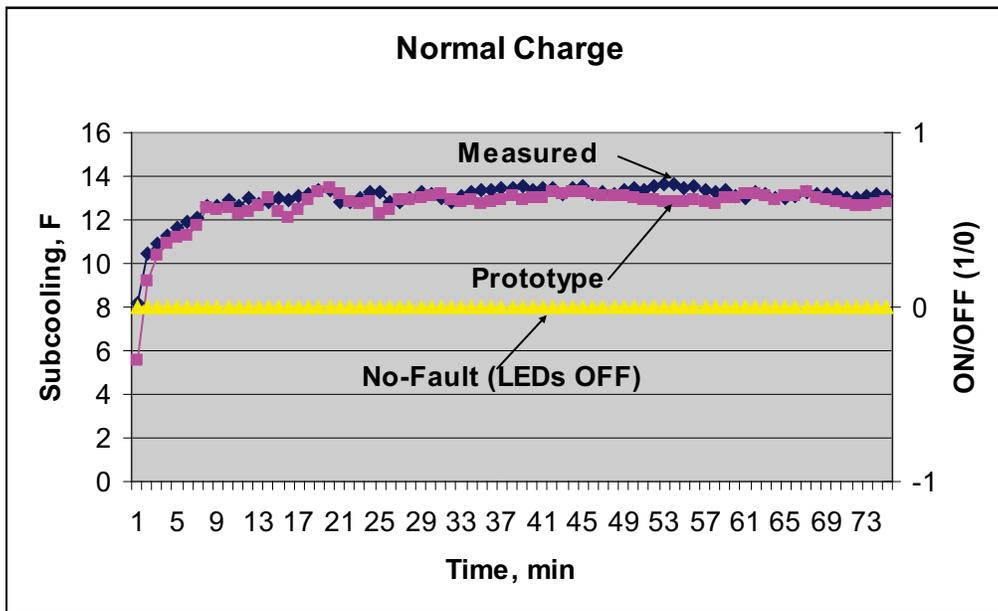
**Figure 4-7 Subcooling Profile Along with ON/OFF Status for the Normal Charge Case.**
