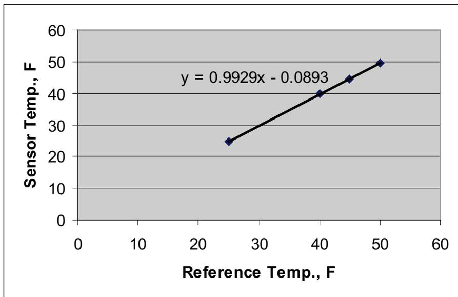
**Figure 2-12 Agreement Between the Prototype's Temperature Sensor and the Reference Temperature.**
