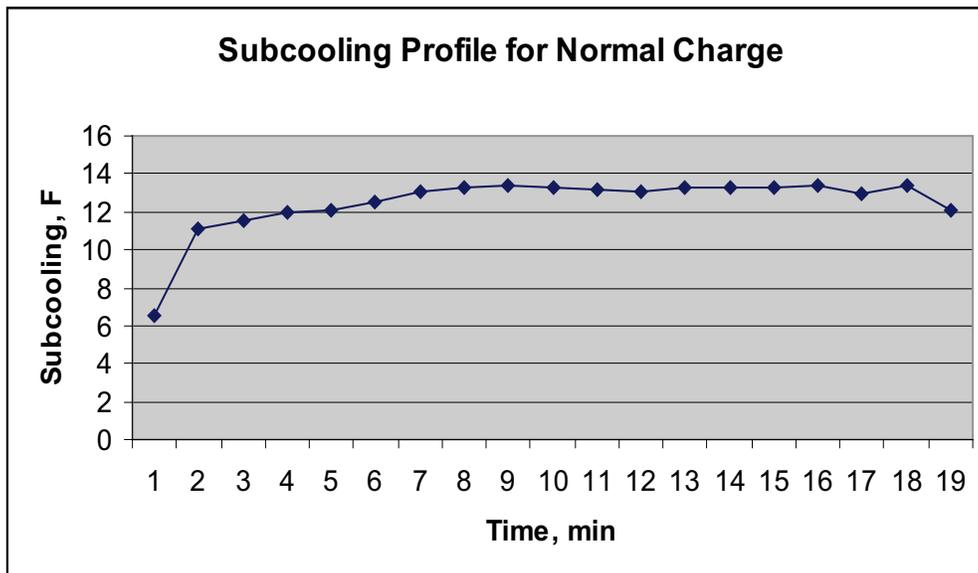
**Figure 3-6 Refrigerant Subcooling as a Function of Time for Normal Charge.**
