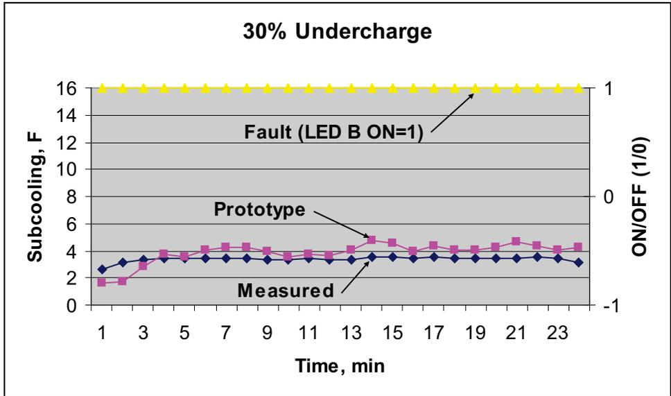
**Figure 4-10 Subcooling Profile Along with ON/OFF Status for the 30% Undercharge Case.**
