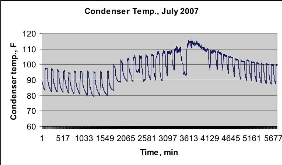
**Figure 2-2 A Condenser Temperature Profile of an R-22 System.**
