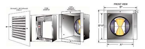
Figure 2. CAR damper shown in exhaust grill assembly
