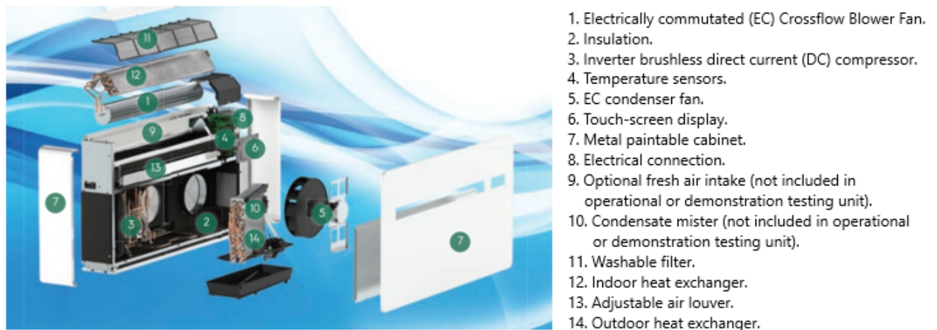
Figure 2. Innova HPAC 2.0 Components
