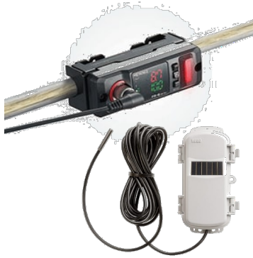
Figure 17. Hydronic Flow and Temperature Measurement Systems for Baseline Heating Energy Measurements
