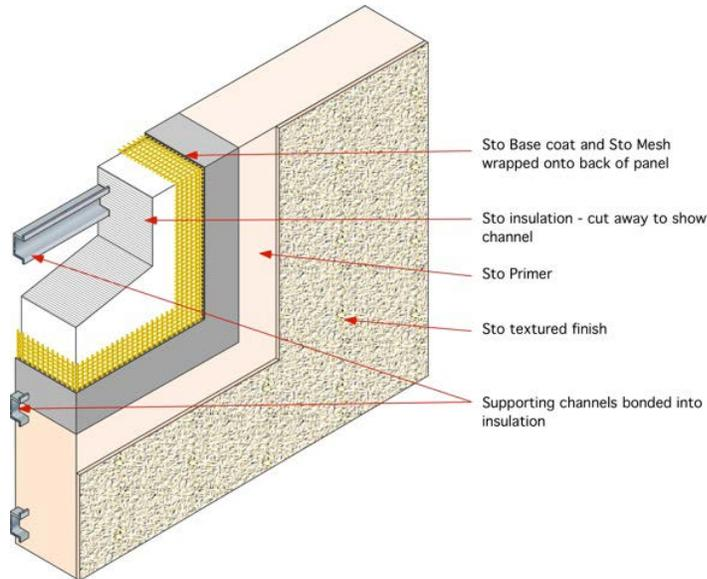
While the final appearance of an EIFS installation resembles stucco, it is a distinctly different system. Stucco is a generic cementitious-based material, whereas EIFSs are proprietary synthetic formulations distributed by manufacturers to a network of authorized applicators. An EIFS is composed of polymeric (organic) bonded aggregate and cement reinforced with a glass mesh. Stucco is made of inorganic cement, sand, and lime.
