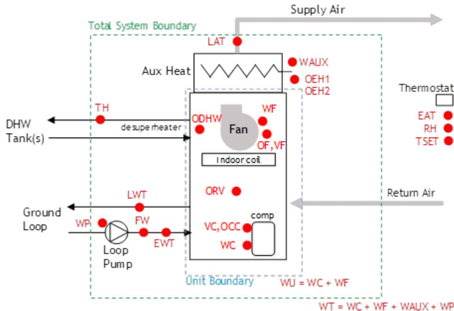
Most of these points are direct measurements by temperature sensors, flow meters, and refrigerant pressures. Refrigeration saturation temperatures, superheat temperatures, and subcooling temperatures are determined using the measured readings combined with refrigerant property calculations.
