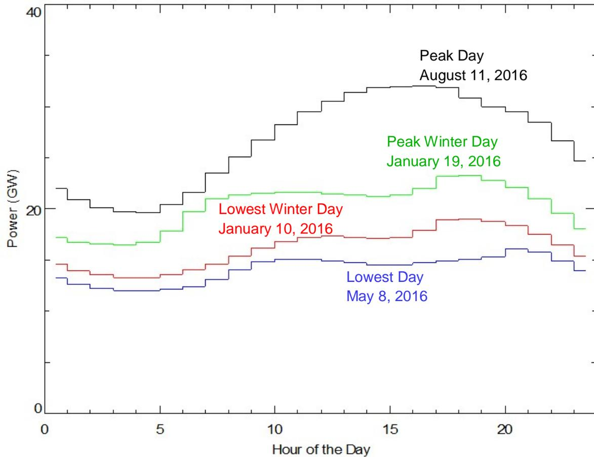
Geothermal heat pumps will result in a similar load shape as air conditioners for the summer, though with a potentially 40-50% lower electric demand per ton because of their higher cooling efficiency as shown by the data in Figure 16.<sup>8</sup> The winter load shape for geothermal heat pumps has the potential to “fill in” the early morning valley in the State’s current electric load profile.
