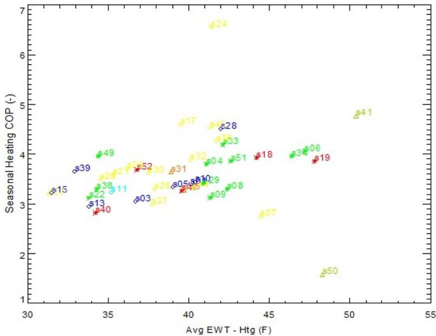
**Figure 14. Distribution of Corrected Heating COPs—by Loop Type and for Total Sample**
