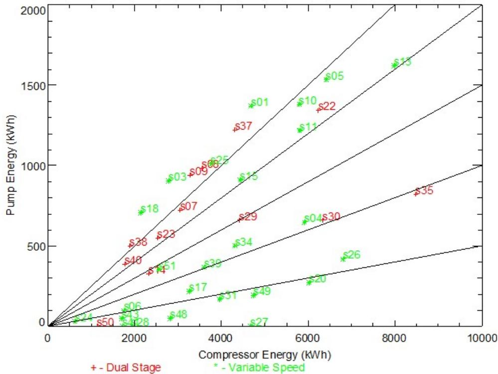
Figure 19 shows how the corrected seasonal system heating COP varies with the pump-to-compressor energy ratio. At ratios near 0.05, the average COP is near 4.0. As the ratio approaches 0.2, the average COP drops closer to 3.0. While the pumping energy reported by Symphony may be questionable in some cases, this overall trend appears to reinforce the importance of minimizing pumping power to improve COP.
