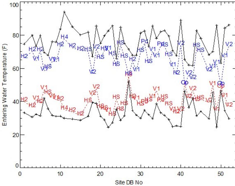
**Figure 5. Comparing Entering Water Temperatures for Different Loop Types**
