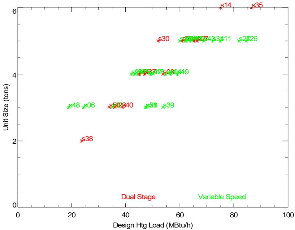
Figure A-2. Comparing Selected Heat Pump Unit Size to Design Heating and Cooling Loads
