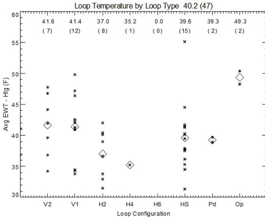
**Figure 6. Comparing Minimum and Average Entering Water Temperatures for Different Loop Types (\*=vertical bores; ◇= horizontal loops; △= other loops)**
