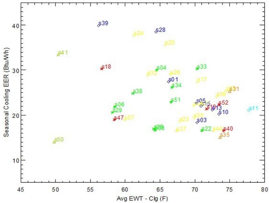
Figure 16. Distribution of Corrected Cooling EERs—by Loop Type and for Total Sample
