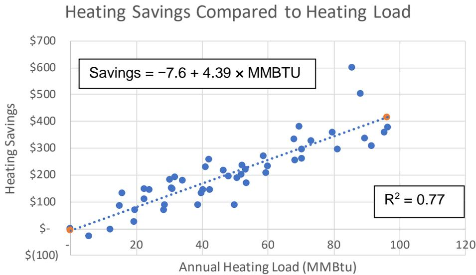
**Figure 29. Trend of Heating Cost Savings with Annual Heating Load—Propane**
