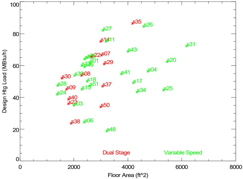
Figure A-1. Comparing Design Heating and Cooling Loads to House Floor Area
