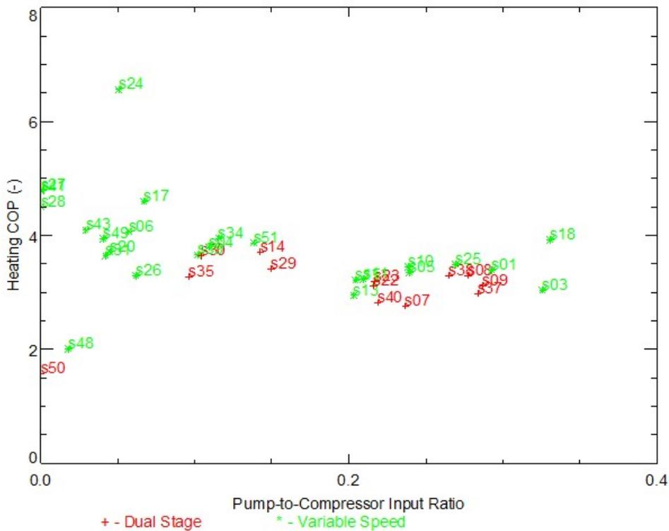
The on-site measurements from Site S8, a dual stage unit where the contractor installed two staged pumps in series, confirmed the relatively poor performance of this pumping arrangement and control strategy compared to variable speed operation. Table 12 shows the pumping power determined by the on-site measurements. The pump-to-compressor power ratio was 13% at high stage and 11% at low stage.
