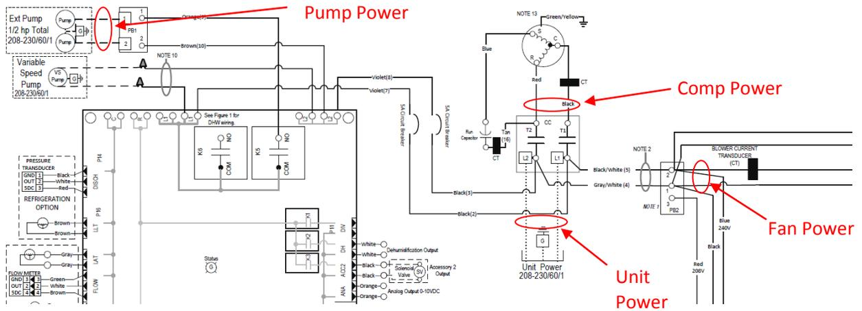
Figure B-4. Locations for Handheld Power Readings
