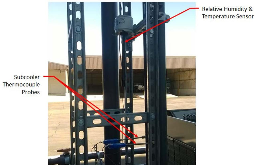
**Figure 10. Thermocouple attached to the refrigeration copper tube**
