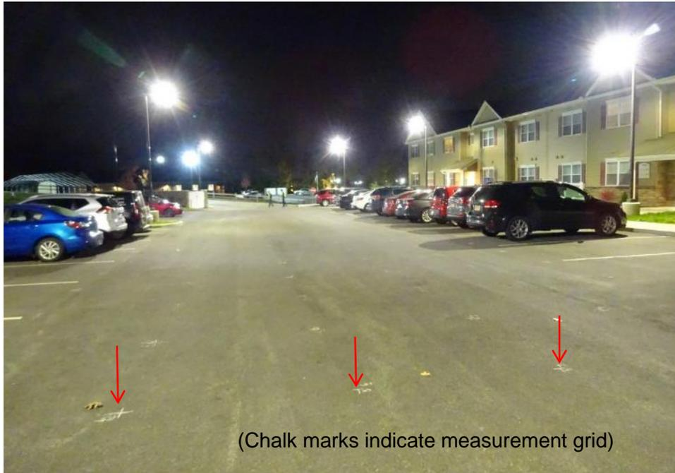
For other outdoor spaces such as sidewalks or lawn areas, IESNA has not established a recommended measurement point for spacing. Therefore, LRC measured lights landing on relevant surfaces (on the ground, on garbage can lids, door handles, etc.) at a regular interval as shown above.
