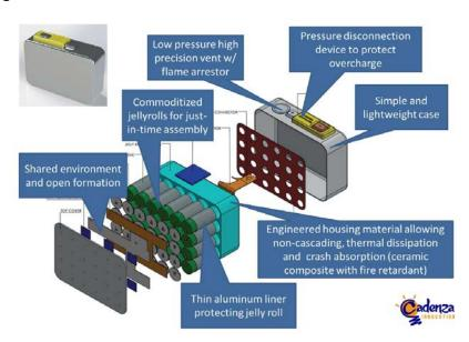
Figure 1. Schematic of the Cadenza Multi-Roll Architecture Platform (the supercell)
