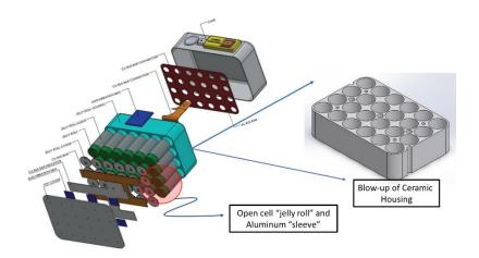
Figure 3 focuses on the pressure disconnect device and the case vent in the Cadenza supercell platform. These features, combined with the ceramic housing shown in Figure 2, protect the system, substitute for the traditional approach of individual sealed lithium cells, and prevent the potential risk of cascading thermal impacts throughout the cell and significantly lower the overall cost of the system.
