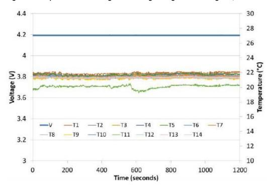
Figure 8. Temperature and voltage monitoring during crush testing at 1,000x cell weight
