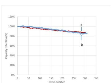
Figure 11. Comparison of the cycle life between the Cadenza supercell vs. stand-alone, lithium-ion cell
