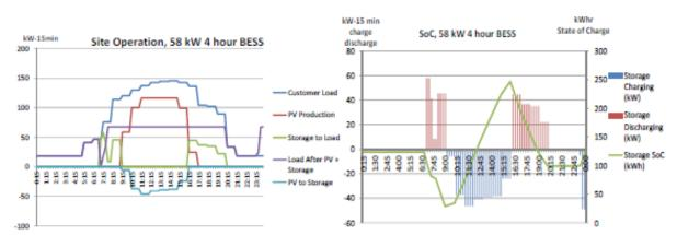
Figure 16. Site Operation and Storage Charge/Discharge Profiles in Demand Reduction Case
