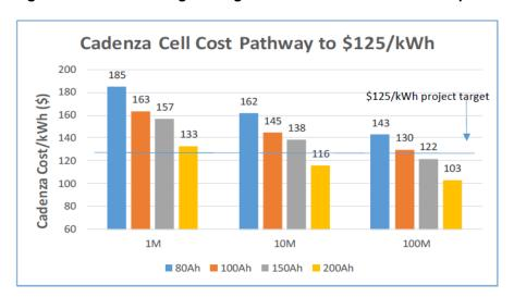
Figure 15. Manufacturing costing estimates for the Cadenza cell/platform
