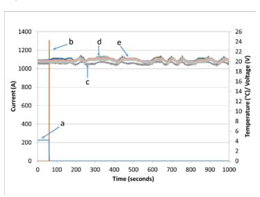
Figure 6. Temperature, voltage and current profiles for external short circuit test of 83 Ah supercell at 100% SOC
