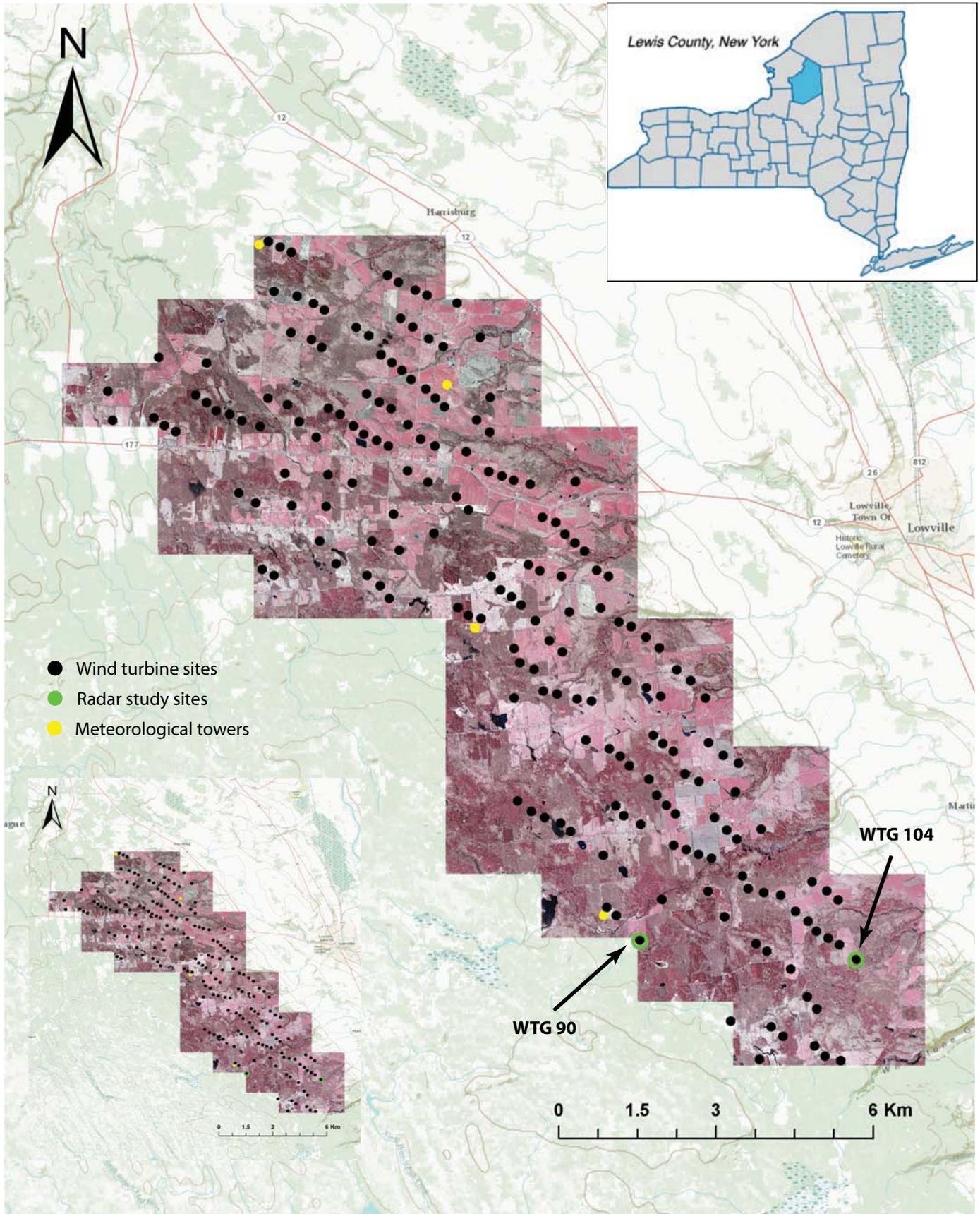
Figure 7. Map showing wind turbine sites, radar study sites and meteorological towers at the Maple Ridge Wind Power Facility.
