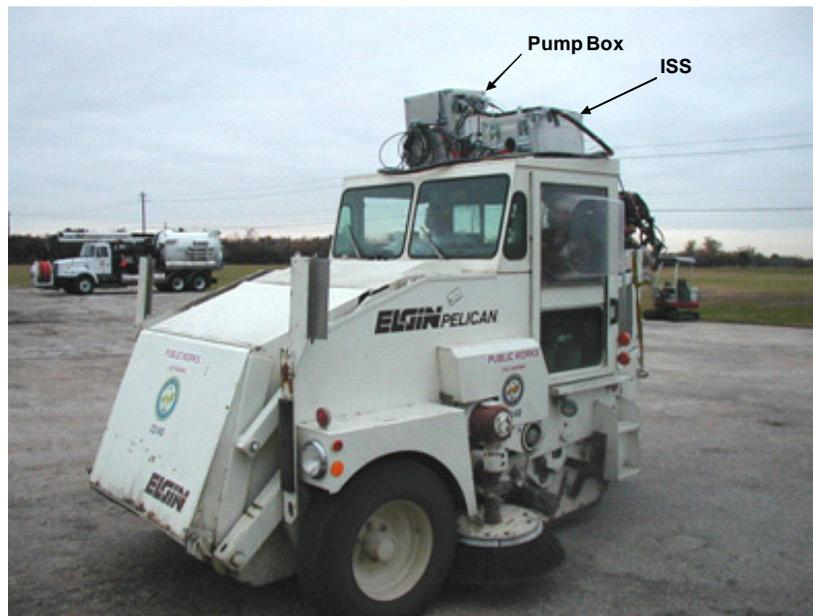
**Figure 6-3. Example ISS and Pump Box Installation on a Sweeper
