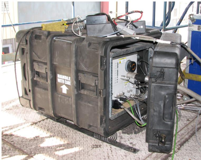
**Figure 6-1. Example PEMS Installation**
