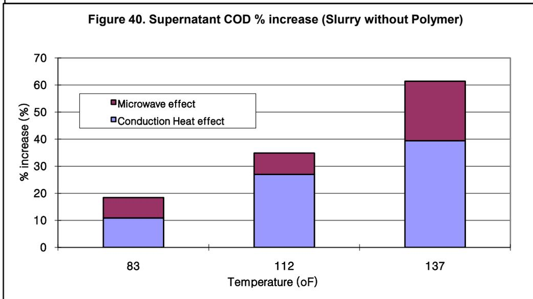
**Temperature Effects: Microwave vs Conduction Heating Dissolved COD - Slurry without Polymer:**
