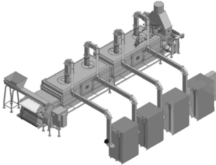
**Figure 52. Schematic Modular Conveyor Oven**
