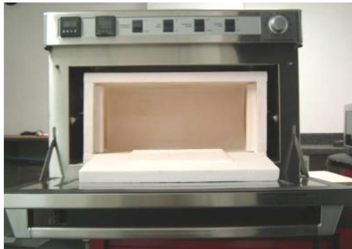
**Figure 2. Microwave 3.2 kW Multimodal Variable Power Applicator**
