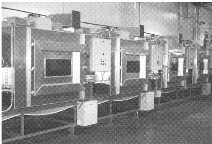
**Figure 51. Modular Conveyor Oven**
