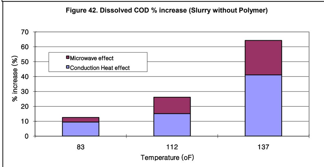
**Temperature Effects: Microwave vs Conduction Heating Dissolved Solids - Slurry without Polymer:**
