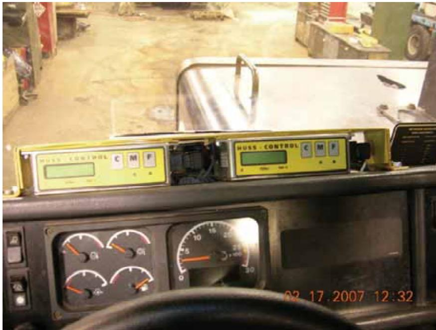
**Figure 3-10. In-Cab Display of Huss ADF Control Modules Installed in the CAT D400 Dump Truck**
