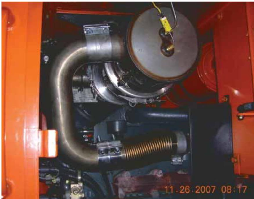
**Figure 3-12. Left-Side View of the ECS DPF Installed on a Case 821 Rubber Tire Loader**
