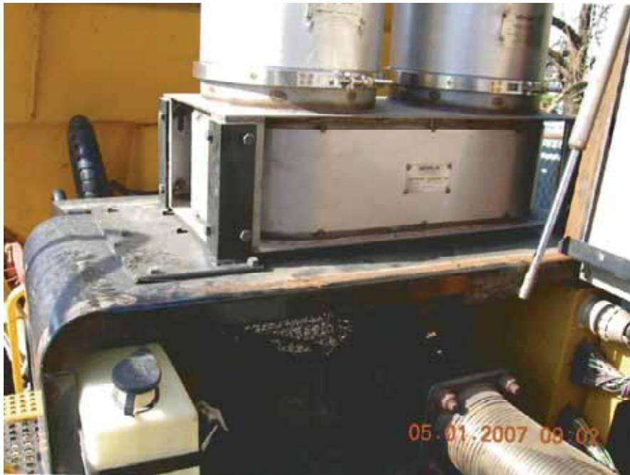
**Figure 3-8. Front View of the Johnson Matthey DPF Mounting Arrangement**
