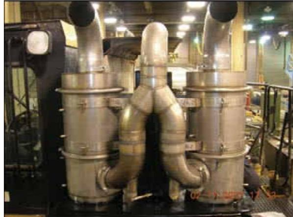
**Figure 3-9. Front (left) and Rear (right) View of the Huss ADF Dual Filter Retrofit Installed on a CAT D400 Dump Truck**
