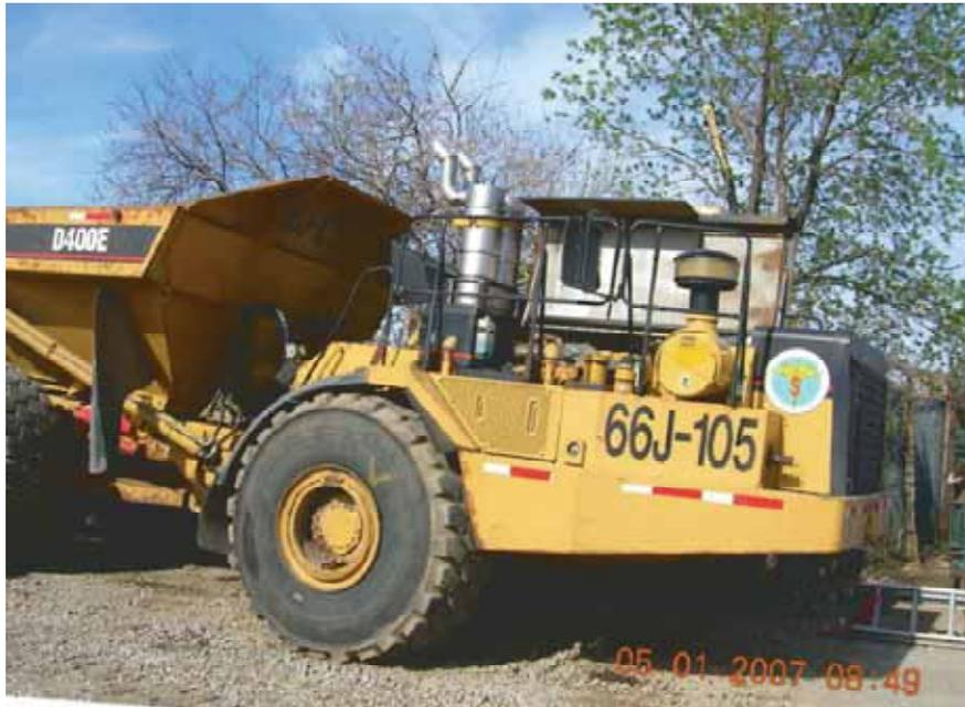
**Figure 3-7. Johnson-Matthey DPF installed on a CAT D400 Dump Truck**
