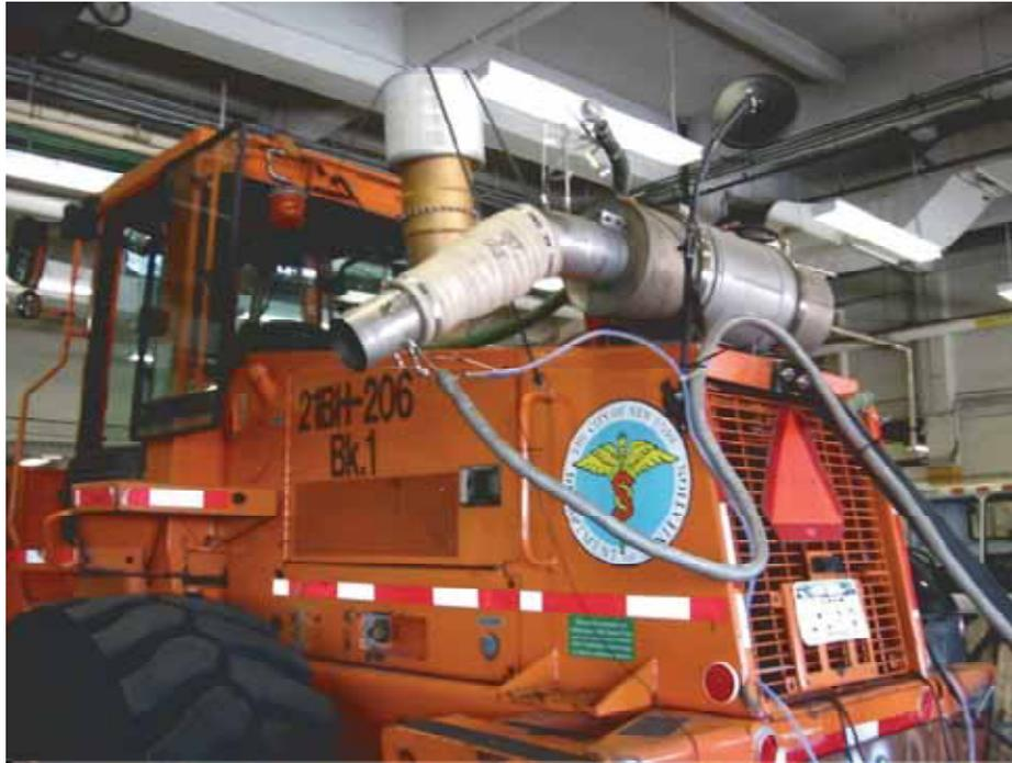
**Figure 3-11. CleanAIR Systems PDPF Installed on a Case 821 Rubber Tire Loader and Instrumented for In-Use Emissions Testing**
