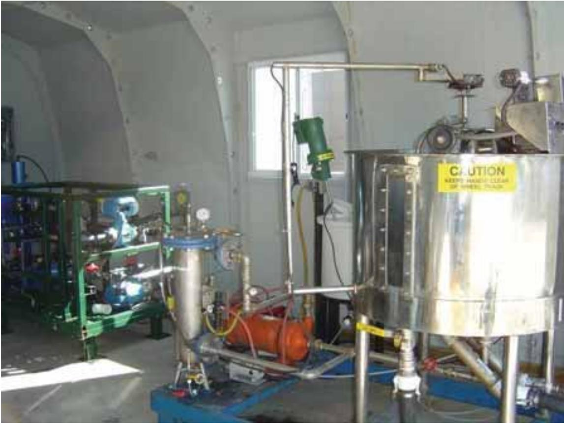
Figure 2-4. Recycled Flow Pressurization System – Krofta Supracell
