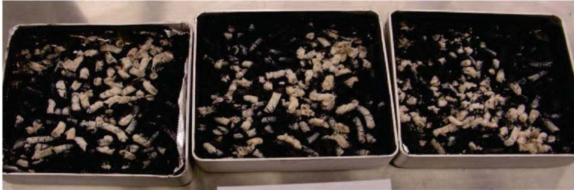
Figure 3-18. Final Char for Wood Pellets Sample.
