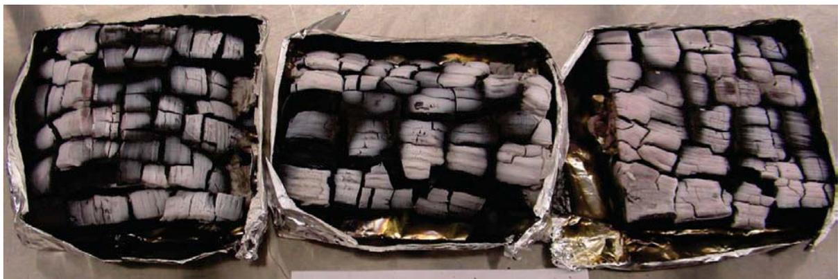
Figure 3-10. Final Char for Ash Wood Sample.
