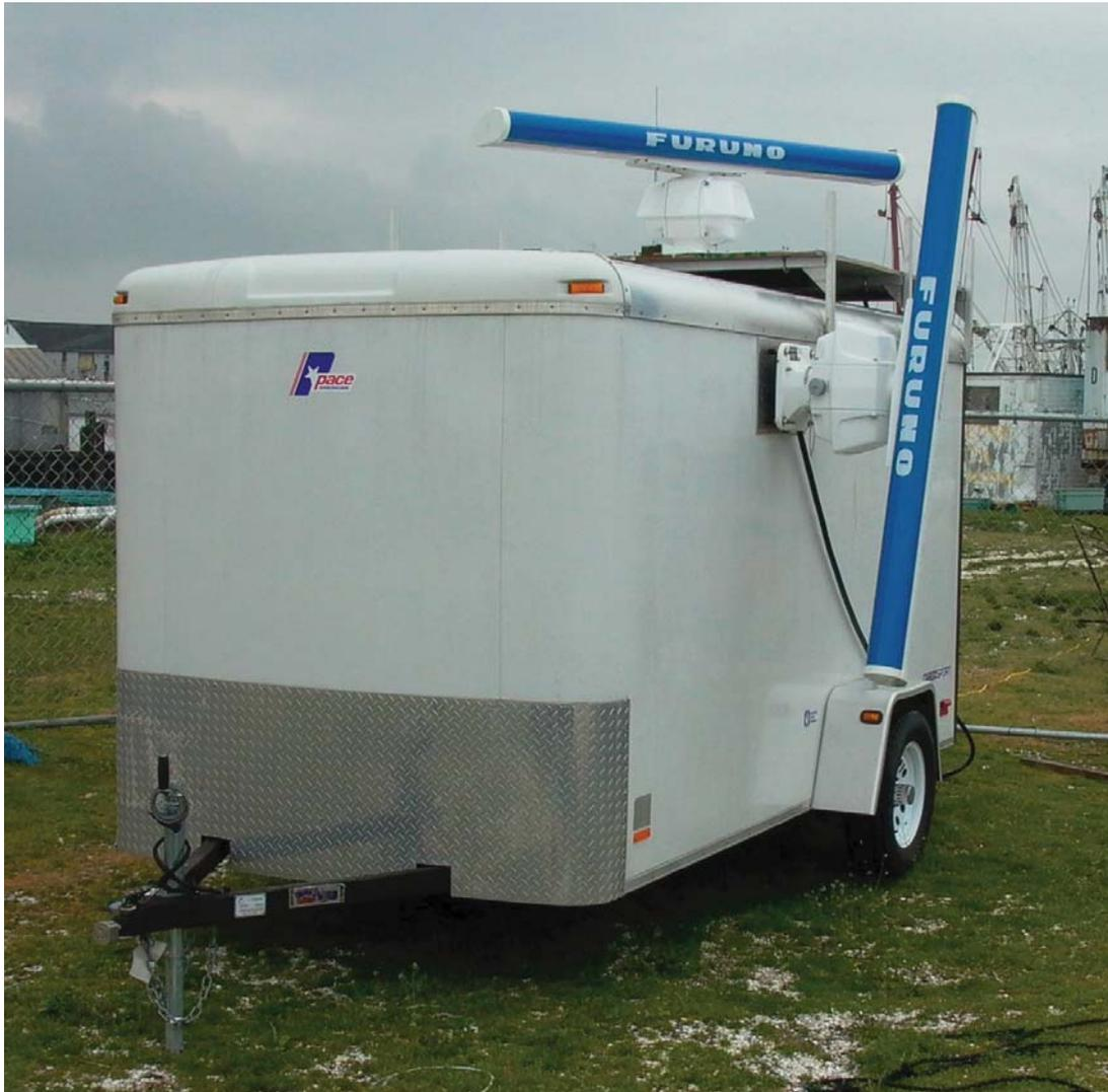
Figure 1. Dual radar system with horizontally and vertically oriented antennas that operate simultaneously. The system allows for data collection on passage magnitude (vertically-oriented radar), altitude (vertically-oriented radar) and flight direction (horizontally-oriented radar).
