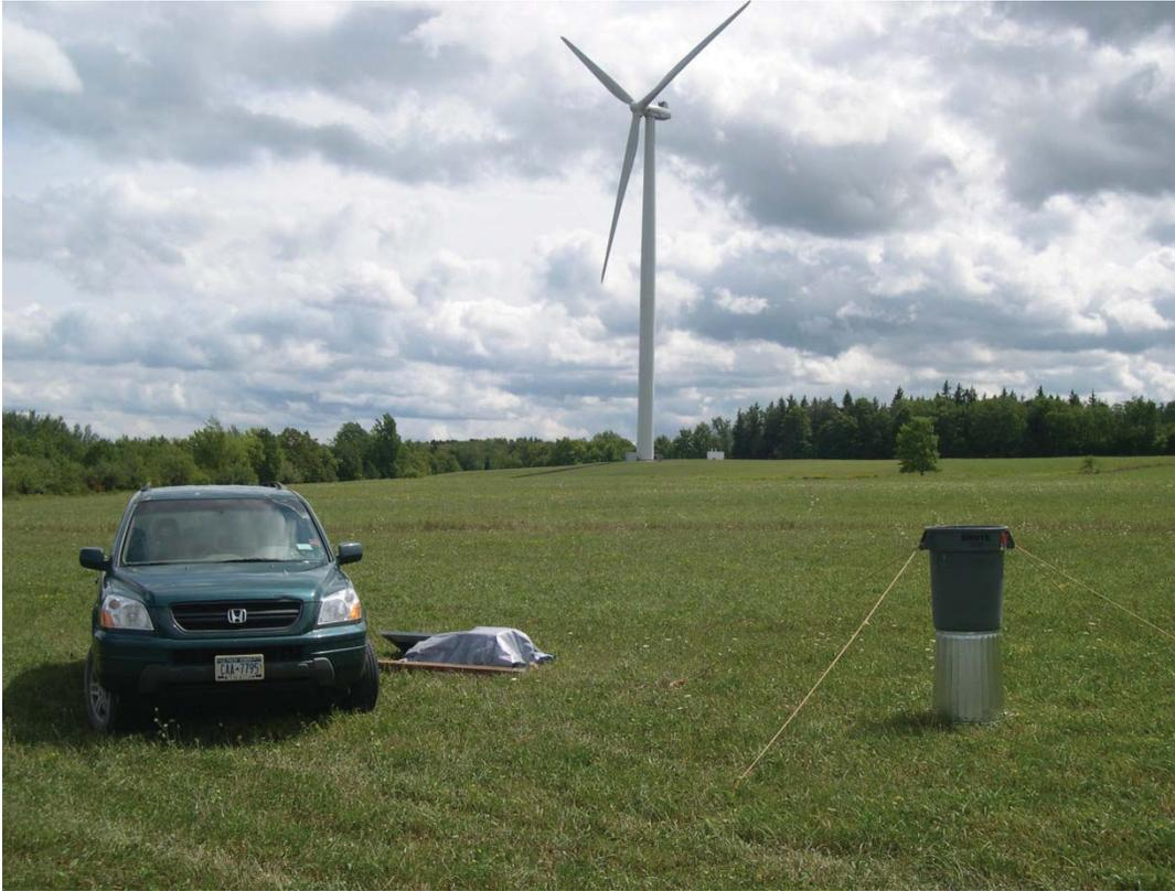
Figure 3. Avian acoustic recording station. Skyward-facing microphone is in gray cylinder. Recording gear and batteries are under plastic tarp.
