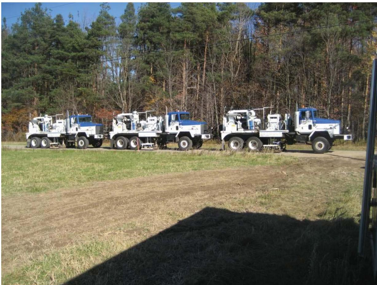
Figure 11: View of prospect area with vibrator trucks
