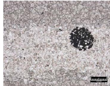
**Little Falls- 6356 ft.** Fine to medium grained, detrital quartz grains, are subrounded to rounded, with common quartz overgrowths on original grains. Common to minor dolomite cement, minor calcite cement, along with pyrite cement, are common pore reducers in this sample. Minor intergranular pores, and intracrystalline pores in dolomite.
