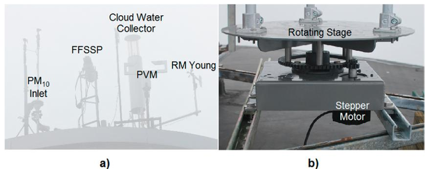
**Fig. 4.** Photographs of (a) instruments on the roof of the Silo building while sampling clouds during CPOC, as viewed from just outside the base of the Silo building on the upwind side, and (b) the base of the FFSSP tower on the roof of the Silo building, attached to a rotating stage, driven by a stepper motor.
