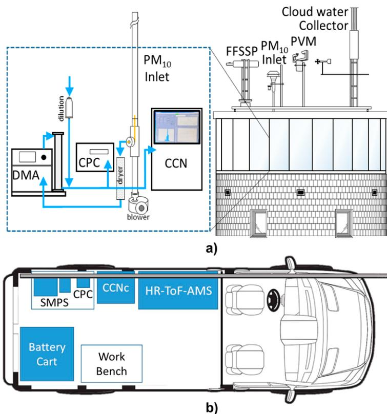
**Fig. 3.** (a) Instruments and inlets on the roof of the ASRC summit research observatory (also known as the Silo building) and housed within the top floor of the Silo building during the CPOC pilot study. (b) Instruments housed within the ASRC Sprinter van.
