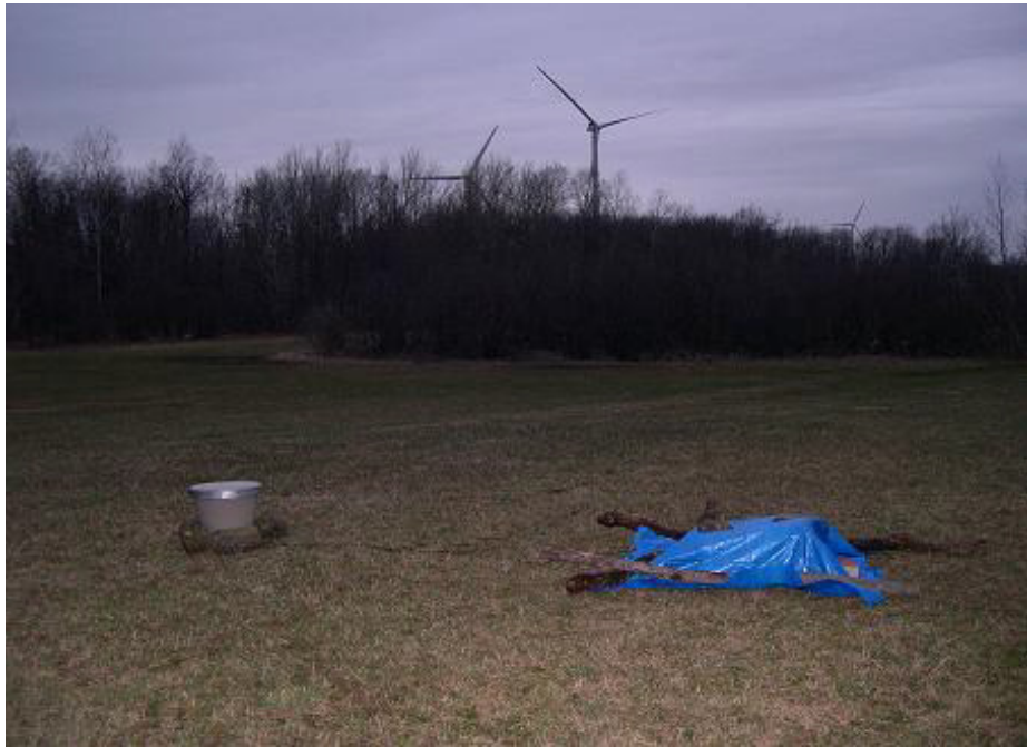
Figure 4c. “Spring 2007” acoustic station. Microphone is tan “flowerpot” container on left. Recording gear and batteries are under tarp. Lat 43.715287, Long -75.557485
