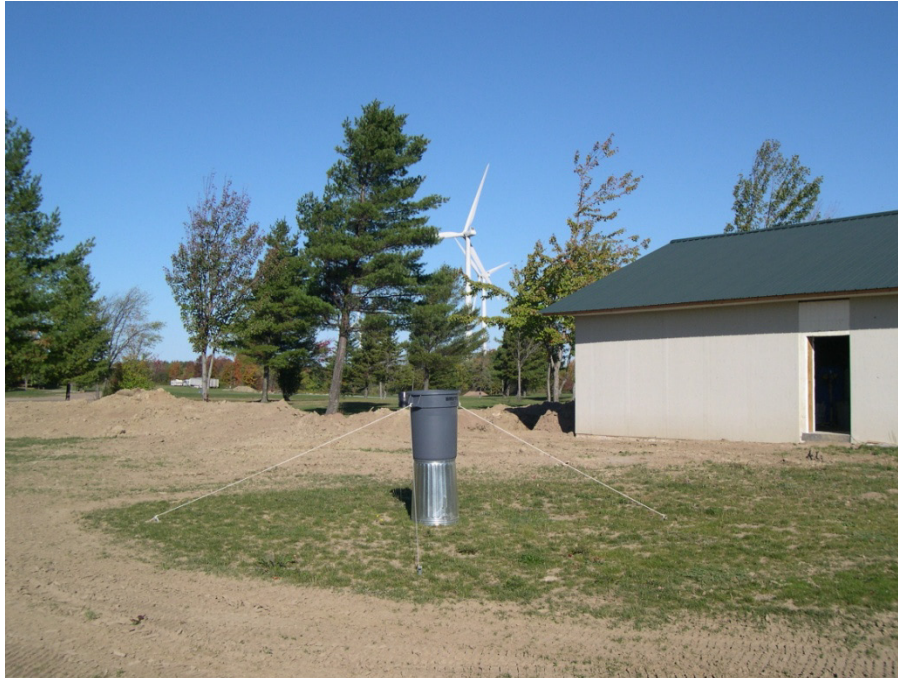
Figure 4b. “Flatrock” acoustic station. Skyward-facing microphone is in gray cylinder. Recording gear is in adjacent building. Lat 43.732623, Long -75.56581
