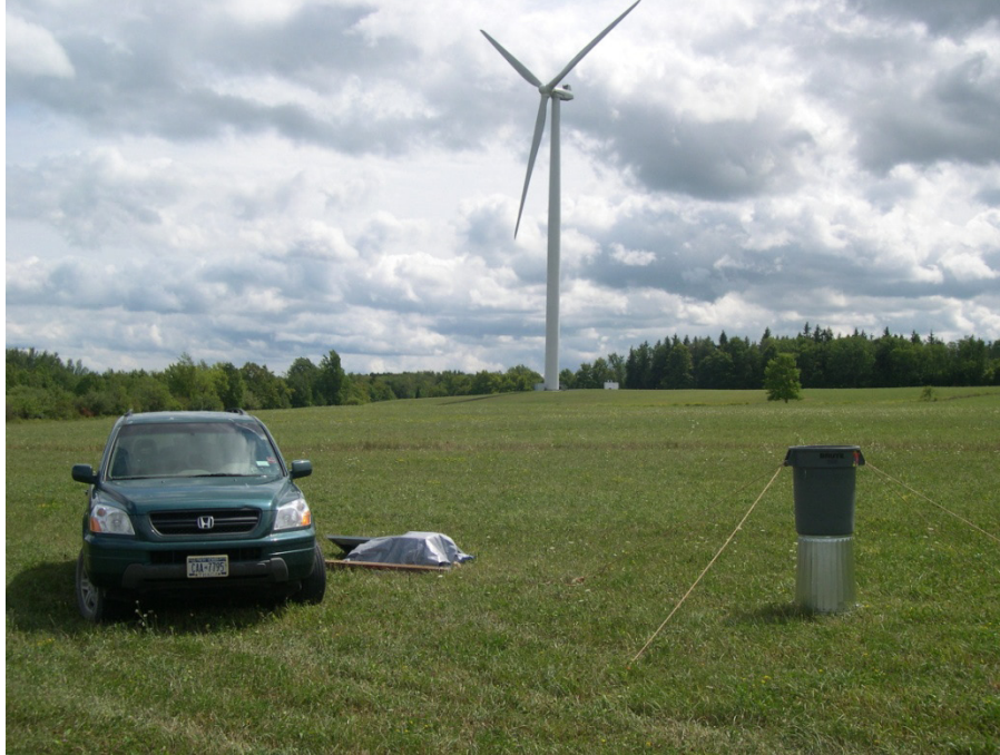
Figure 4a. “Radar” acoustic station. Skyward-facing microphone is in gray cylinder. Recording gear and batteries are under plastic tarp. The white New Jersey Audubon radar trailer can be seen just to the right of the base of the wind turbine. Lat 43.714767, Long -75.505257
