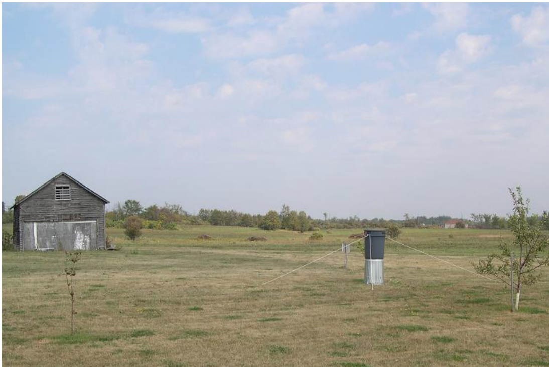
Figure 4d. “CVP-n” acoustic station on the Cape Vincent Peninsula in northern New York. Skyward-facing microphone is in gray cylinder. Lat 44.143564, Long -76.206056
