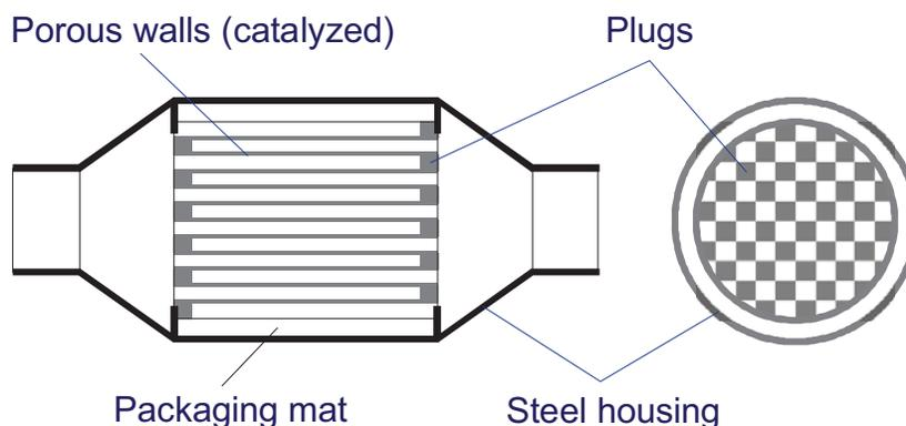
**Figure 4-1. Catalyzed Diesel Particulate Filter**
