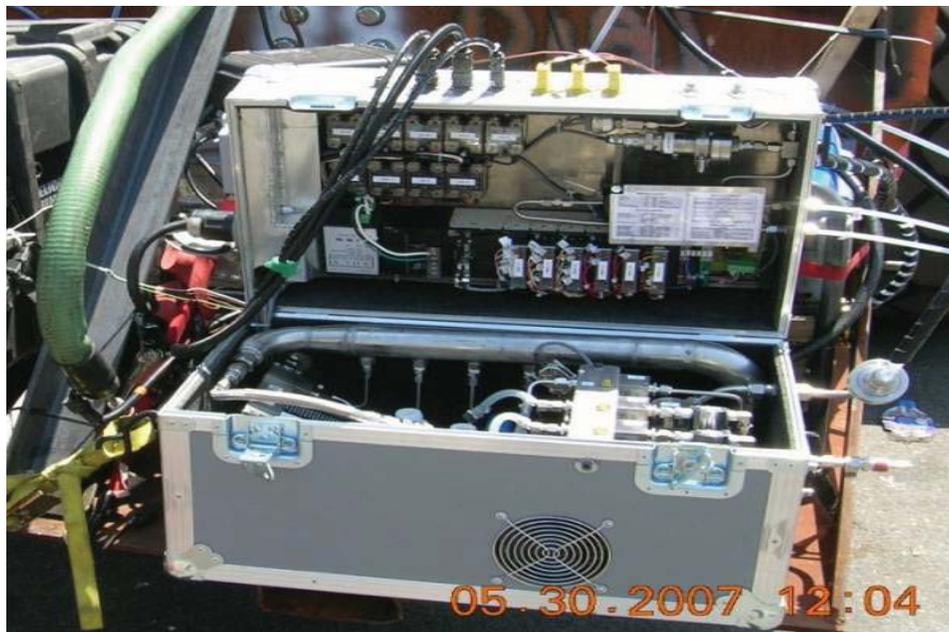
The Ride-Along Vehicle Emissions Measurement (RAVEM) system is capable of measuring PM as well as NO<sub>x</sub>, CO, and CO<sub>2</sub>. Optional capabilities also allow the measurement and quantification of total hydrocarbons (THC), sulfur dioxide (SO<sub>2</sub>), ammonia (NH<sub>3</sub>), and nitrous oxide (N<sub>2</sub>O), as well as individual species of volatile organic compounds (VOC) and carbonyls such as formaldehyde, acetaldehyde, and acrolein.
