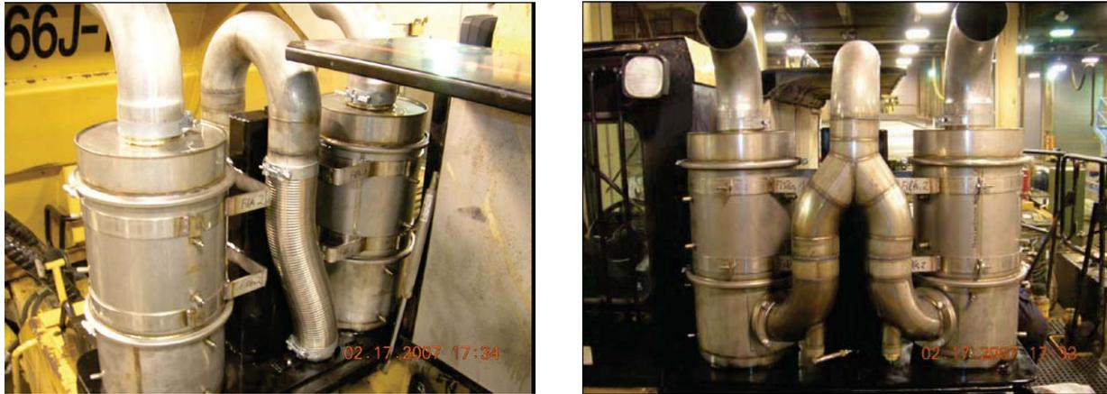
**Figure 4-15. Front (left) and Rear (right) View of the Huss ADFP Dual Filter Retrofit Installed on a CAT D400 Dump Truck**
