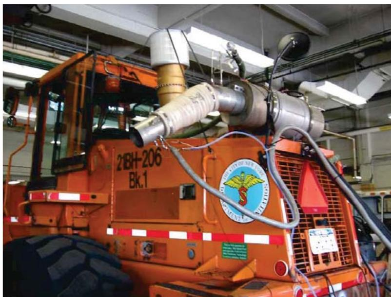
**Figure 4-3. CleanAIR Systems PDPF Installed on a Case 821 Rubber Tire Loader and Instrumented for In-Use Emissions Testing**
