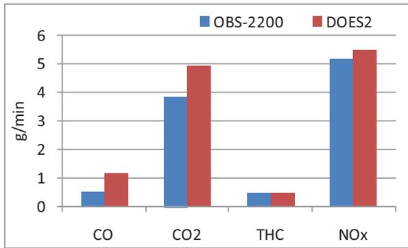
**Figure 4-23: Pre-CleanAIR PDPF Emissions Results from the OBS-2200 and the DOES2**
