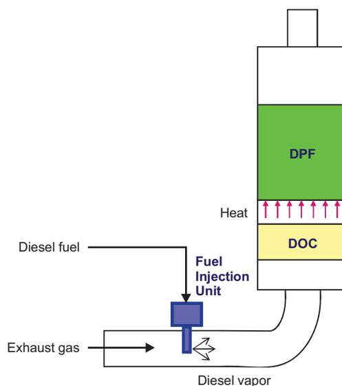
**Figure 4-12. Filter with Catalytic Combustion of Fuel**
