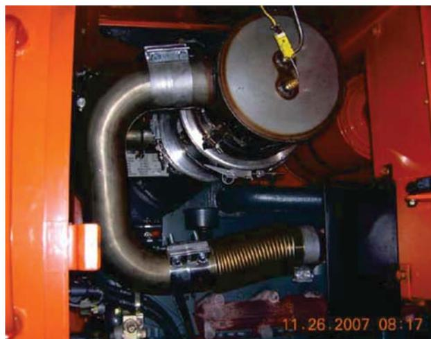
**Figure 4-5. Left-Side View of the ECS DPF Installed on a Case 821 Rubber Tire Loader**
