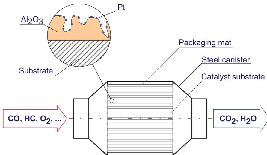
**Figure 4-22. Schematic of Diesel Oxidation Catalyst**
