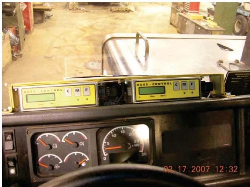
**Figure 4-16. In-Cab Display of Huss ADFP Control Modules Installed in the CAT D400 Dump Truck**
