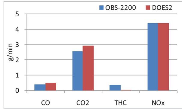
**Figure 4-26: Post-AirMeex ADPF Emissions Results from the OBS-2200 and the DOES2**
