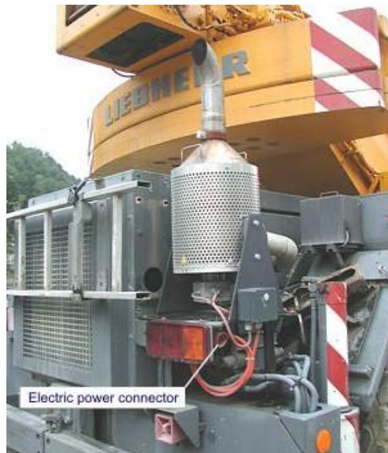
**Figure 4-7. Shore Power Regenerated Filter on Construction Machinery (Switzerland)**
