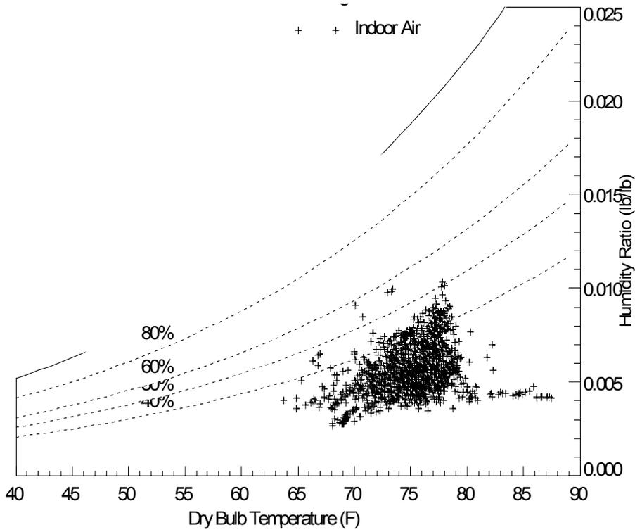
**Figure 77. Daily Conditions Shown on the Psychrometric Chart during Cooling at R-House**
