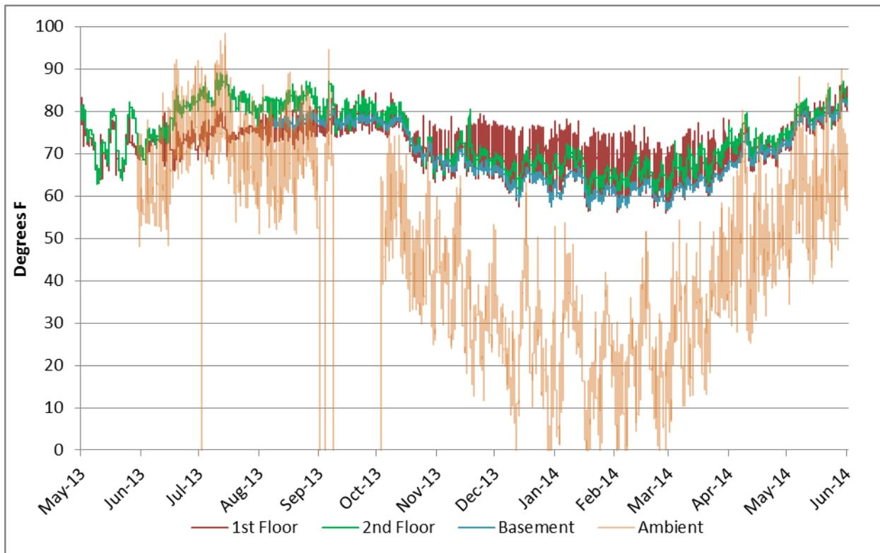
In Townhome B, the heat pump was operating 36% of the time over the period from Aug 14, 2013 to June 9, 2014 when heat pump data was logged. Tables 23, 24, and 25 show the amount of time that indoor temperatures were out of normal comfort range, as a percent of time that the heat pump was on and as a percentage of total monitoring time.
