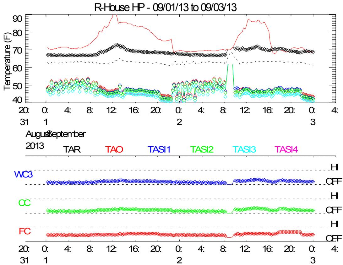
Figure 63. Heat Pump Performance for a Typical Cooling Day at R-House
