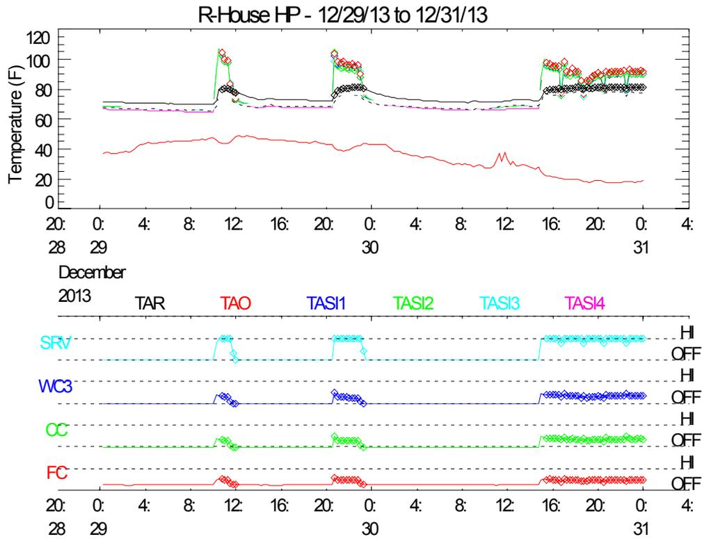
Figure 67. Heat Pump Operation Trends during Defrosting at R-House
