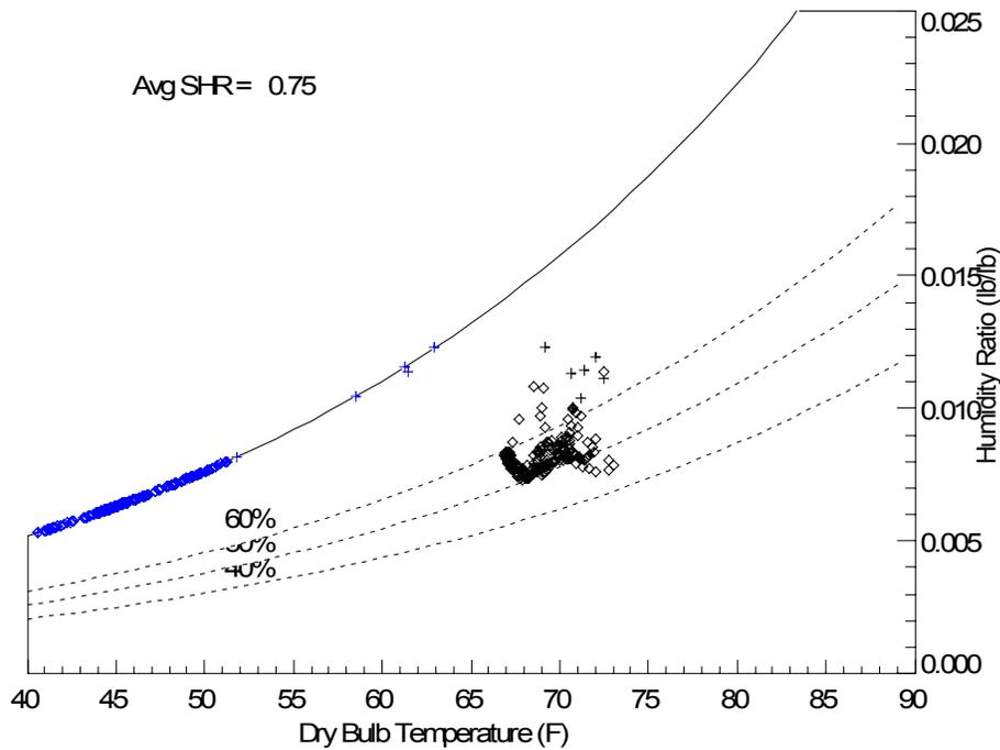
**Figure 65. Room Sensible Heat Ratio (SHR) for a Typical Cooling Day at R-House**
