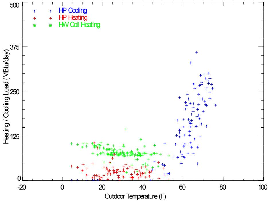
Figure 71. Total Heating and Cooling Loads vs. Outdoor Temperature (R-House)
