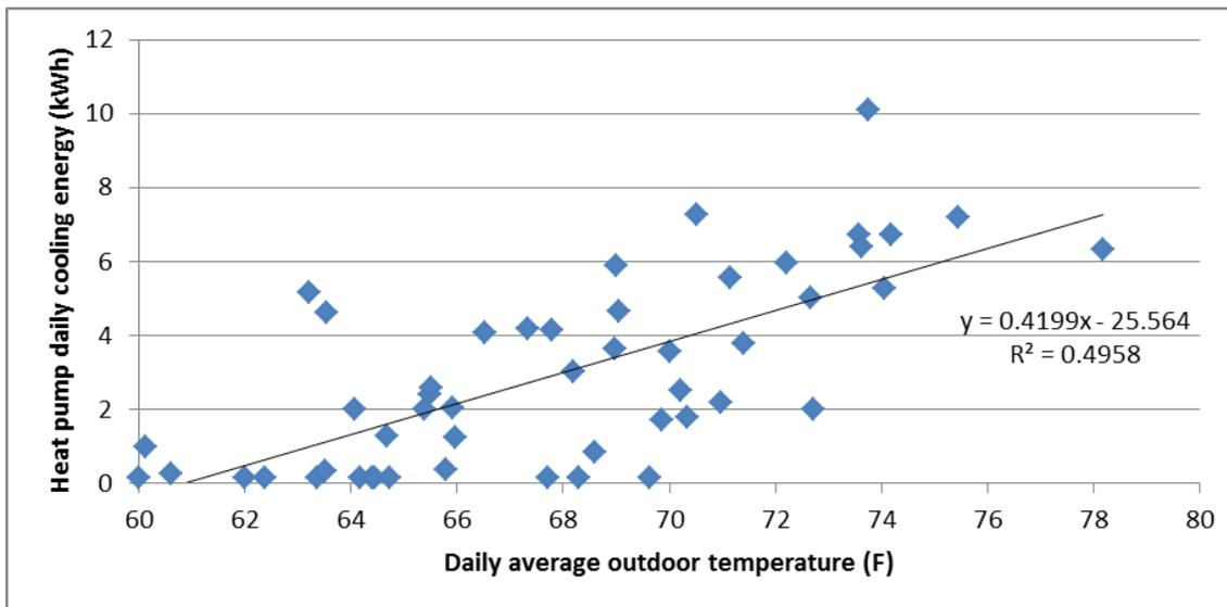
The maximum power draw of these units is approximately 2 kW. Because of the on-off nature of the heat pump operation, the heat pump was often operating at its maximum output, despite the fact that the unit was oversized relative to the home's calculated load at design temperature.
