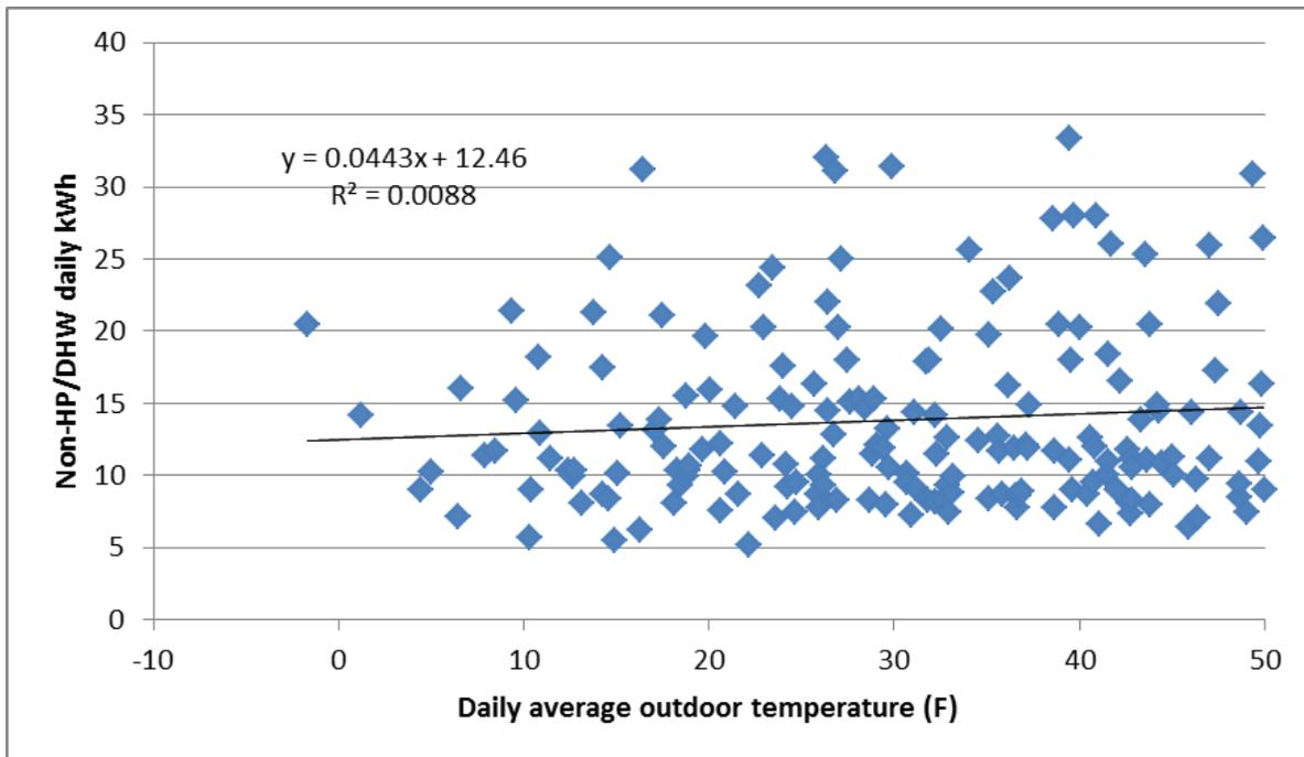
Comparison of non-HP/DHW energy for Townhome A during the 2013 and 2014 cooling seasons shows an increase from about 14 kWh per day to 17 kWh per day (Figure 43). Part of this increase could be due to the addition of the three floor transfer fans at 25 watts each and the reported increase in occupancy of the home.
