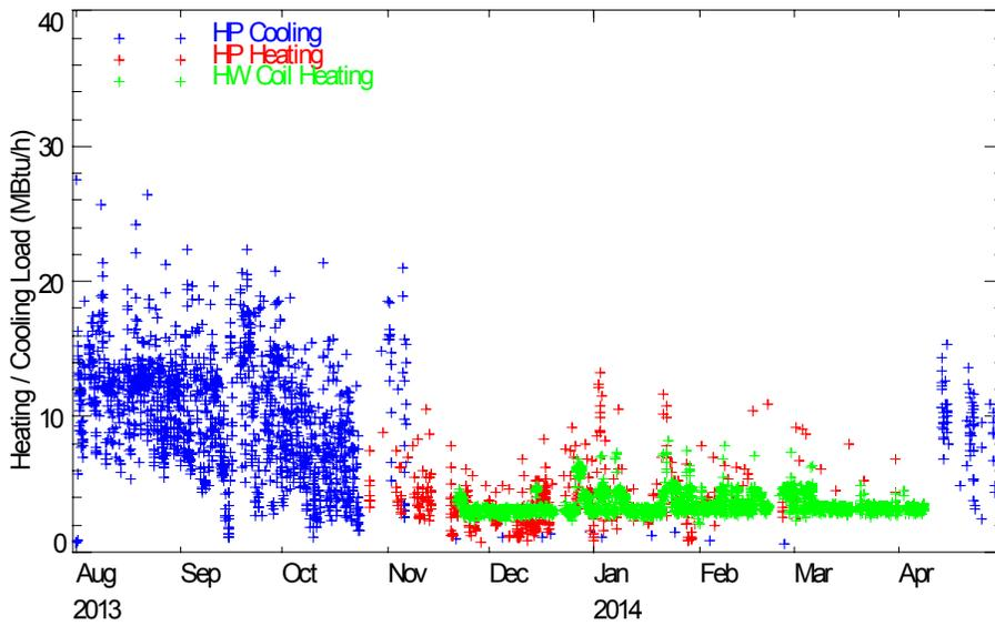
Figure 70 and Figure 71 shows the trend of measured space heating and cooling loads with ambient temperature on a daily basis, a trend often referred to as the heating load line. The figures show that except for a very low outdoor temperature (i.e., outdoor temperature less than 20°F), the heating load was nearly constant and independent of the outdoor temperature while there was a sharp increment in cooling load with a small increment in outdoor temperature.
