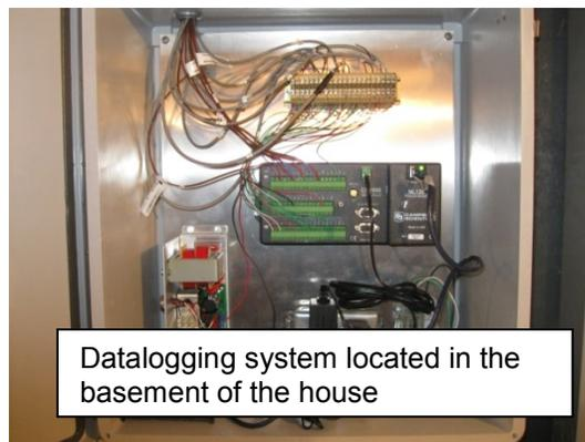
**Figure 60. Flow Test Setup for the MSHP and Various Sensors to Monitor MSHP Performance at R-House**
