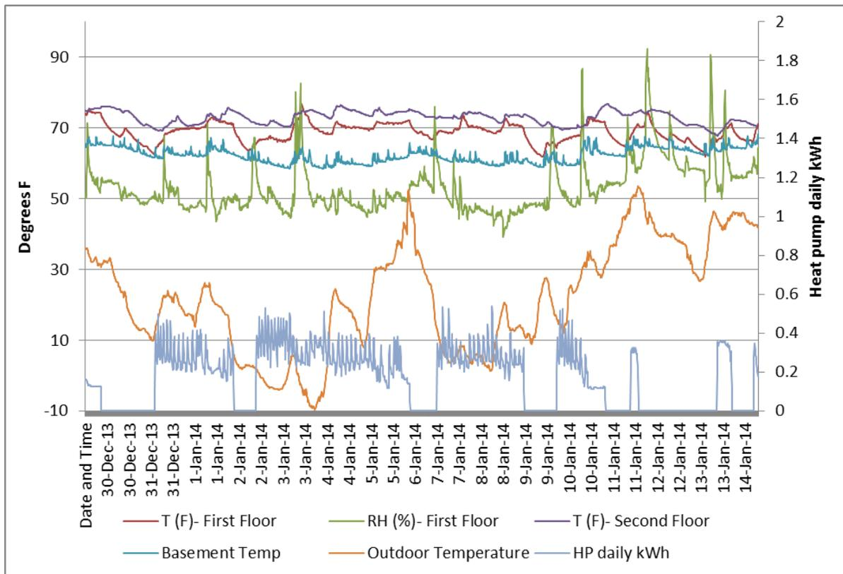
The Townhome A data show that the first floor temperatures were controlled closer to the desired setpoint than the second floor temperatures, which were warmer in summertime and slower to react to the activation of the heat pump in wintertime.
