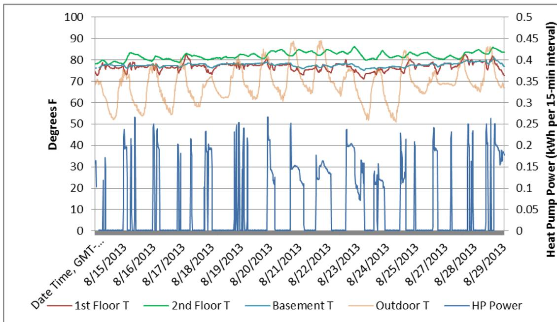
During the summer cooling season, this sample data showed that the heat pump in Townhome B was operated less frequently. First-floor temperatures were generally in the mid-to-high-70s when the heat pump was on. Second-floor temperatures reached into the low 80s with the heat pump on during the hottest weather. Interestingly, the basement temperature was generally between the first and second floor temperature during this period (Figure 52).
