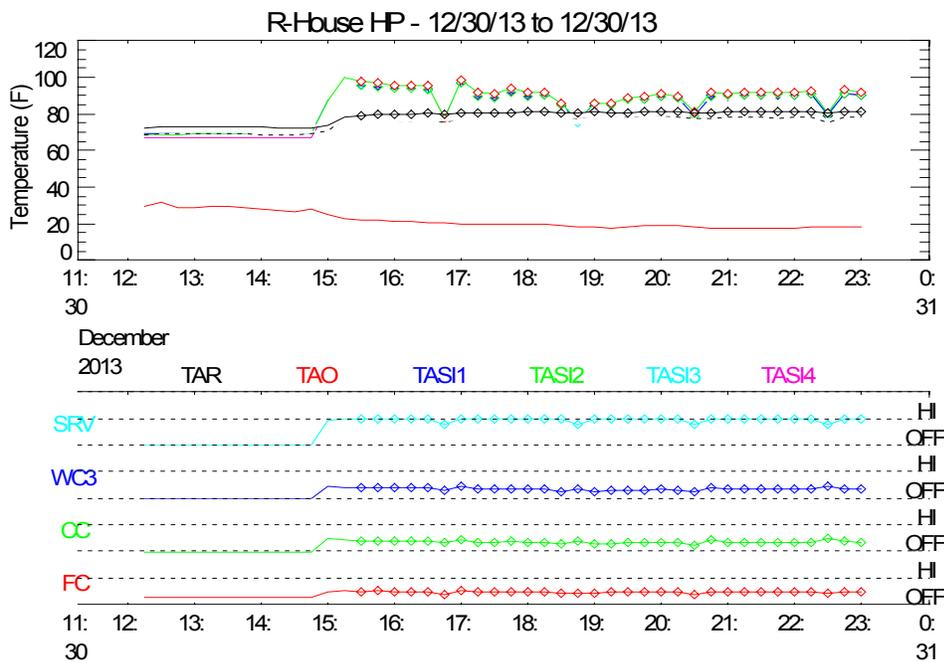
**Figure 68. Heat Pump Performance for a Typical Heating Day at R-House**
