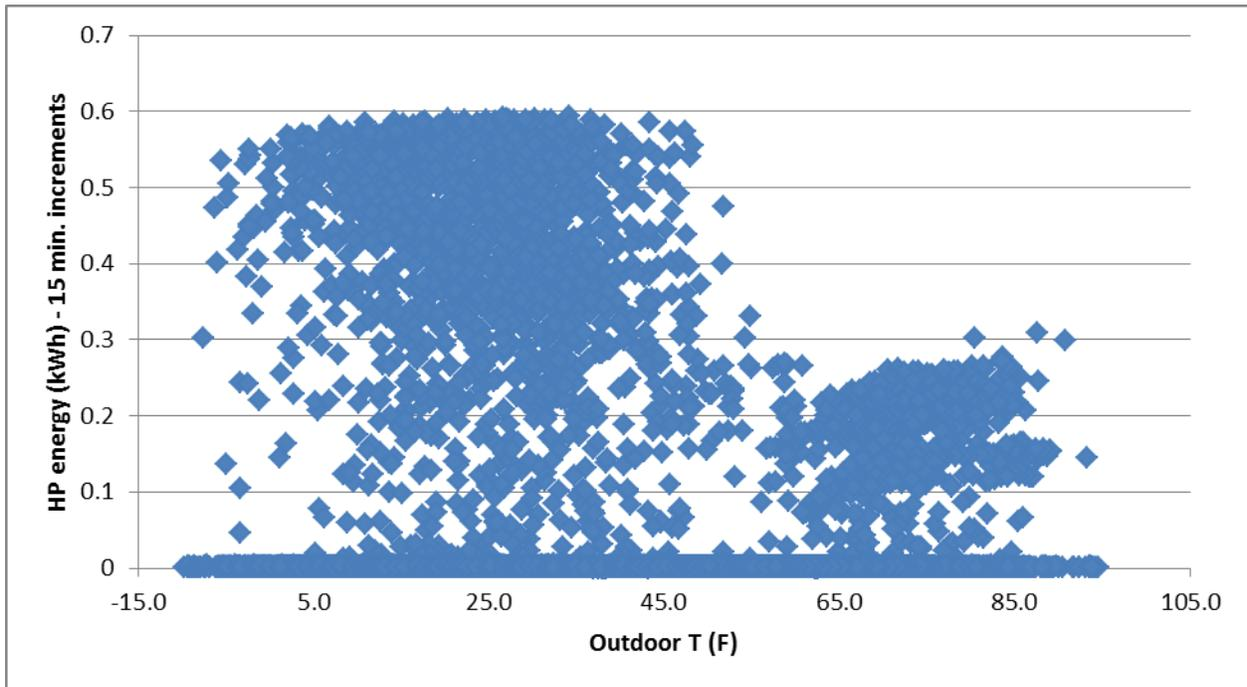
Figure 38. Heat Pump Power as a Function of Outdoor Temperature for Townhome B
