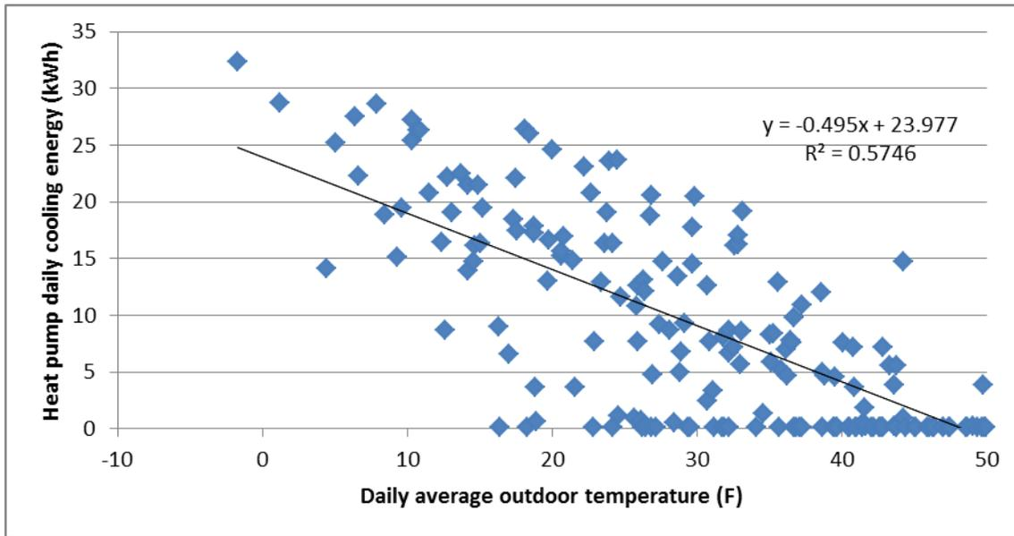
Figure 36. Cooling Load Line at Townhome B
