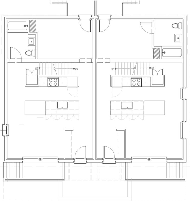
**Figure 30. Hudson Passive Townhomes Second Floor Plan**
