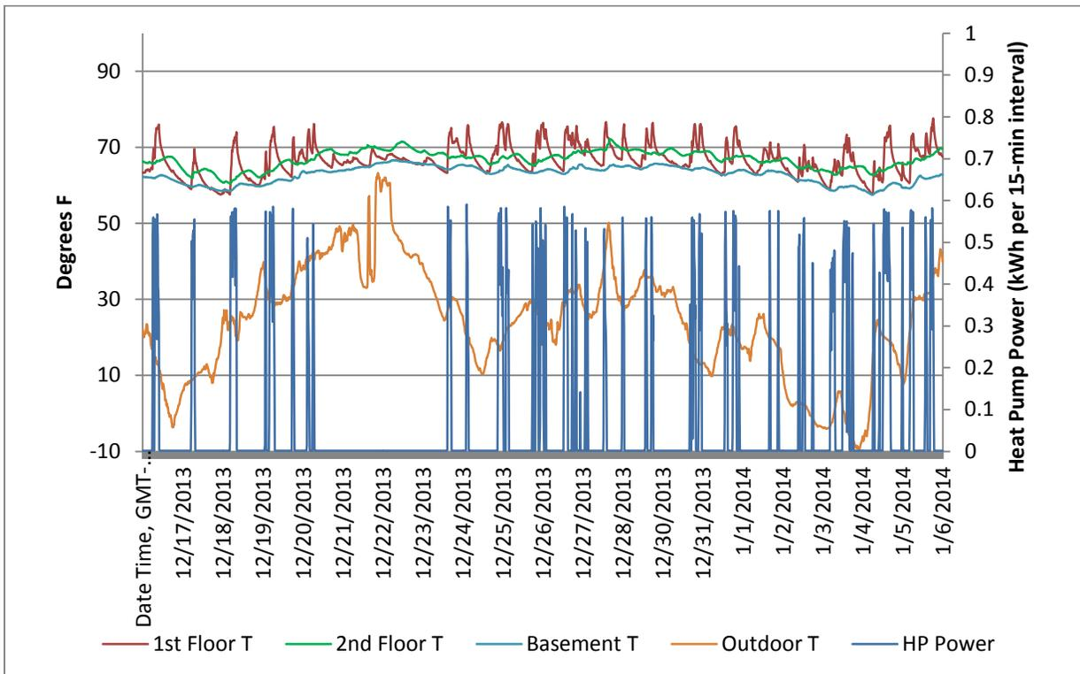
**Figure 50. Sample Heating Season Temperatures and Heat Pump Operation for Townhome B**
