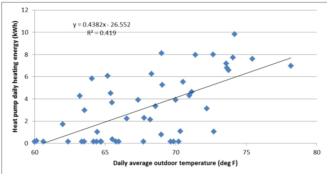
Figure 35. Heating Load Line at Townhome B
