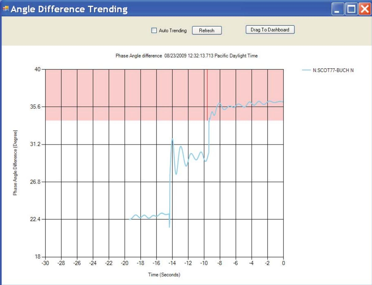
Figure 17 Trending Chart of Angle Difference between N. SCOT77 and BUCH N Substations
