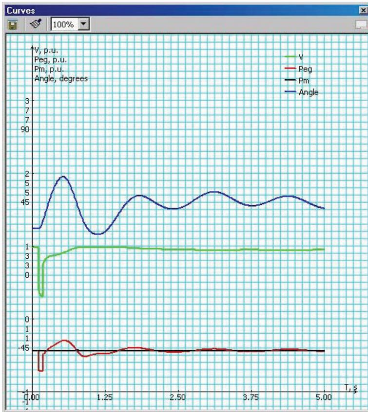
**Figure 5-6. Fault at Bus # [redacted] Clears in 0.08 sec**
