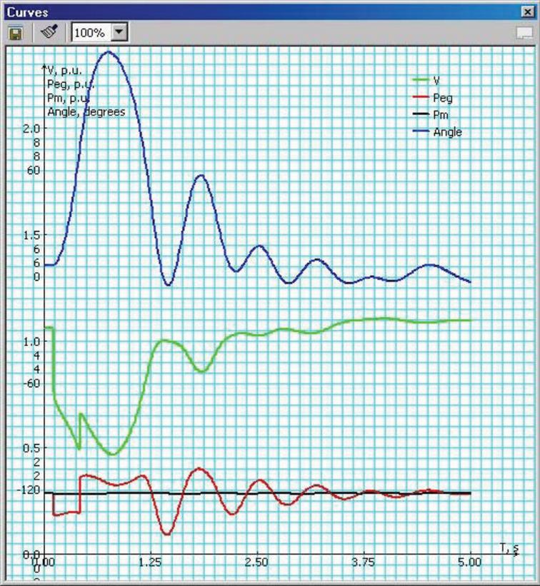
**Figure 5-11. Fault at Bus # [redacted] Clears in 0.27 sec**
