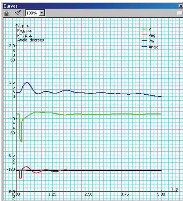
**Figure 5-10. Fault at Bus # [redacted] Clears in 0.08 sec**
