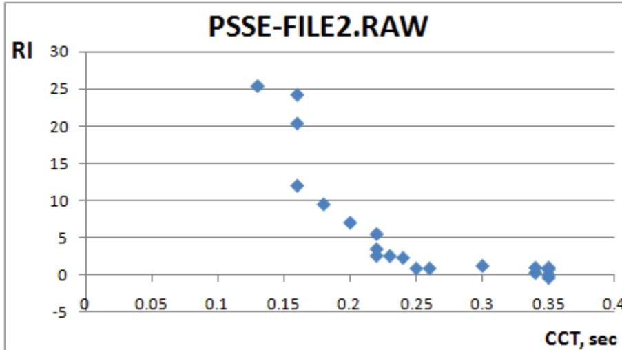
**Figure 6-28. Distribution of the Ranking Index by the Critical Clearing Time for Case “PSSE-FILE2.RAW”**
