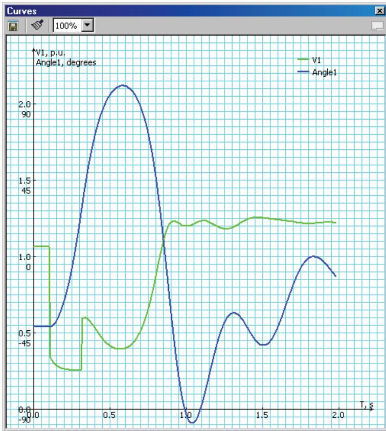
**Figure 6-26. Fault at Bus # 138.0 Clears in 0.20 sec**
