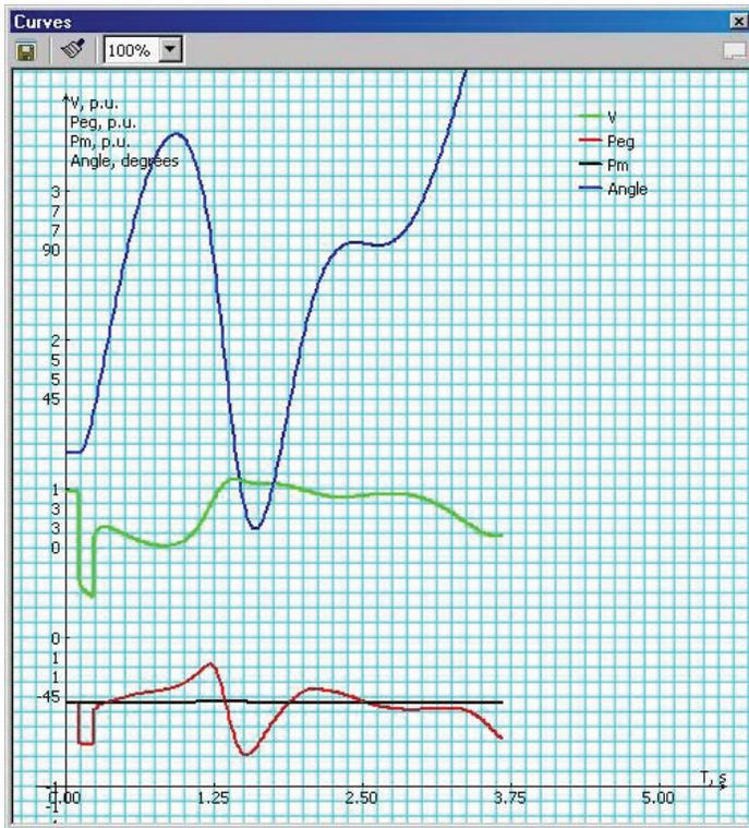
**Figure 5-8. Fault at Bus # [redacted] Clears in 0.13 sec**
