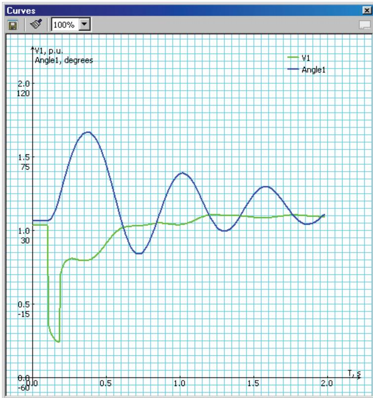
**Figure 6-20. Fault at Bus # 115.0 Clears in 0.08 sec**
