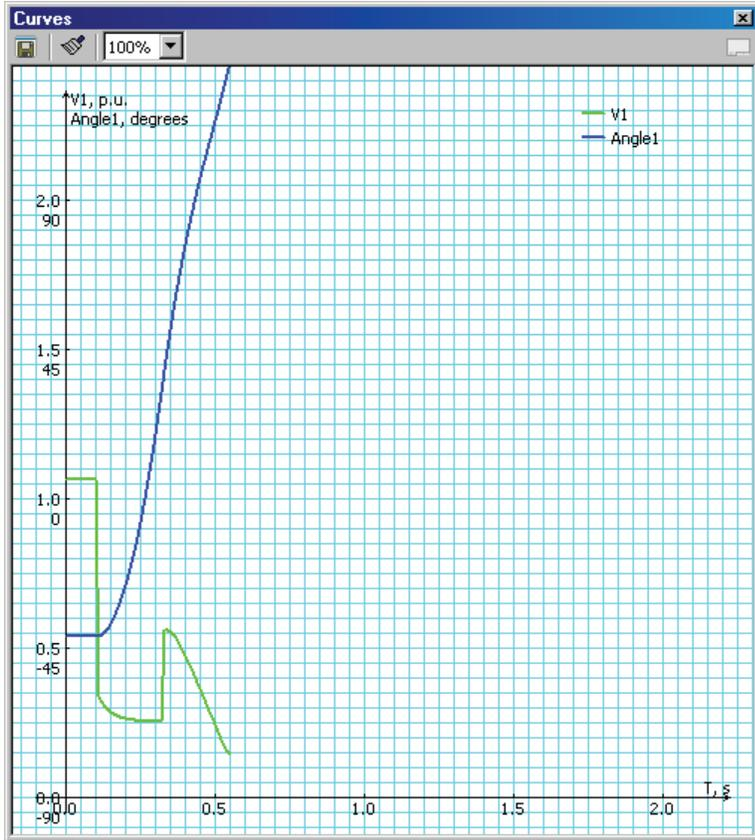
**Figure 6-27. Fault at Bus # 138.0 Clears in 0.21 sec**
