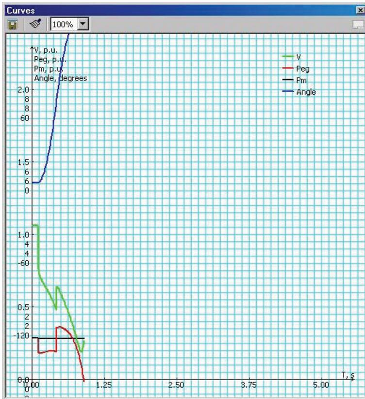
**Figure 5-12. Fault at Bus # [redacted] Clears in 0.28 sec**
