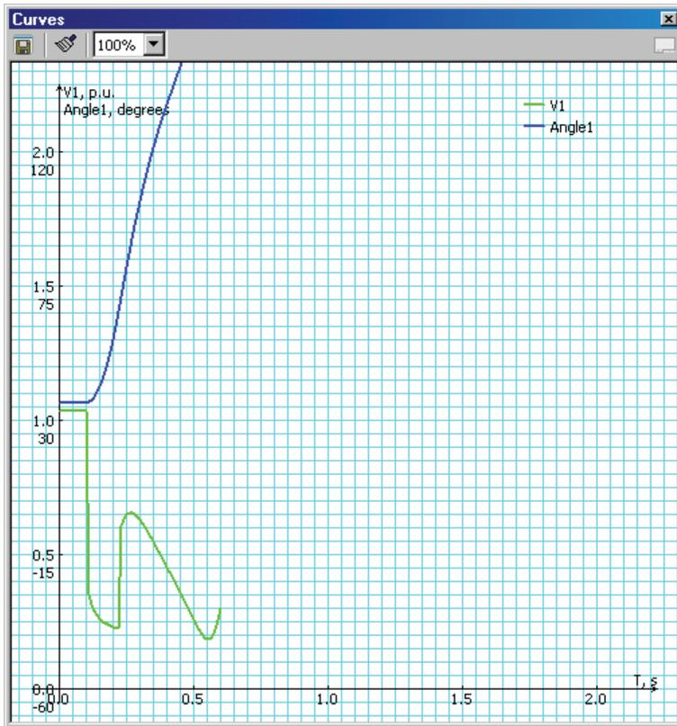
Figure 6-22. Fault at Bus # [redacted] 115.0 Clears in 0.13 sec
