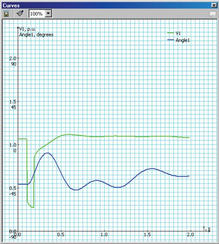
Figure 6-25. Fault at Bus # 138.0 Clears in 0.08 sec
