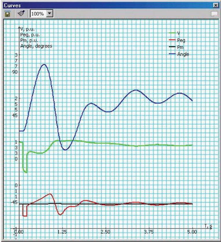
**Figure 5-7. Fault at Bus # [redacted] Clears in 0.12 sec**
