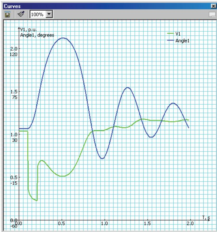
**Figure 6-21. Fault at Bus # 115.0 Clears in 0.12 sec**
