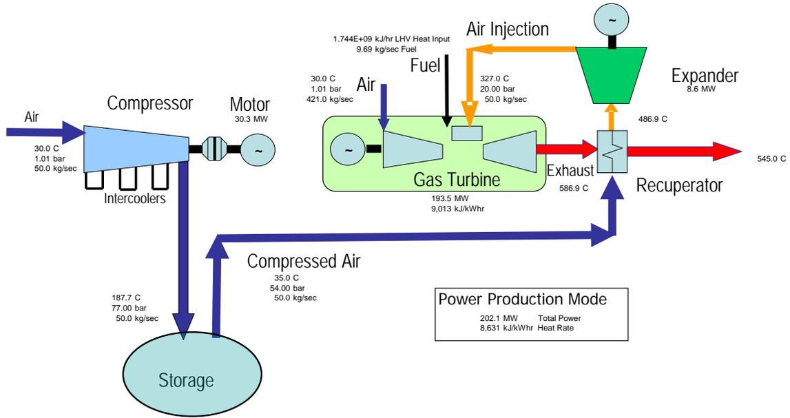
**Figure 25: Schematic and Heat and Mass Balance for the CAES-AI/HP Expander Plant Option**
