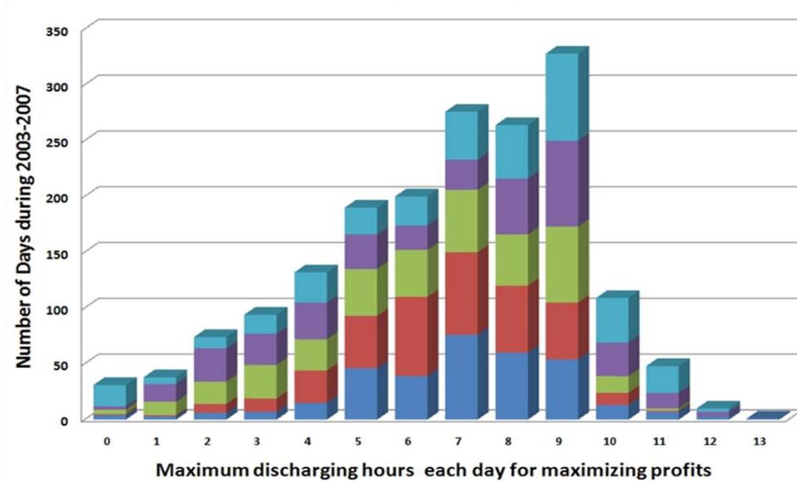
Figure 19: Anticipated operating hours for CAES unit with power ratio of 1.0 during 2003–2007
