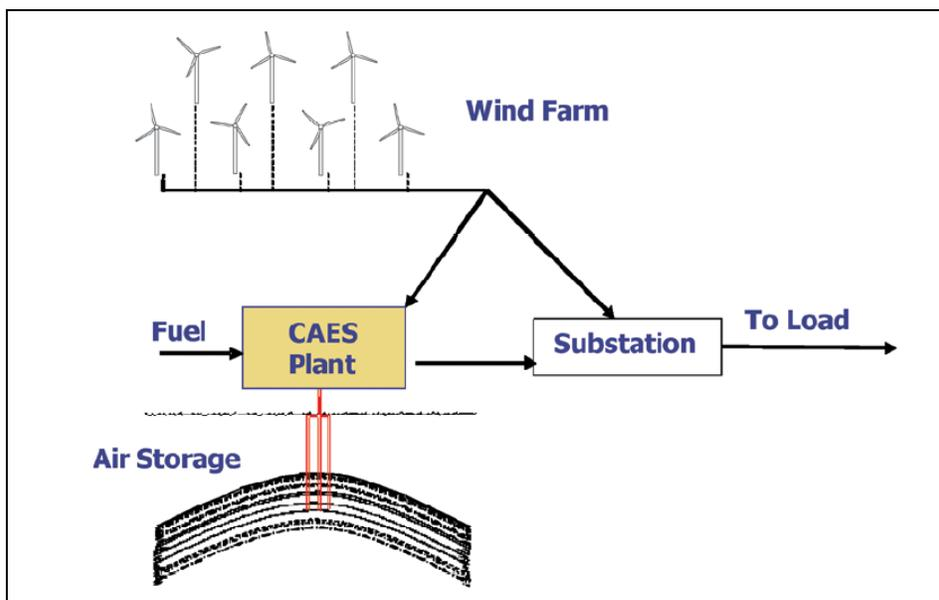
Figure 17: Schematic of a CAES System (Denholm)
