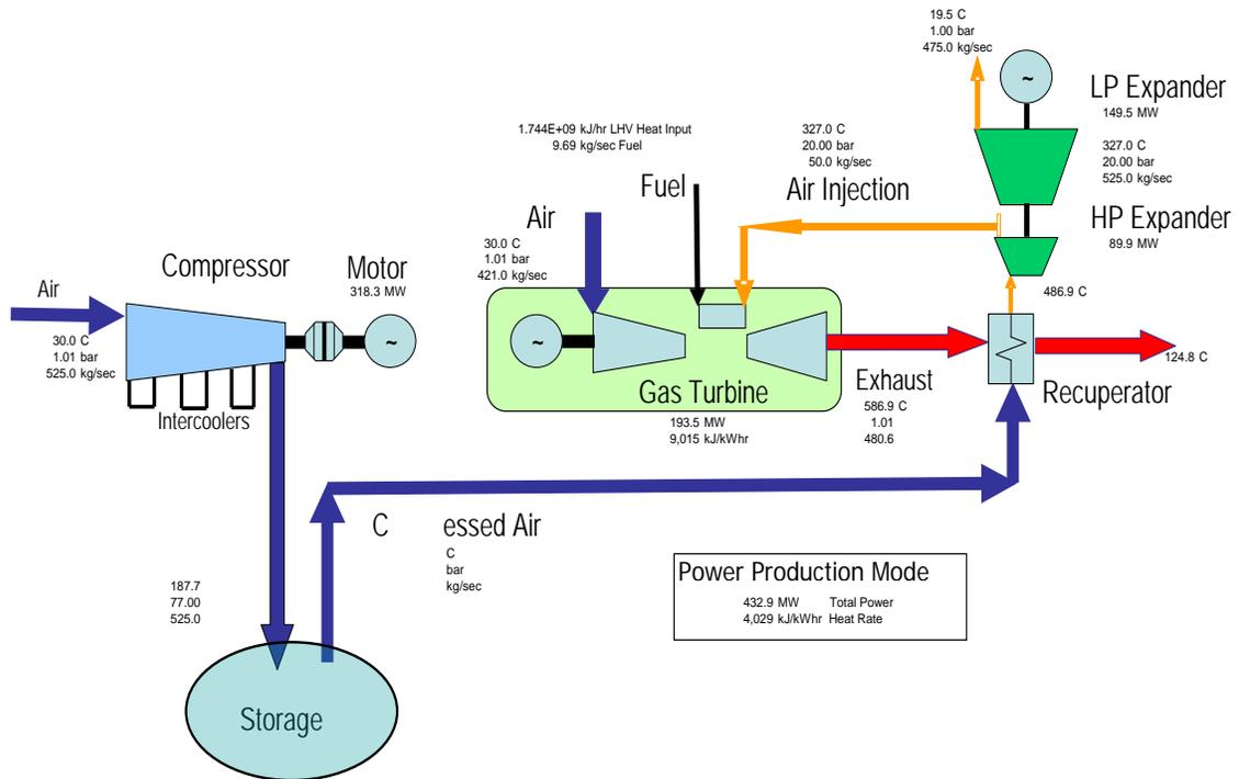
**Figure 16: Schematic and Heat and Mass Balance for the CAES-AI/Expander Concept**
