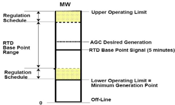
**Figure 18: Generating Unit Operating Characteristics for regulation service. Source: NYISO**
