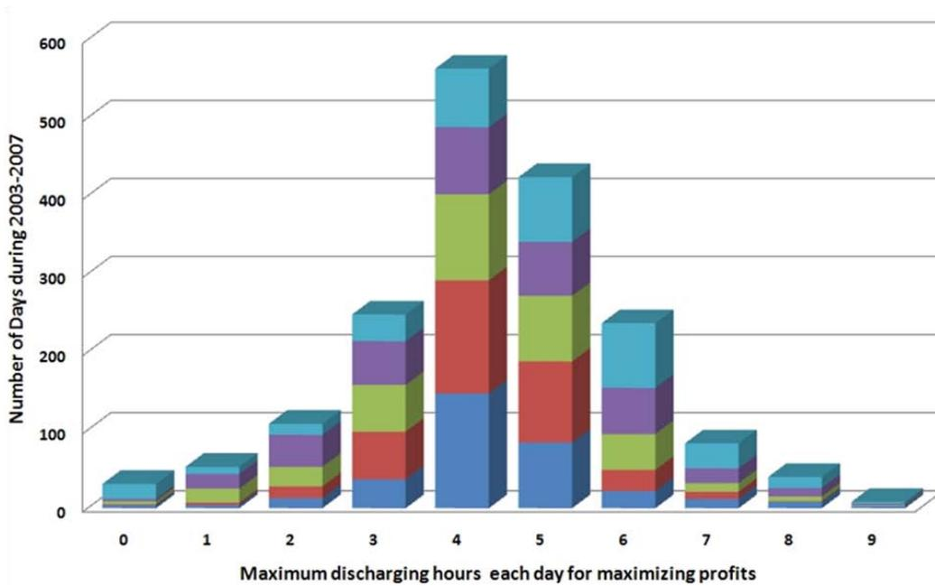
**Figure 36: Anticipated operating hours for CAES unit with power ratio of 0.5 during 2003–2007**
