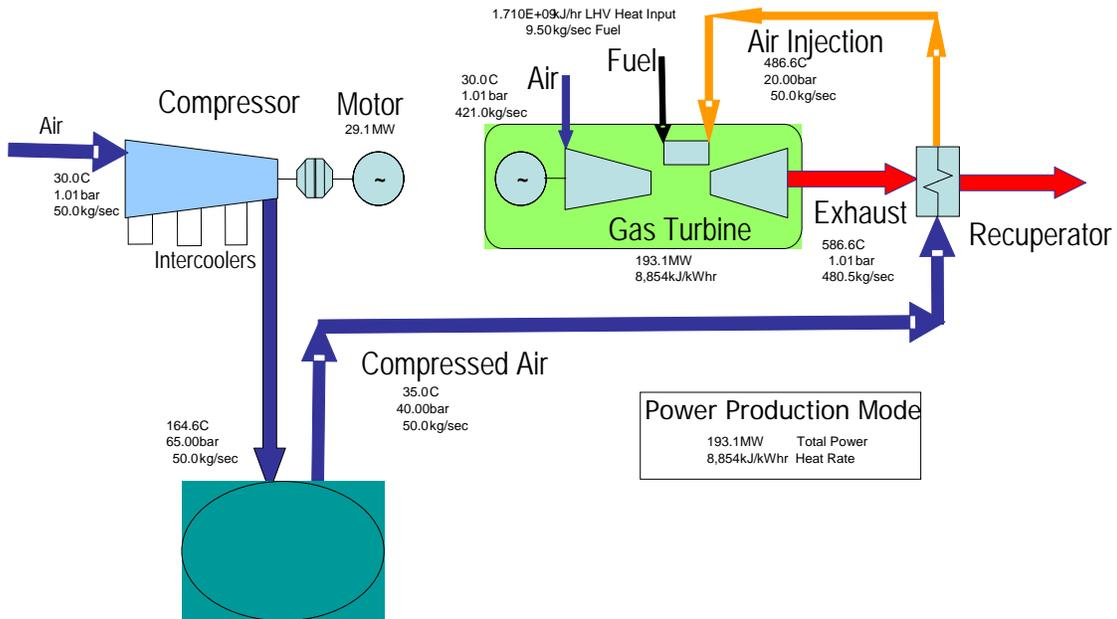
Figure 23: Schematic and Heat and Mass Balance for the CAES AI Plant Option
