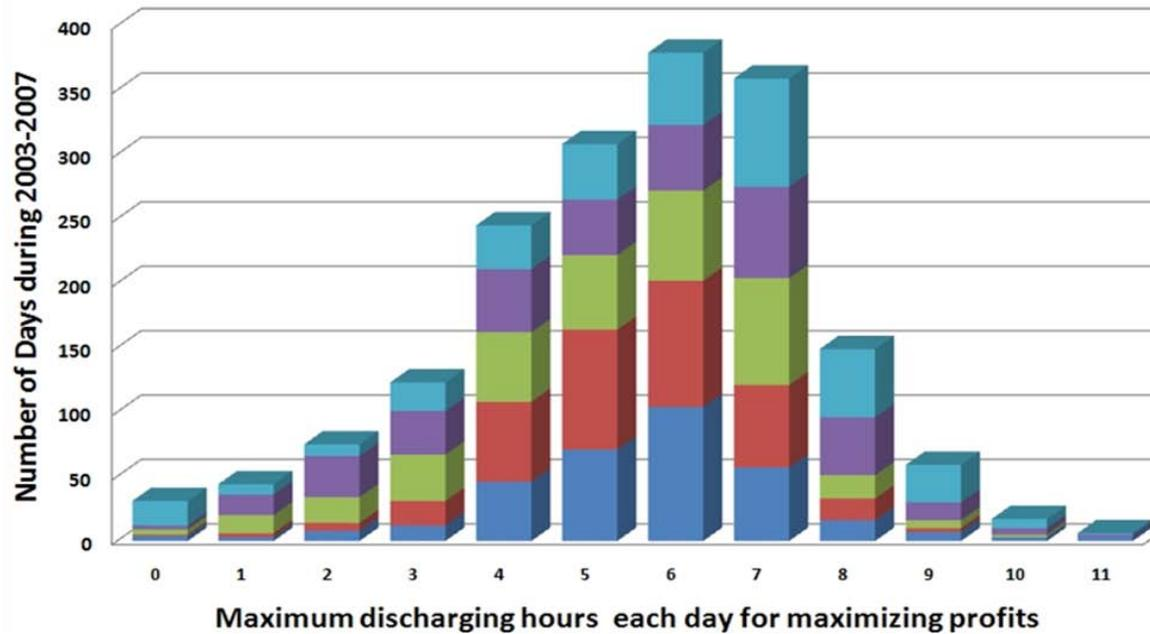
Figure 187: Anticipated operating hours for CAES unit with power ratio of 0.75 during 2003–2007
