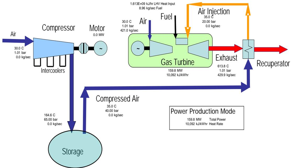
**Figure 24: Schematic and Heat and Mass Balance for the CAES AI Plant Option Without Air Injection (Based on Performance of GE7241-FA-CT)**
