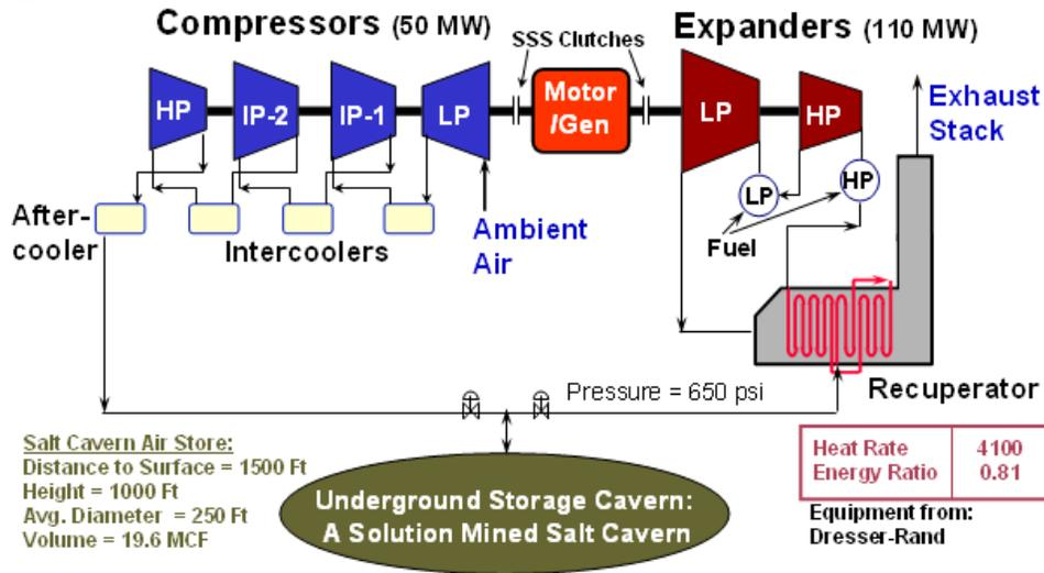
**Figure 1: Schematic of Conventional CAES Plant (e.g., the McIntosh, Alabama CAES plant, 110MW-26 Hour)**
