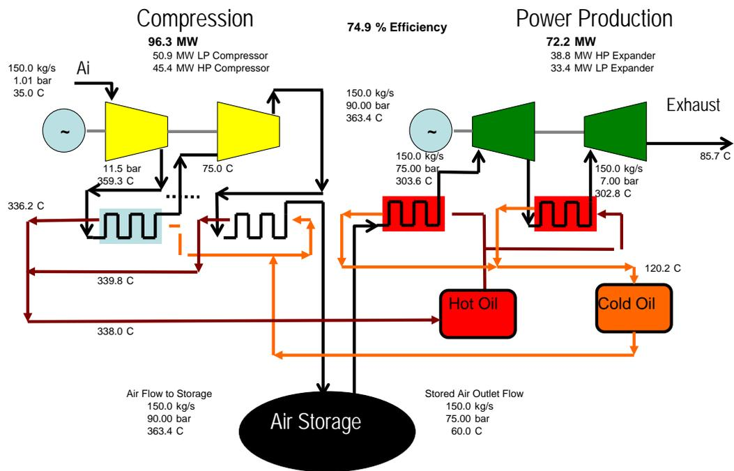
**Figure 29: Schematic and Heat and Mass Balance for the CAES Adiabatic Plant Design Option**
