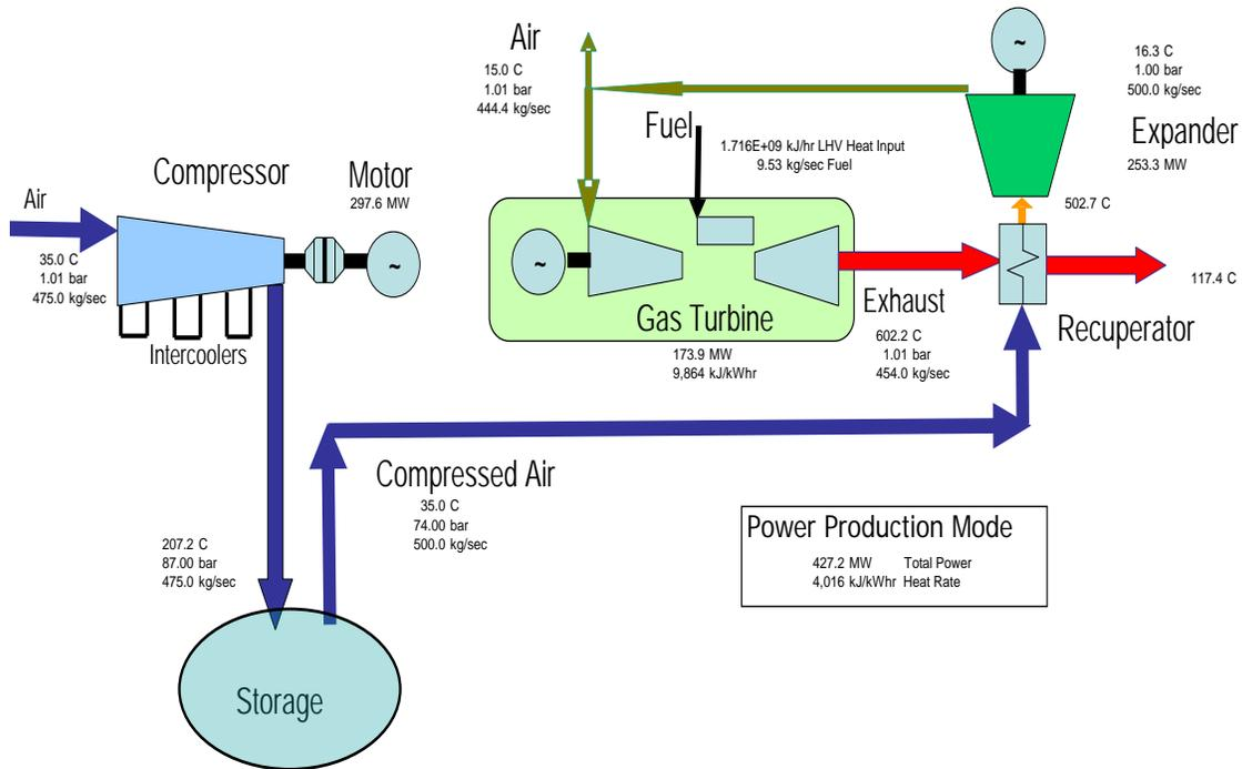
**Figure 27: Schematic and Heat and Mass Balance for the CAES/Expander/Inlet Chilling Plant Option**
