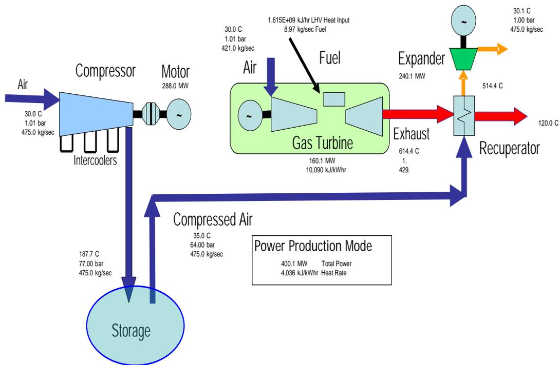
**Figure 28: Schematic and Heat and Mass Balance for the CAES/Expander Plant Option**
