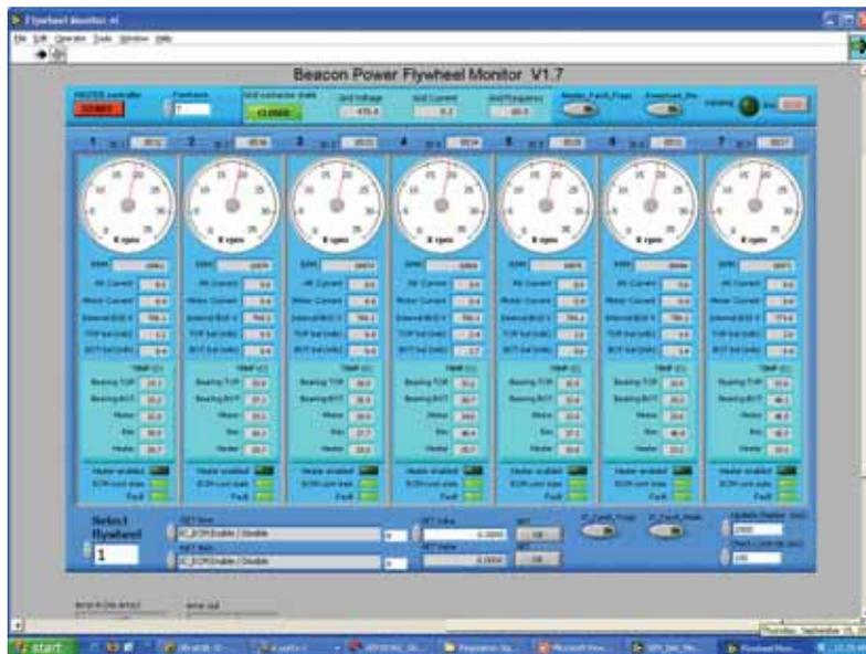
This interface provides detailed operating data about each flywheel. This will be used to monitor individual flywheel performance and adjust operating set-points.
