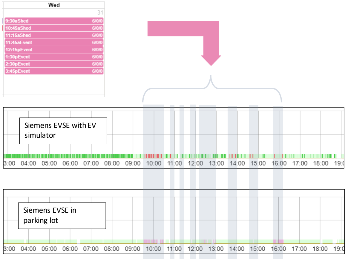
Figure 18. EVSE Responses to a Sequence of Scheduled Events
