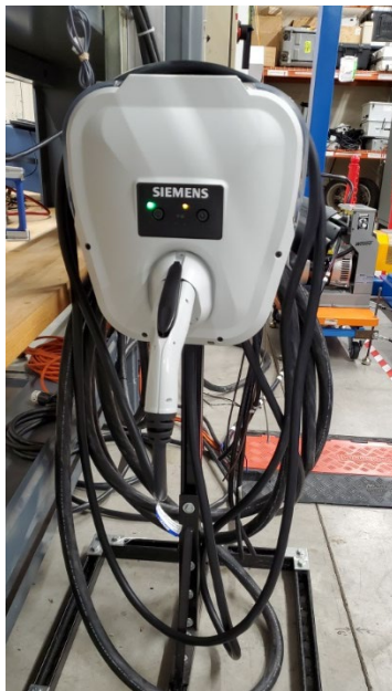
Figure 12. Electric Vehicle Supply Equipment Under Test
