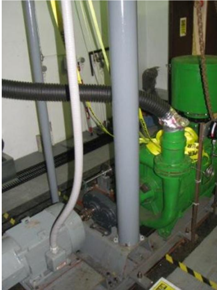
Figure 2-2. Wind turbine tower simulation tube (a length of 6 inch diameter pipe), right, was installed on test rig. The tube (later welded top and bottom) was instrumented on both ends with vibration sensors so their signals could be assessed for predicted vs. measured transmission loss and distortion. The thinner vertical tube at left was later removed from the test set-up.
