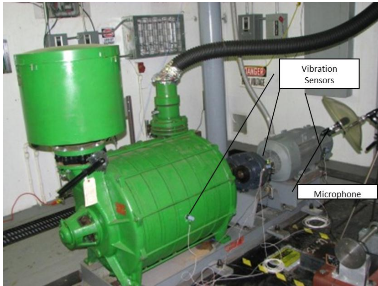
Figure 2-3. In-House test rig as finally configured. Not shown is vibration sensor at top of Tower Simulation Tube.
