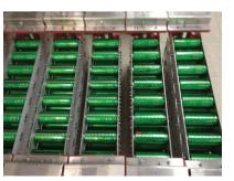
Testing is underway to use capacitors as energy storage devices on subway cars. The capacitors will absorb regenerative breaking energy and then release energy to supplement acceleration.
